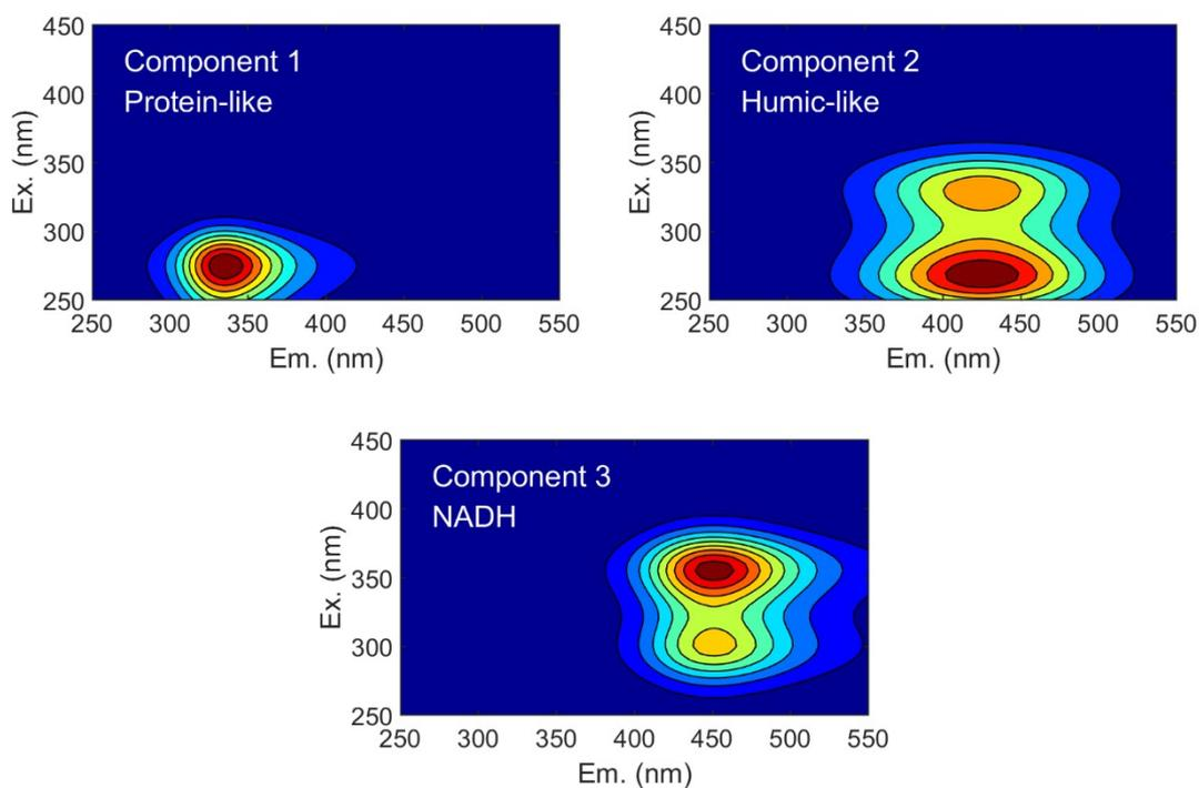
**Figure S4** PARAFAC components decomposed from EEMs acquired with Optic fiber
