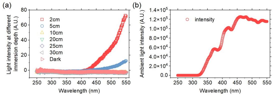
**Figure S11** Light intensity at different immersion depths in activated sludge suspension (a), and ambient light intensity (b)
