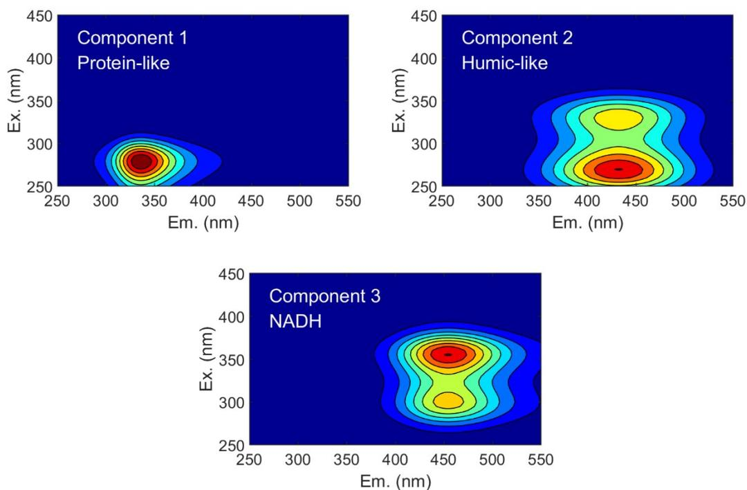
**Figure S5** PARAFAC components decomposed from EEMs acquired with conventional right-angle EEM (the SMP, EPS, and IPS samples)
