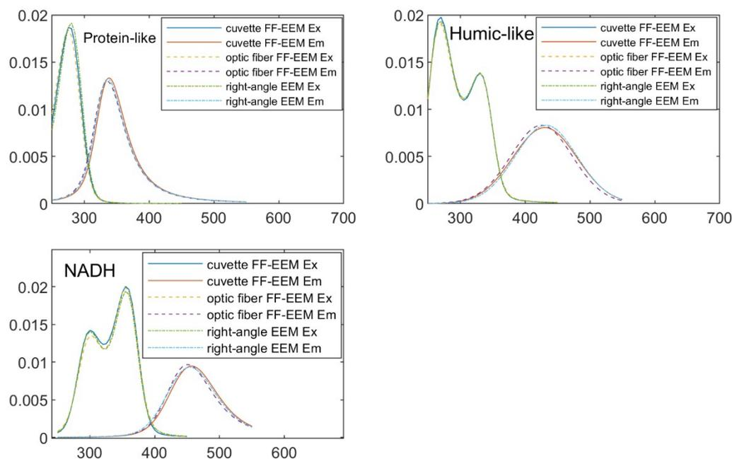
**Figure S8** Comparison of the Ex loading and Em loading of each component from different PARAFAC models.
