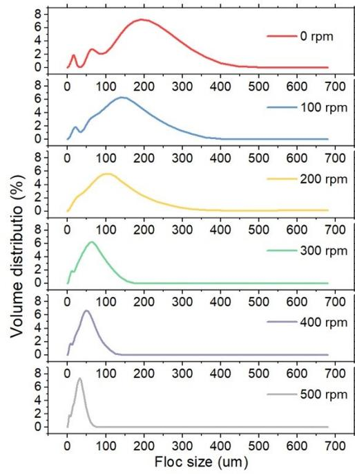
**Figure S2** Floc sizes at different stirring speeds.
