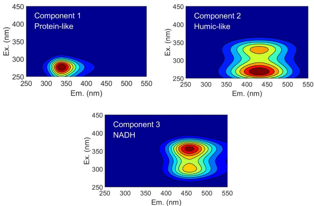
**Figure S3** PARAFAC components decomposed from EEMs acquired with cuvette
