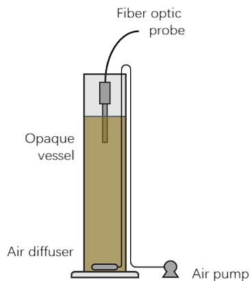
**Figure S1** Schematic diagram of fiber optic FF-EEM measurement for activated sludge suspended solid.
