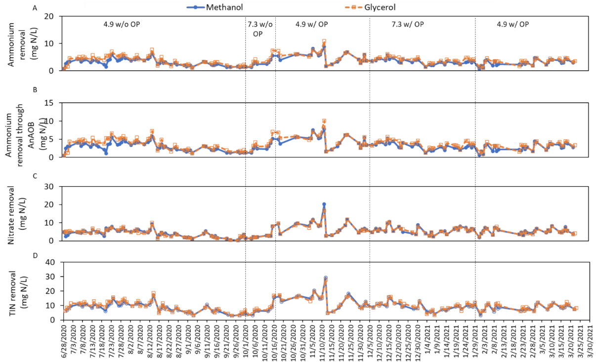
Figure S2. Methanol and glycerol filters removal at 4.9 and 7.3 m/hr with and without phosphorus addition. A. Ammonium removal, B. Ammonium removal through AnAOB, C. nitrate removal, D. TIN removal. The steady state phase discussed in the main paper is at 4.9 m/hr with phosphorus addition
