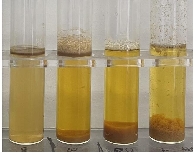
**Fig. S10.** Effect drawing of wastewater treatment in DF process (from left to right, NaClO, CaCl<sub>2</sub>, PAC and PAM are added in order)
