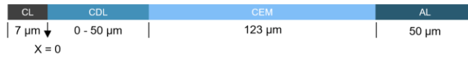
Fig. S3 Schematic of the one-dimensional model with the thickness of each component indicated. X = 0 represents where the Distance from Cathode is calculated from in all modelling figures.
