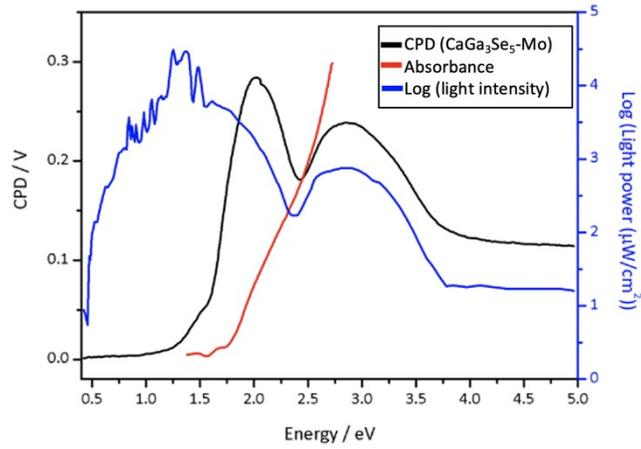
**Figure S3.** Overlay of the logarithmic irradiance with the optical absorbance and surface photovoltage spectrum of a CGSe film on Mo.
