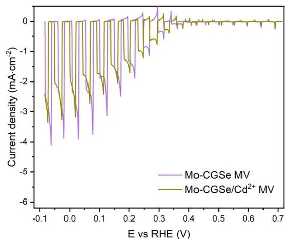
**Figure S2.** Linear sweep voltammetry (LSV) scans under chopped illumination ( $400\text{ nm}$ ,  $81\text{ mW}\cdot\text{cm}^{-2}$ ) for Mo-CGSe MV junction before and after  $\text{Cd}(\text{OAc})_2$  treatment.
