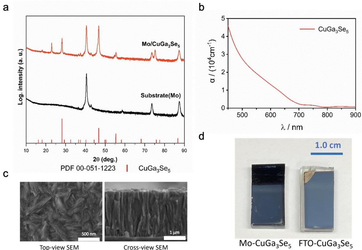
**Figure S1.** a) XRD pattern of CGSe film on Mo substrate. b) Optical absorption spectrum. c) SEM images of the Mo-CGSe electrode. d) Photograph of the two films on Mo and FTO.
