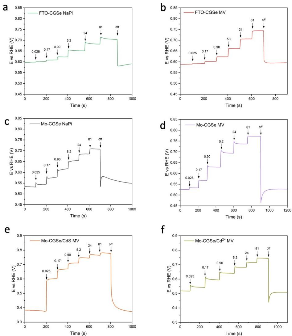
**Figure S4.** Open circuit potential (OCP) data in the dark and under 400 nm monochromatic illumination of variable intensity (irradiance given in  $\text{mW}\cdot\text{cm}^{-2}$ ). (a) FTO-CGSe/NaPi. (b) FTO-CGSe/MV. (c) Mo-CGSe/NaPi. (d) Mo-CGSe/MV. (e) Mo-CGSe/CdS/MV. (f) Mo-CGSe/Cd<sup>2+</sup>/MV. Electrolytes were de-aerated by continuous N<sub>2</sub> bubbling.
