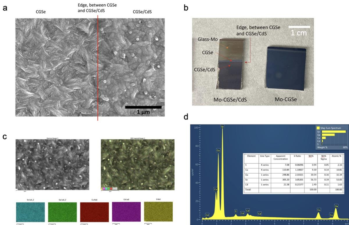
**Figure S5.** (a) Top-view SEM image of the Mo-CGSe/CdS electrode, showing the region where the left part is the CGSe surface and the right part is the CGSe/CdS surface. This corresponds to the border marked in the photograph, and is the result from masking half of the sample with scotch tape. (b) Photograph of the Mo-CGSe/CdS and the Mo-CGSe electrodes. (c)(d) EDS mapping, elemental spectrum and quantification results of the Mo-CGSe/CdS surface.
