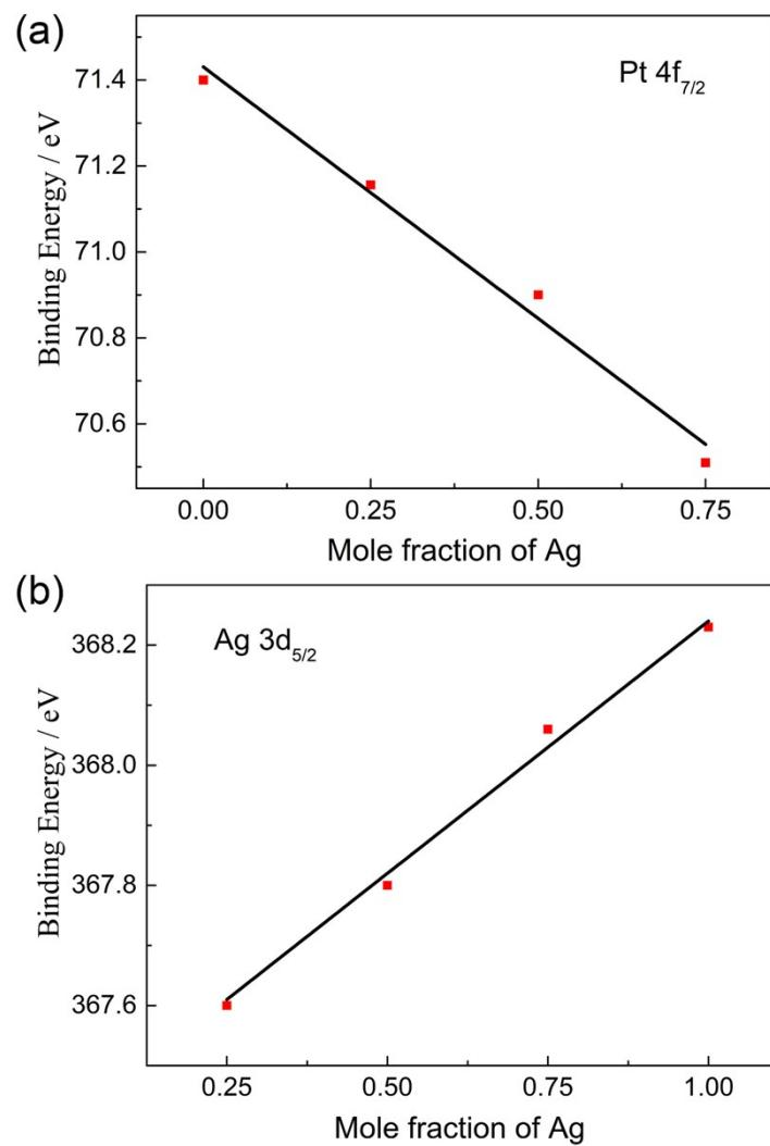
**Figure S 5(a, b)** Plot of the binding energy of Pt  $4f_{7/2}$  and Ag  $3d_{5/2}$  versus the Ag mole fraction in the precursor, respectively.
