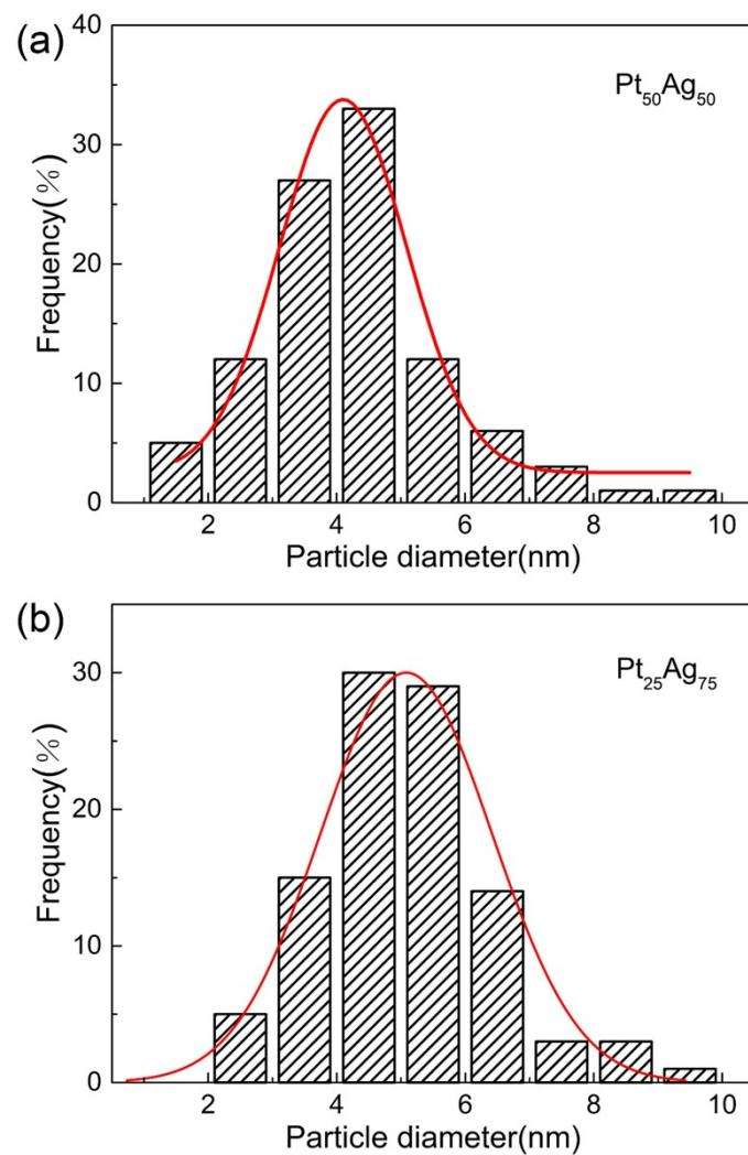
**Figure S 4** Particle size distribution of as-prepared samples corresponding to Fig-S3. (a)  $\text{Pt}_{50}\text{Ag}_{50}$  NP, (b)  $\text{Pt}_{25}\text{Ag}_{75}$  NP.
