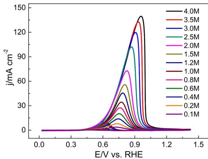
**Figure S11** Cyclic voltammetry profiles of methanol oxidation reaction(MOR) for Pt<sub>50</sub>Ag<sub>50</sub> NP 1 M KOH solution containing methanol of various concentrations at a scan rate of 50 mV s<sup>-1</sup>.
