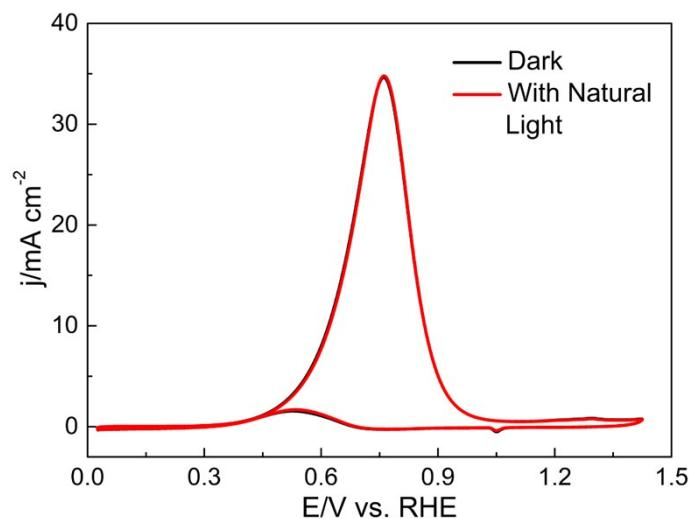
**Figure S15** Effect of the natural light on methanol oxidation reaction of Pt<sub>50</sub>Ag<sub>50</sub> NP in 1 M methanol + 1 M KOH solution at a scan rate of 50 mV s<sup>-1</sup>.
