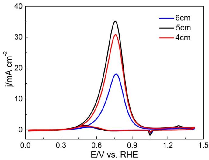
**Figure S12** Cyclic voltammetry profiles of methanol oxidation reaction (MOR) for  $\text{Pt}_{50}\text{Ag}_{50}$  NP with different substrate-target distance in 1 M methanol + 1 M KOH solution at a scan rate of  $50 \text{ mV s}^{-1}$ .
