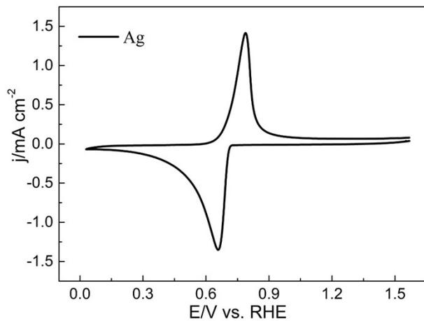
**Figure S 7** Cyclic voltammetry(CV) profiles of Ag NP in 0.1 M  $\text{HClO}_4$  solution at a scan rate of  $50 \text{ mV s}^{-1}$ .
