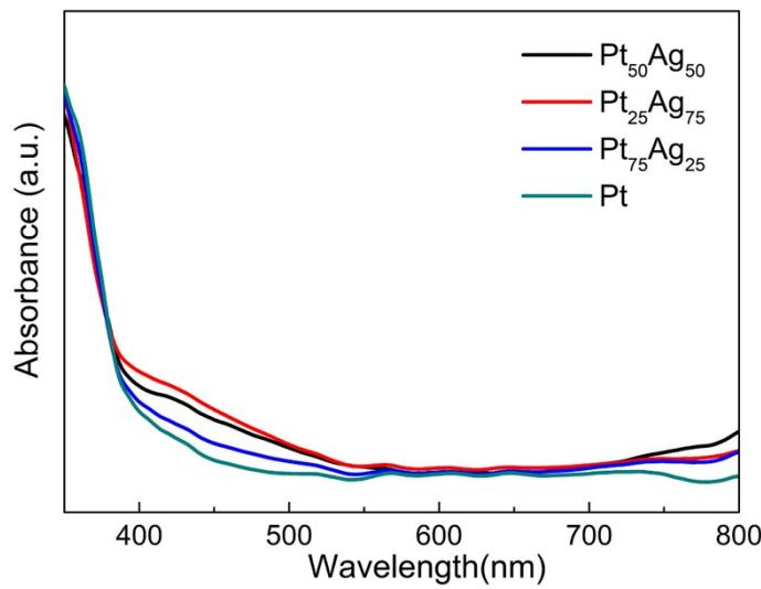
**Figure S14** Diffuse reflectance UV-vis absorption spectroscopy of Pt, Pt<sub>75</sub>Ag<sub>25</sub>, Pt<sub>50</sub>Ag<sub>50</sub> and Pt<sub>25</sub>Ag<sub>75</sub> NP.
