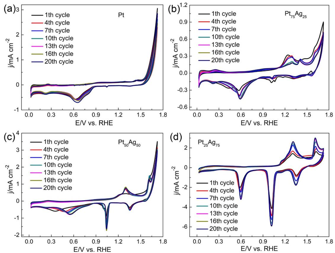
**Figure S10** Cyclic voltammetry profiles of as-prepared samples in 1 M KOH solution at a scan rate of 50 mV s<sup>-1</sup>. (a) Pt NP, (b) Pt<sub>75</sub>Ag<sub>25</sub> NP. (c) Pt<sub>50</sub>Ag<sub>50</sub> NP, (d) Pt<sub>25</sub>Ag<sub>75</sub> NP.
