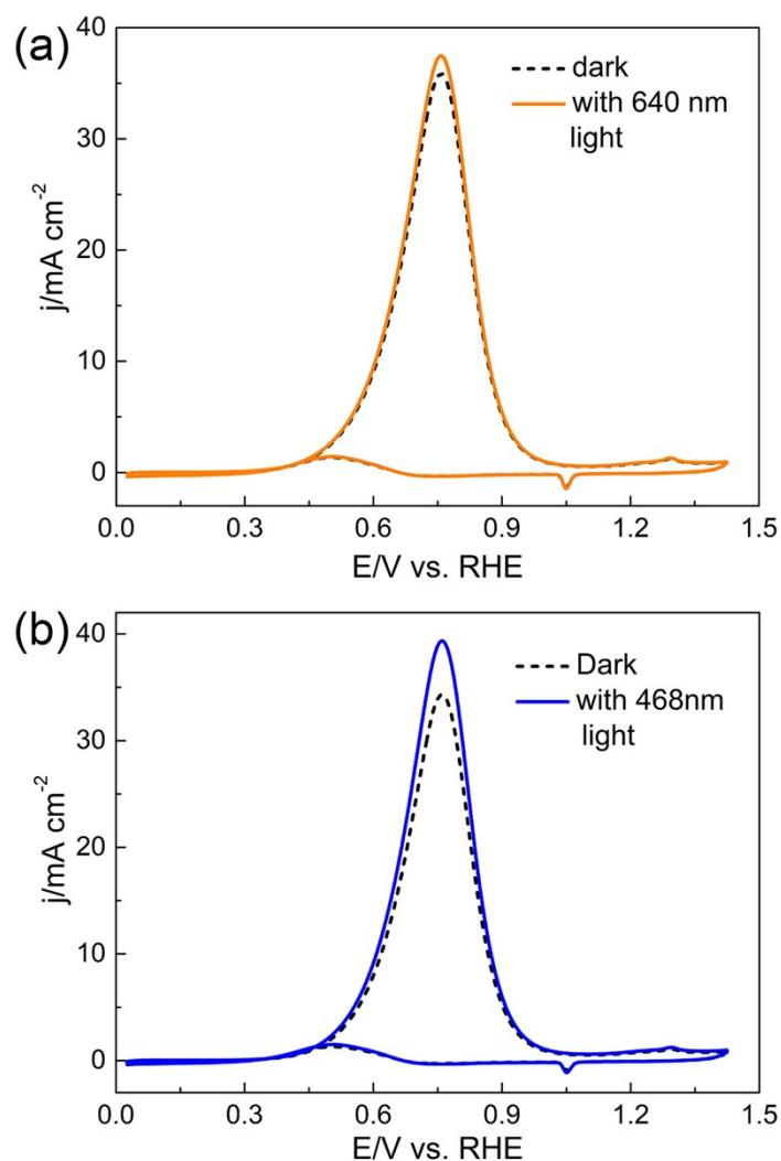
**Figure S16** Effect of the UV light of 640 nm and 468 nm on methanol oxidation reaction of  $\text{Pt}_{50}\text{Ag}_{50}$  NP in 1 M methanol + 1 M KOH solution at a scan rate of  $50 \text{ mV s}^{-1}$ .
