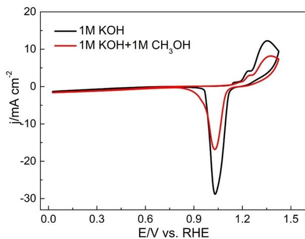
**Figure S 9** Cyclic voltammetry (CV) profiles of Ag NP in 1 M KOH solution (black) and in 1 M methanol + 1 M KOH solution (red) at a scan rate of  $50 \text{ mV s}^{-1}$ .
