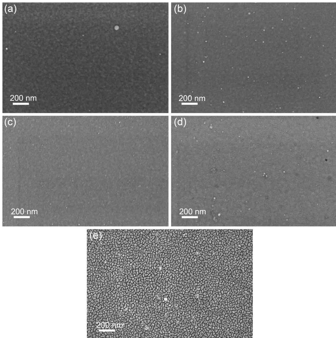
**Figure S1.** Morphology characterization of as-prepared samples. SEM images of Pt NP (a), Pt<sub>75</sub>Ag<sub>25</sub> NP (b), Pt<sub>50</sub>Ag<sub>50</sub> NP (c), Pt<sub>25</sub>Ag<sub>75</sub> NP (d), and Ag NP (e).
