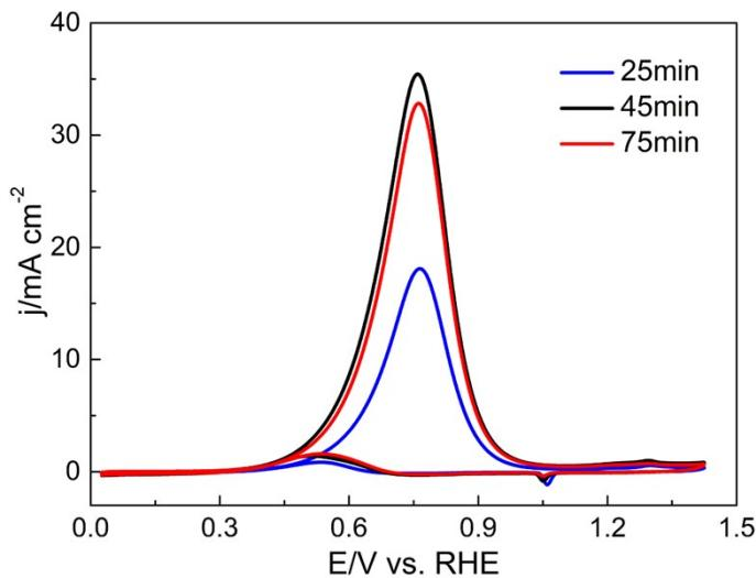
**Figure S13** Cyclic voltammetry profiles of methanol oxidation reaction (MOR) for  $\text{Pt}_{50}\text{Ag}_{50}$  NP with different deposition time in 1 M methanol + 1 M KOH solution at a scan rate of  $50\text{mV s}^{-1}$ .
