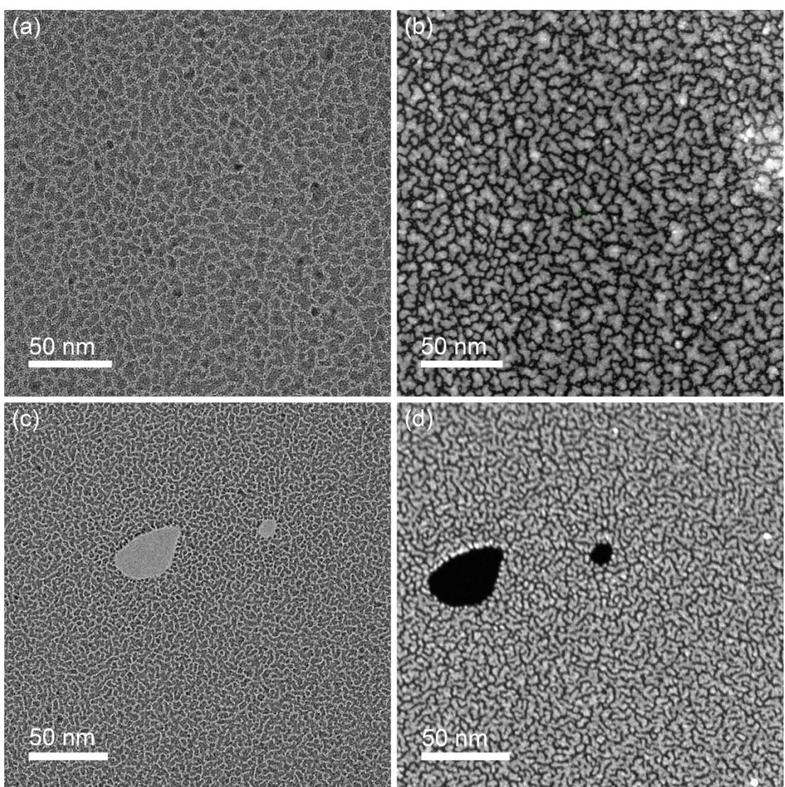
**Figure S 3** (a) STEM images of  $\text{Pt}_{50}\text{Ag}_{50}$  NP. (b) HAADF-STEM image of  $\text{Pt}_{50}\text{Ag}_{50}$  NP. (c) STEM images of  $\text{Pt}_{25}\text{Ag}_{75}$  NP. (d) HAADF-STEM image of  $\text{Pt}_{25}\text{Ag}_{75}$  NP.
