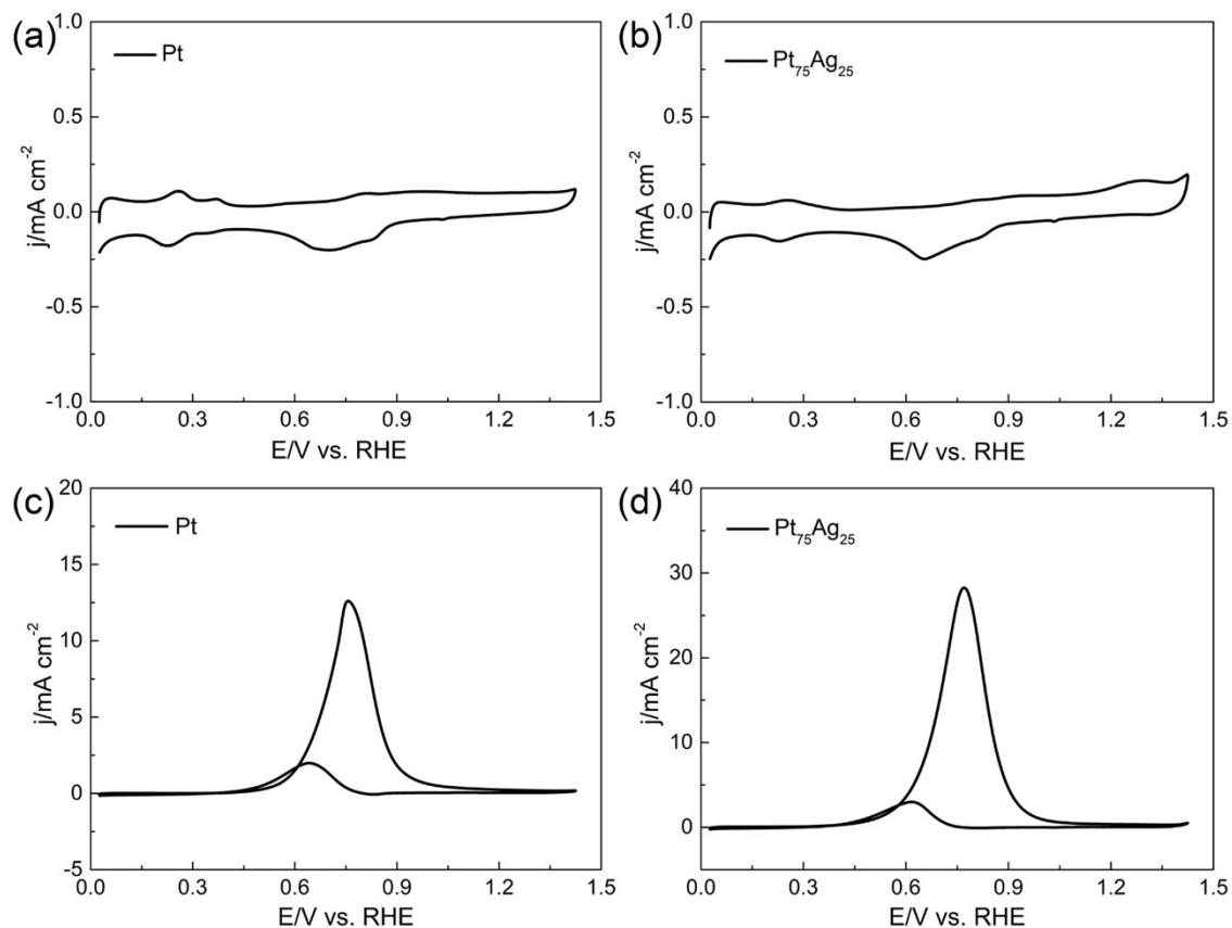
**Figure S 8(a, b)** Cyclic voltammetry profiles of Pt and  $\text{Pt}_{75}\text{Ag}_{25}$  nanoparticles in 1 M KOH solution. (c, d) Cyclic voltammetry profiles during methanol oxidation reaction for Pt and  $\text{Pt}_{75}\text{Ag}_{25}$  nanoparticles in 1 M methanol and 1 M KOH solution. All graphs are at a scan rate of  $50 \text{ mV s}^{-1}$ .
