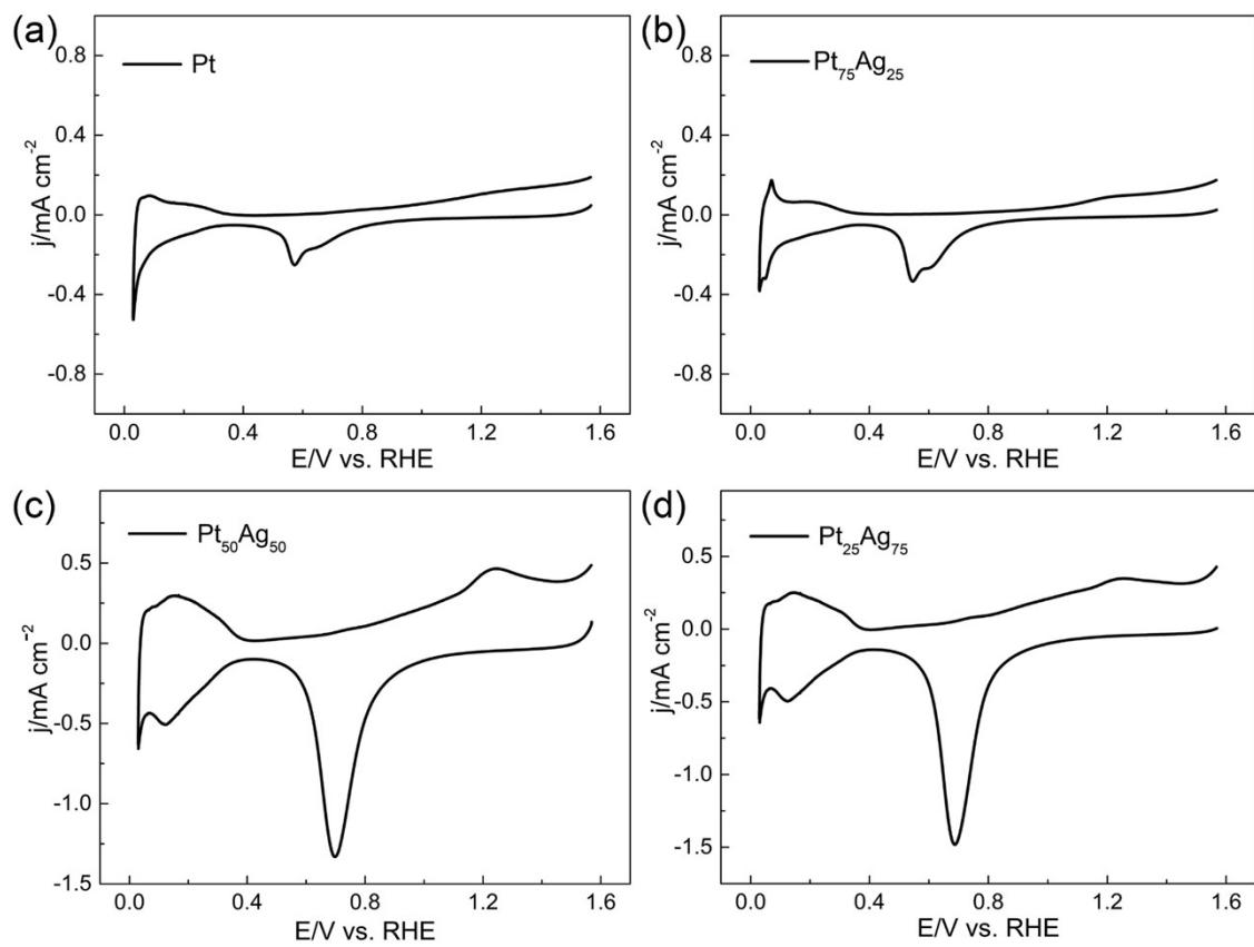
**Figure S 6** Cyclic voltammetry (CV) profiles of as-prepared samples in 0.1 M  $\text{HClO}_4$  solution at a scan rate of  $50 \text{ mV s}^{-1}$ . (a) Pt NP s, (b)  $\text{Pt}_{75}\text{Ag}_{25}$  NP. (c)  $\text{Pt}_{50}\text{Ag}_{50}$  NP, (d)  $\text{Pt}_{25}\text{Ag}_{75}$  NP.
