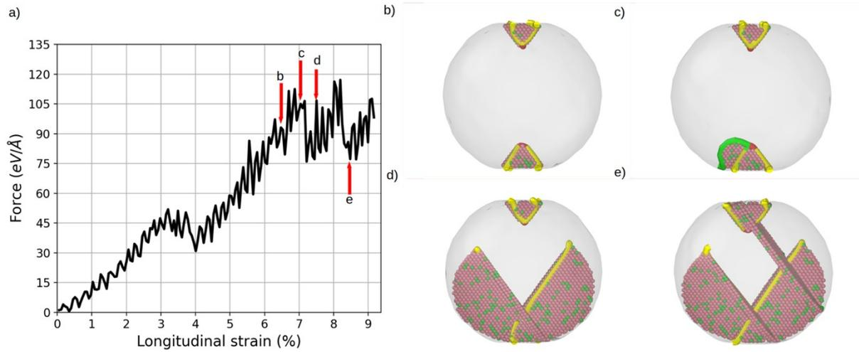
**Figure S8** (a) Dislocation density and force-strain curve of random mix  $\text{Co}_{87.5}\text{Ni}_{12.5}$ . Snapshots at: (b) 6.5%, (c) 7.0%, (d) 7.5%, and (e) 8.5% of longitudinal strain. Shockley partial, Hirth, and Other dislocation are represented by a green, yellow, and red lines, respectively; Co hcp atoms are represented by pink spheres, whereas Ni hcp atoms are represented by green spheres, while fcc atoms are omitted for clarity.
