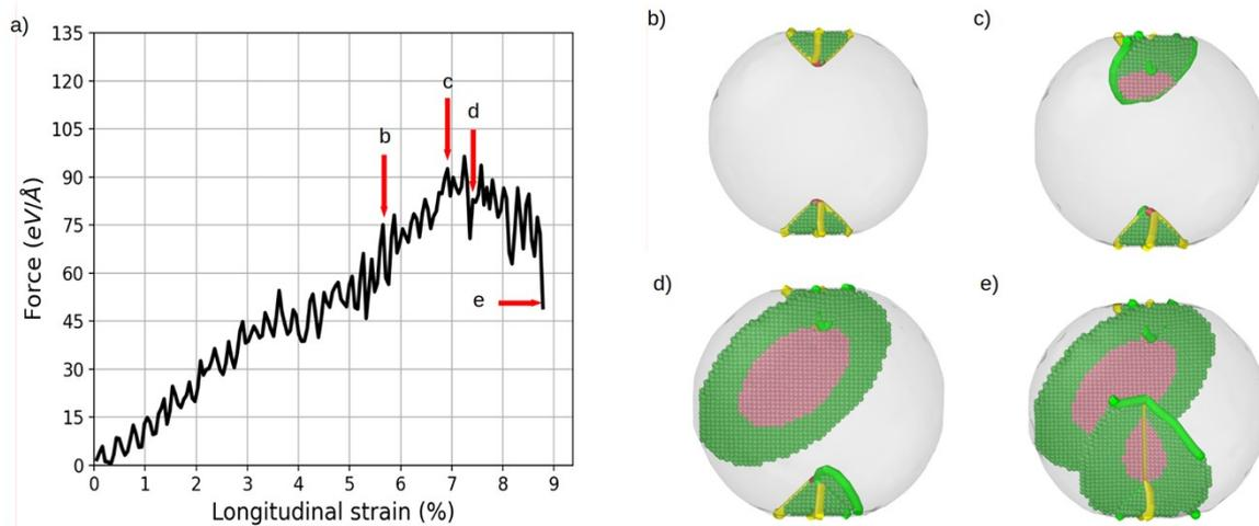
**Figure S4** (a) Dislocation density and force-strain curve of core-shell  $\text{Co}_{25}\text{Ni}_{75}$  Snapshots taken at: (b) 5.6%, (c) 6.92%, (d) 7.41%, and (e) 8.81% of longitudinal strain. Shockley partial, Hirth, and Other dislocation are represented by a green, yellow, and red lines, respectively; Co hcp atoms are represented by pink spheres, whereas Ni hcp atoms are represented by green spheres, while fcc atoms are omitted for clarity.
