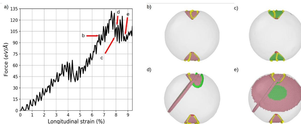
**Figure S1.** (a) Dislocation density and force-strain curve of core-shell Ni<sub>12.5</sub>Co<sub>87.5</sub> Snapshots taken at: (b) 6.65%, (c) 7.92%, (d) 8.1%, and (e) 8.71% of longitudinal strain. Shockley partial, Hirth, and Other dislocation are represented by a green, yellow, and red lines, respectively; Co hcp atoms are represented by pink spheres, whereas Ni hcp atoms are represented by green spheres, while fcc atoms are omitted for clarity.
