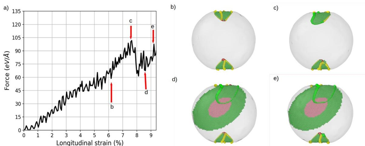
**Figure S3.** (a) Dislocation density and force-strain curve of core-shell  $\text{Co}_{12.5}\text{Ni}_{87.5}$  Snapshots taken at: (b) 6.18%, (c) 7.63%, (d) 8.54%, and (e) 9.14% of longitudinal strain. Shockley partial, Hirth, and Other dislocation are represented by a green, yellow, and red lines, respectively; Co hcp atoms are represented by pink spheres, whereas Ni hcp atoms are represented by green spheres, while fcc atoms are omitted for clarity.
