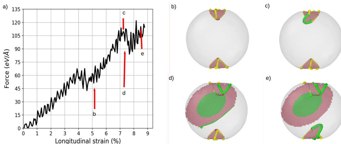
**Figure S2.** (a) Dislocation density and force-strain curve of core-shell  $\text{Ni}_{25}\text{Co}_{75}$  Snapshots taken at: (b) 5.53%, (c) 7.45%, (d) 7.62%, and (e) 8.66% of longitudinal strain. Shockley partial, Hirth, and Other dislocation are represented by a green, yellow, and red lines, respectively; Co hcp atoms are represented by pink spheres, whereas Ni hcp atoms are represented by green spheres, while fcc atoms are omitted for clarity.
