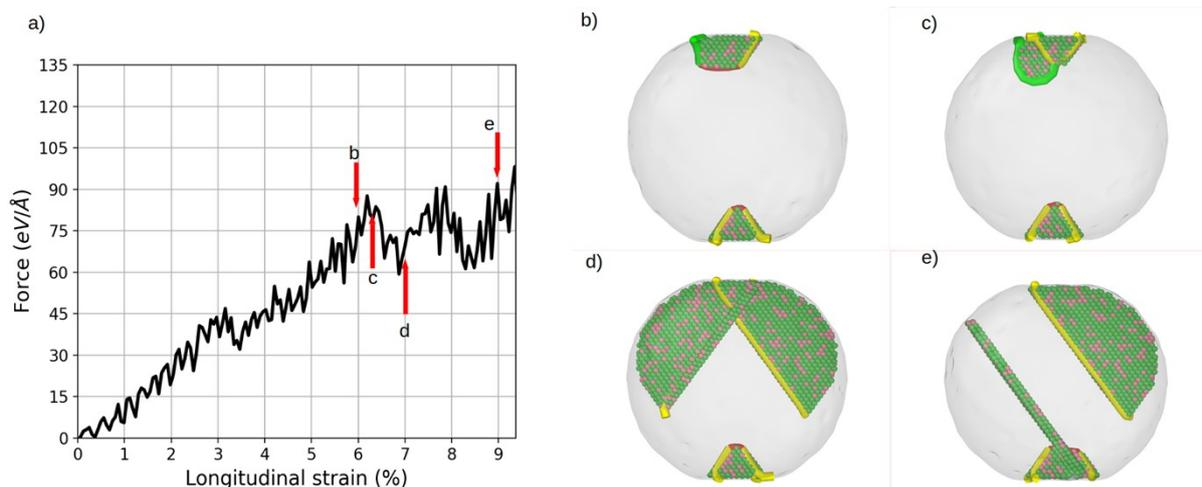
**Figure S6** (a) Dislocation density and force-strain curve of random mix  $\text{Co}_{25}\text{Ni}_{75}$ . Snapshots at: (b) 6.0%, (c) 6.3%, (d) 7.0%, and (e) 9.0% of longitudinal strain. Shockley partial, Hirth, and Other dislocation are represented by a green, yellow, and red lines, respectively; Co hcp atoms are represented by pink spheres, whereas Ni hcp atoms are represented by green spheres, while fcc atoms are omitted for clarity.
