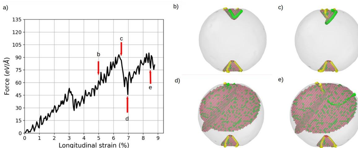
**Figure S7** (a) Dislocation density and force-strain curve of random mix  $\text{Co}_{75}\text{Ni}_{25}$ . Snapshots at: (b) 5.0%, (c) 6.41%, (d) 7.0%, and (e) 8.5% of longitudinal strain. Shockley partial, Hirth, and Other dislocation are represented by a green, yellow, and red lines, respectively; Co hcp atoms are represented by pink spheres, whereas Ni hcp atoms are represented by green spheres, while fcc atoms are omitted for clarity.
