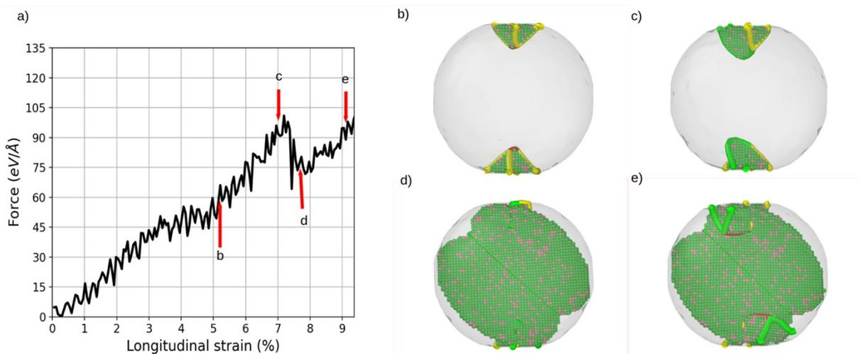
**Figure S5** (a) Dislocation density and force-strain curve of random mix  $\text{Co}_{12.5}\text{Ni}_{87.5}$ . Snapshots at: (b) 5.15%, (c) 7.01%, (d) 7.67%, and (e) 9.16% of longitudinal strain. Shockley partial, Hirth, and Other dislocation are represented by a green, yellow, and red lines, respectively; Co hcp atoms are represented by pink spheres, whereas Ni hcp atoms are represented by green spheres, while fcc atoms are omitted for clarity.
