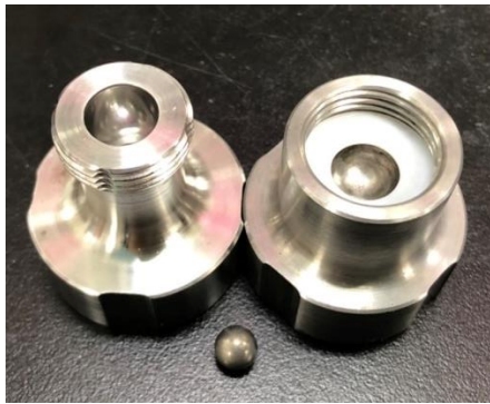
Figure S2. Stainless jar and ball used in this study.
