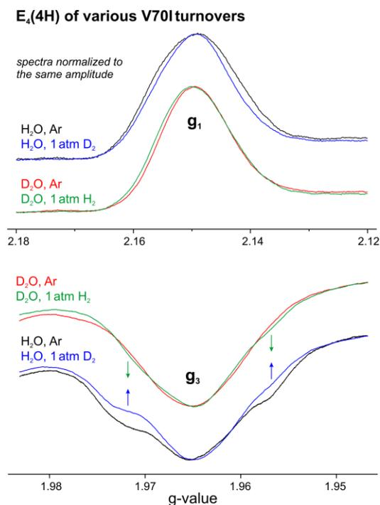
**Figure S1.** Expanded  $g_1$  and  $g_3$  portions of X-band EPR spectra of the  $E_4(4H)$  level intermediates showing effect of  $\alpha$ -V70I turnover conditions ( $H_2O$  vs  $D_2O$ ; Ar vs  $D_2$  and  $H_2$  atmosphere) on signal linewidth of trapped  $E_4$  state. **EPR conditions:** temperature, 12 K; microwave frequency,  $\sim 9.36$  GHz; microwave power, 10 mW; modulation amplitude, 3 G; time constant, 160 ms; field sweep speed, 5 G/s.
