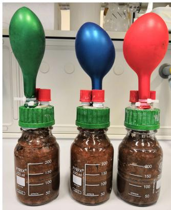
**Figure S 4:** experimental setup used for working at low pressure conditions
