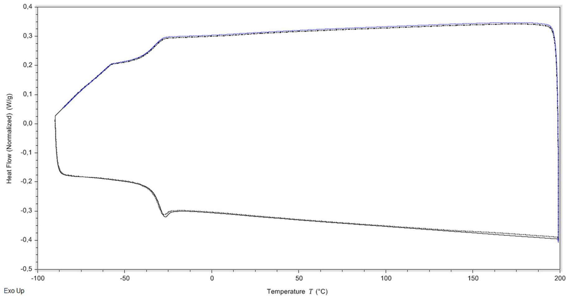
Figure S 25: Differential scanning calorimetry analysis of the purified polymer. Two cycles at 10K min<sup>-1</sup>.
