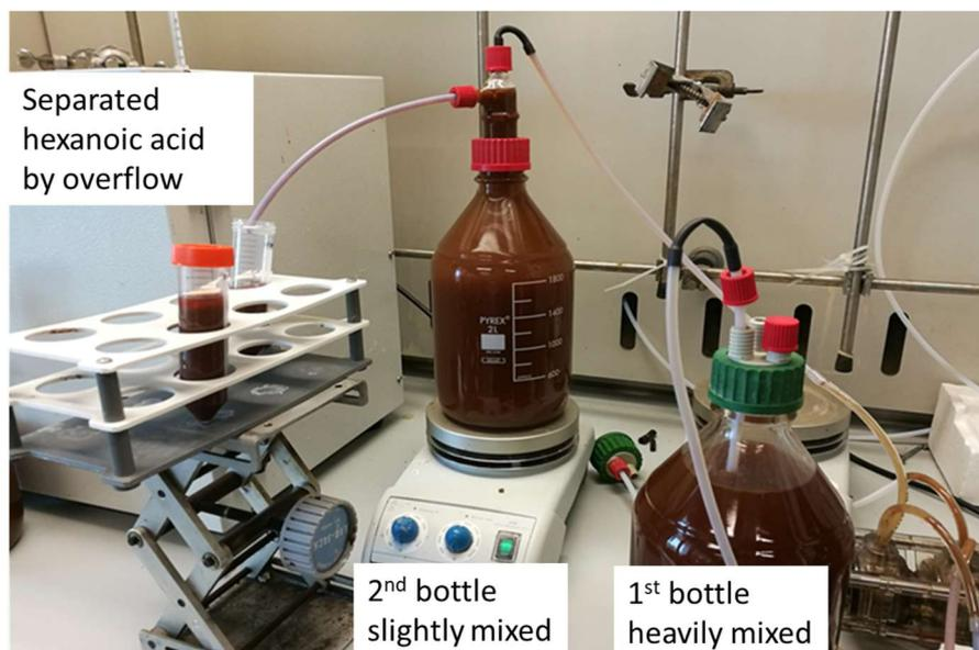
**Figure S 7:** Experimental set-up for separating the insolubilized hexanoic acid.
