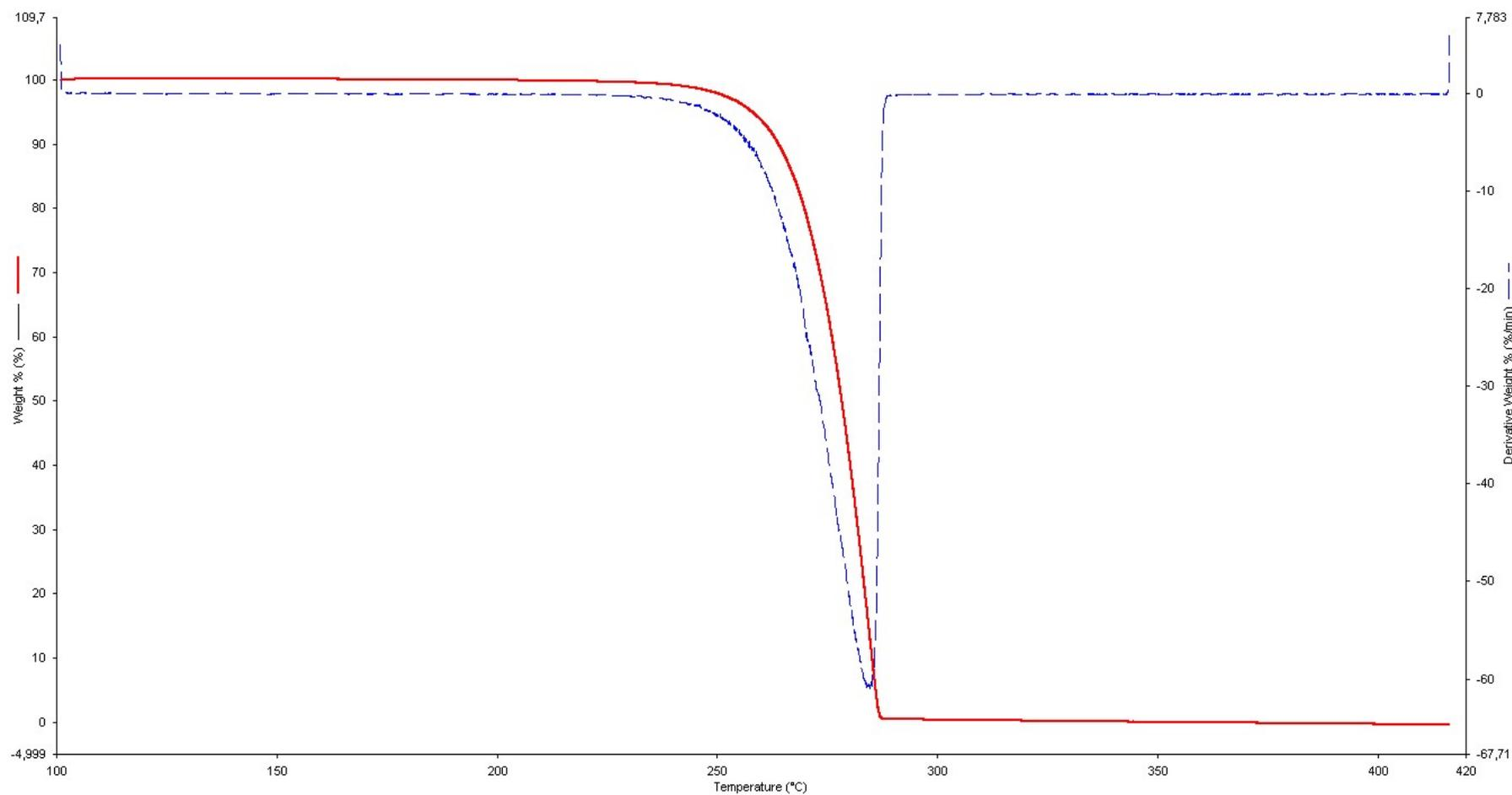
**Figure S 26:** thermogravimetric analysis of the purified polymer, with a degradation temperature of 287 °C.
