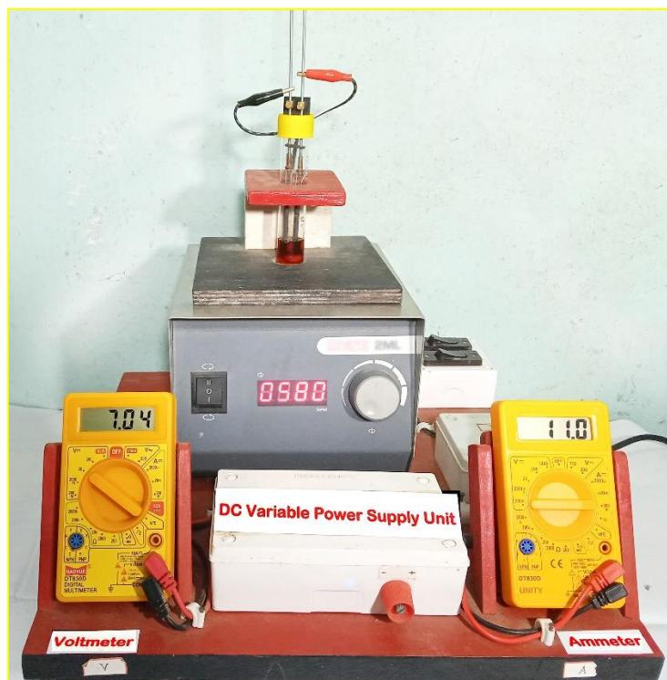
**Figure S1a:** Pictorial view (Front-View) of the experimental set-up for the model reaction showing the designed ‘DC Variable Power Supply’ unit tagged with Voltmeter and Ammeter, and an undivided electrochemical cell containing a pair of graphite plates (cathode and anode) and the reaction mixture within a glass vessel placed on a magnetic stirrer with constant stirring at ambient conditions.
