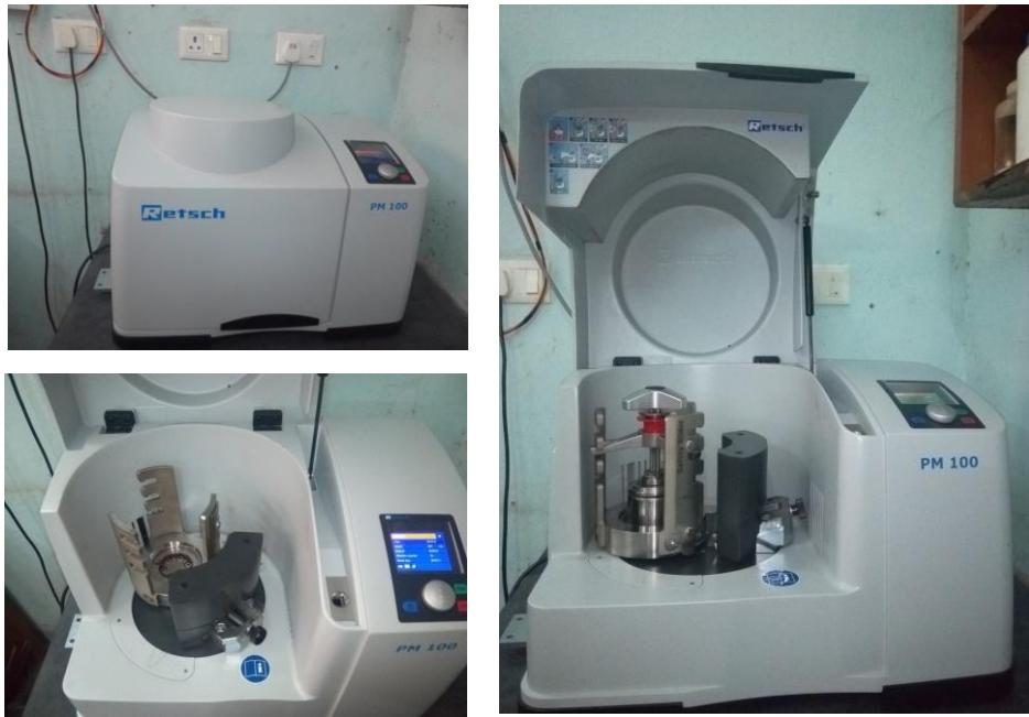
**Figure S1b:** Pictorial view PM 100, Retsch GmbH, Germany, ball-milling apparatus
