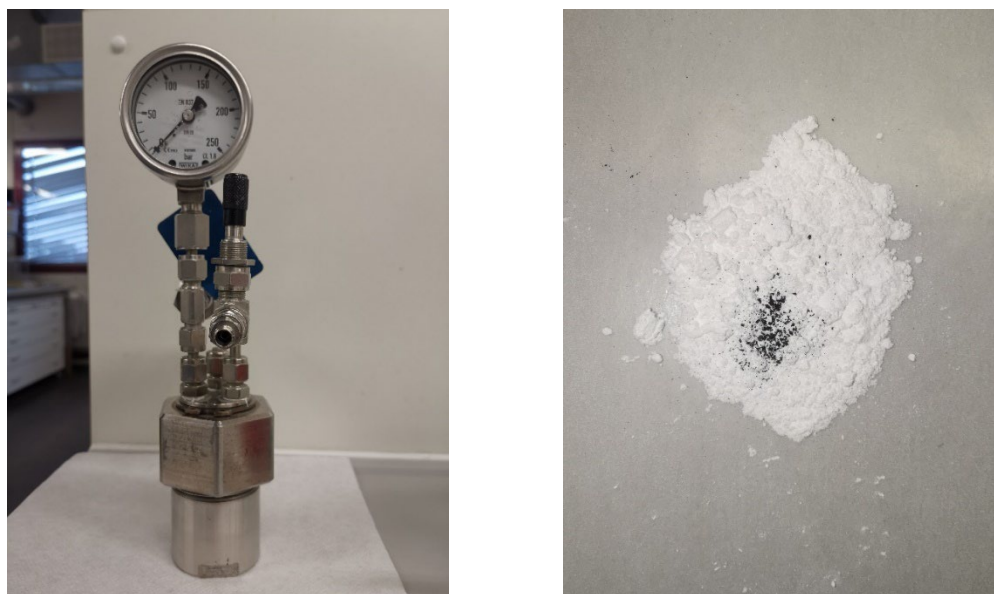
Figure E1. Left) One of the used 50 ml autoclaves. Right) Experimental approach with 138 mg PHB and 5 mg Ru/CeO 2 .
