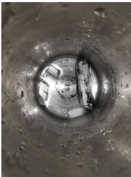
Figure S19. Picture taken after the PHB, PLA and PET recycling approach. Reaction solution has been deducted. The remaining polymer fragments (After reaction 97.6 mg – initially 101.9 mg) are made of PET.
