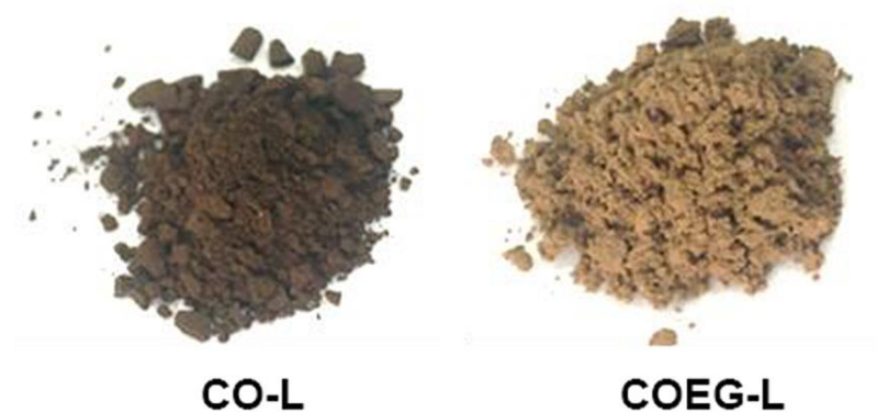
Fig. S5 Digital images of the isolated CO-L and COEG-L. the dark color of CO-L revealed a severe condensation of lignin as previously described while COEG-L showed a light brown color, demonstrating that the lignin was less condensed due to the tailoring effect of EG.
