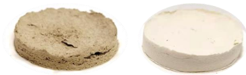
Fig. S7 Digital images of COPA-SR (left) and COPD-SR (right). The SR from COPA fractionation system showed a darker color than the COPD system, revealing that the hydroxy rich PD molecules can promote delignification, possibly due to the hydrogen bond formation between alkoxyated lignin and DES.
