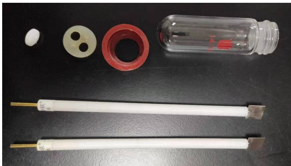
Figure S1. The materials used to make the electrolytic cell for the synthesis of \beta -amino nitriles.
