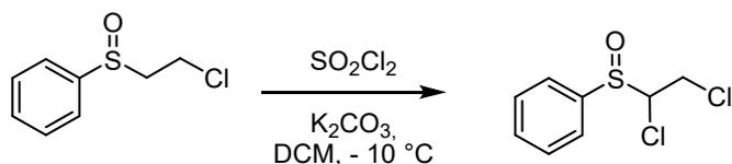
Figure S14. Synthetic scheme for the preparation of ((1,2-dichloroethyl)sulfinyl)benzene (CEPSOCl)
