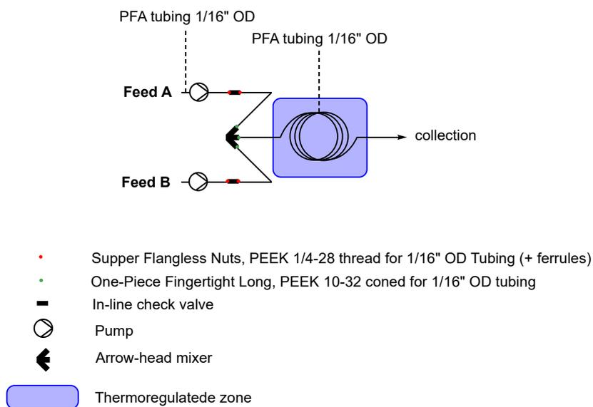
Figure S2. Detailed setup for the continuous flow oxidation of thioethers.
