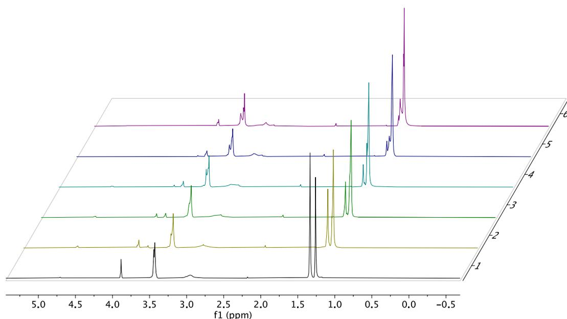
Figure S4. Stacked <sup>1</sup>H NMR spectra showing the hypochlorite exchange between **tBuOCl** and **MeOCl**. Spectrum 1 was recorded within a few seconds of addition of **tBuOCl**. Subsequent spectra were recorded at intervals of 10 min.
