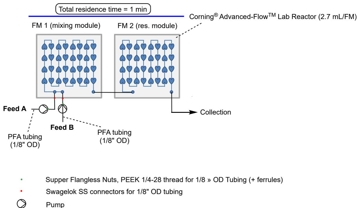
Figure S3. Detailed continuous flow setup for the neutralization of CWA simulants (Lab scale).
