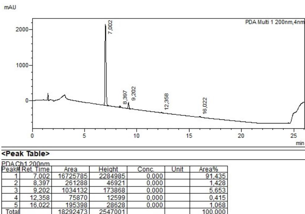
Figure S5. HPLC chromatogram of the oxidation of **1a** under the optimized conditions. (Flow rate: 1.2 mL min<sup>-1</sup>; Residence time: 60 s; Feed solutions: thioanisole (**1a**) 0.5 M in MeOH, and *t*BuOCl 0.55 M in MTBE.)
