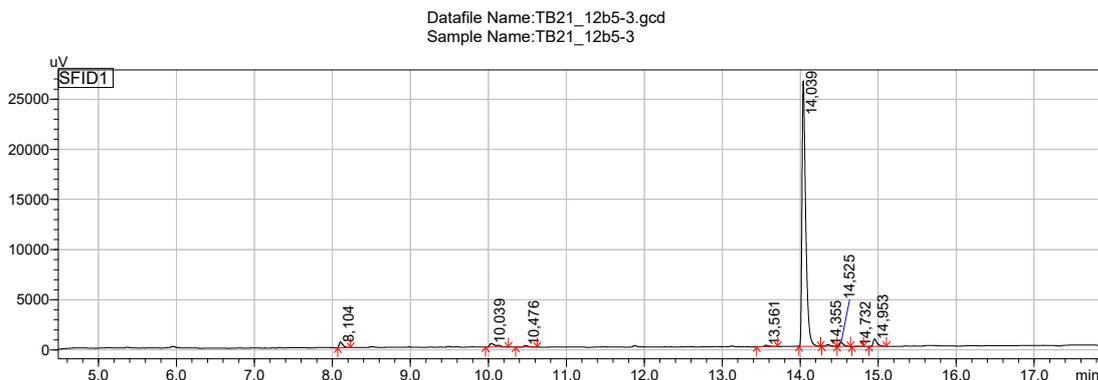
Figure S8. GC-FID chromatogram of the oxidation of **CEES** under optimized conditions (Flow rate: 1.2 mL min<sup>-1</sup>; Residence time: 60 s; Feed solutions: **CEES** 0.5 M in MeOH, and tBuOCl 0.6 M in MTBE.)
