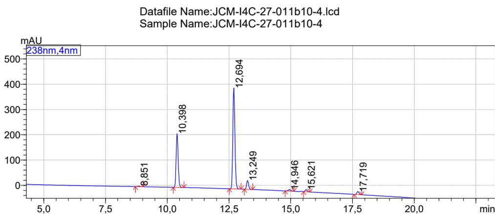
Figure S9. HPLC chromatogram of the oxidation of **CEPS** according the following conditions: Flow rate: 1.2 mL min<sup>-1</sup>; Residence time: 60 sec; Feed solutions: **CEPS** 0.5 M in MeOH, and *t*BuOCl 1 M in MTBE.
