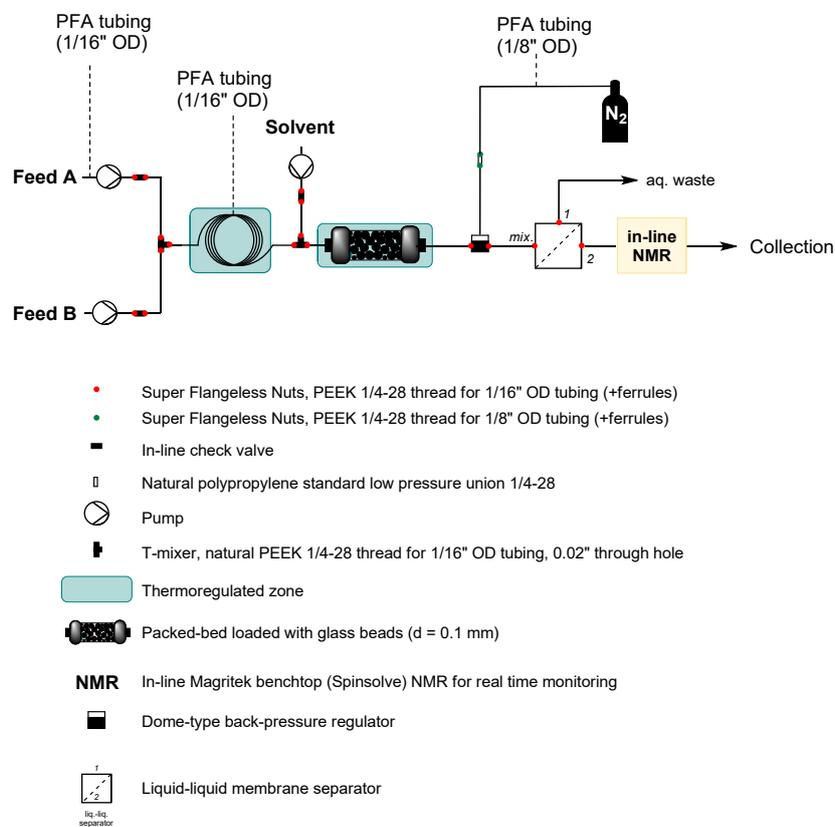
Figure S1. Detailed setup for the continuous flow preparation of organic hypochlorites.
