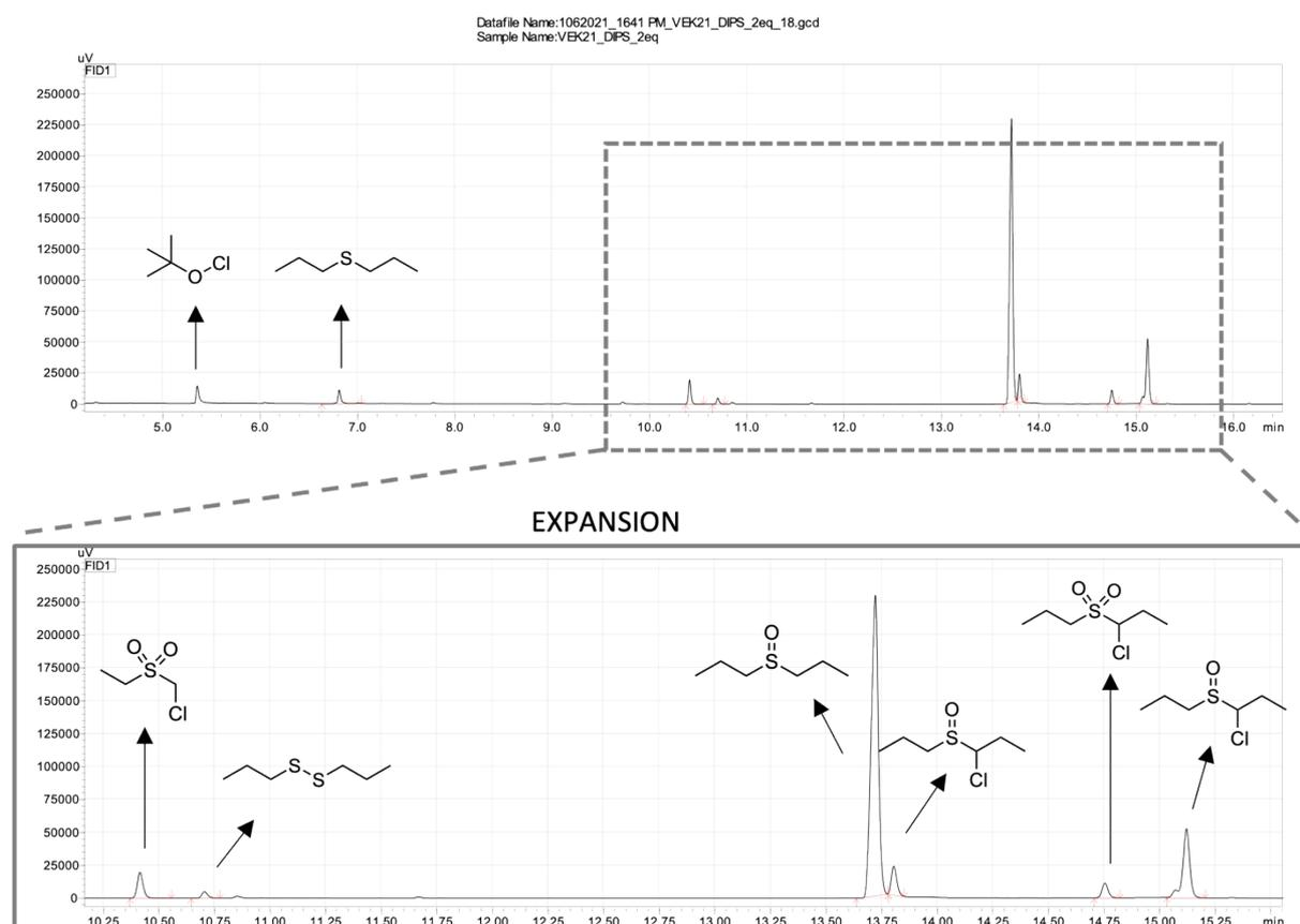
Figure S11. Identification of all the major peaks obtained in oxidation procedures for **1d**.
