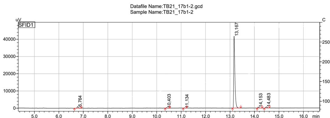
Figure S7. GC-FID chromatogram for the oxidation of **1d** under optimized conditions. (Flow rate: 1.2 mL min<sup>-1</sup>; Residence time: 60 s; Feed solutions: dipropylsulfide (**1d**) 0.5 M in MeOH, and *t*BuOCl 0.55 M in MTBE.)
