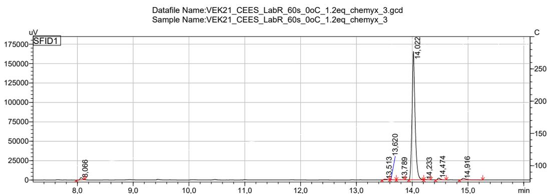
Figure S10. GC-FID chromatogram for the oxidation of **CEES** in mesofluidic scale (Lab Reactor) For exact reaction conditions, see the paragraph on procedure above.
