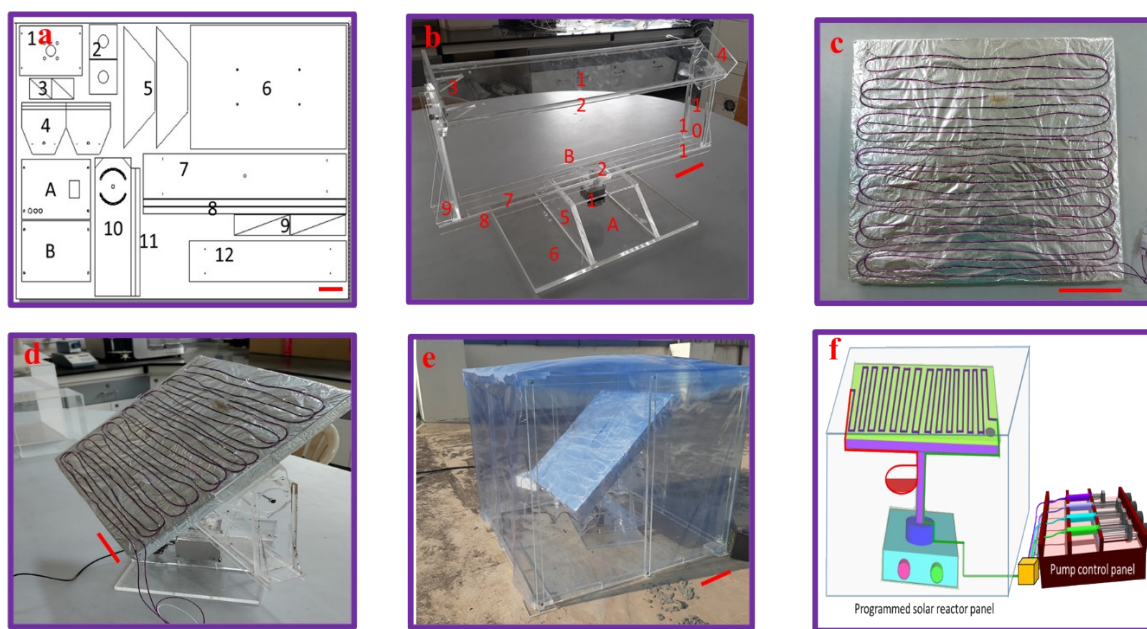
Figure S7. (a) Laser cutting design of solar panel; (b) acrylic body chassis of solar panel; (c) PFA tubing solar reactor; (d) pasting of solar reactor on acrylic body chassis of solar panel; (e) Solar panel under blue light film; (f) schematic diagram of photo reaction set-up, bar represent the 10 cm.
