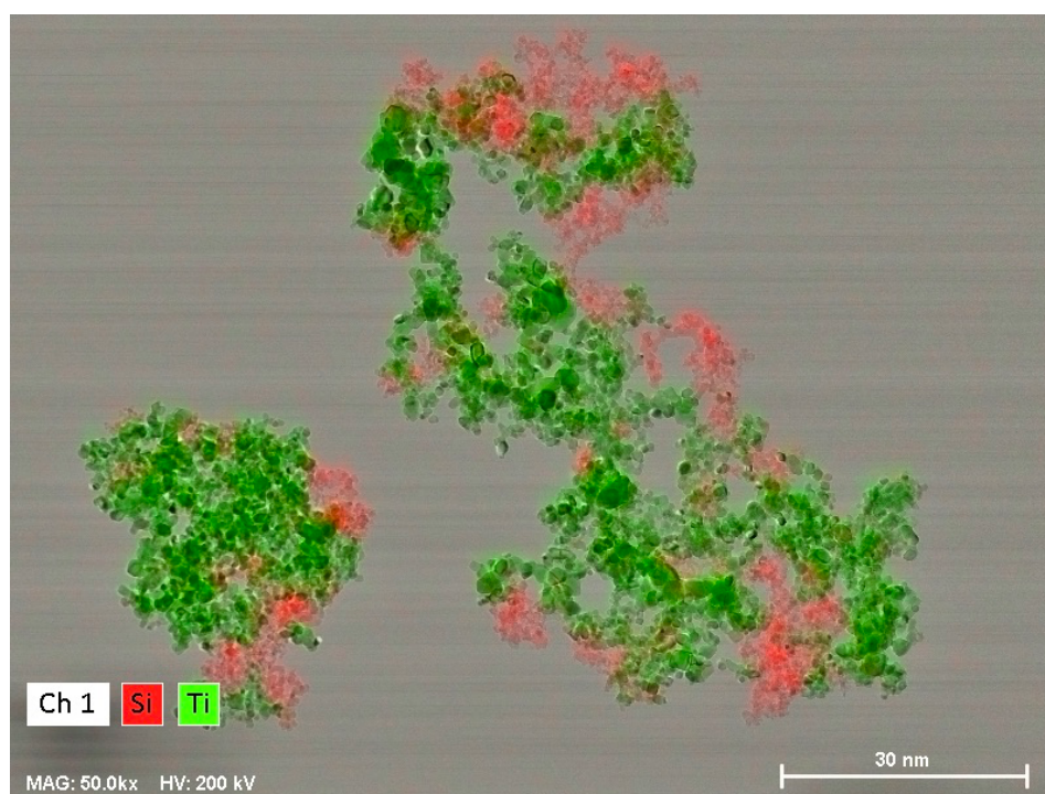
Fig. S14 TEM EDX mapping of image of sitinakite reaction mixture after ball milling (30 minutes 400 rpm), same sample as in Fig. S13.
