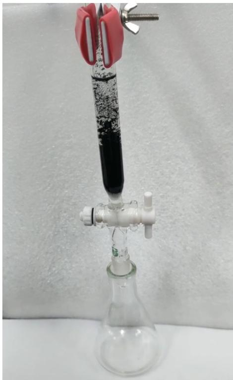
**Fig. S2.** Photograph of fixed-bed system based on NHG monolith hydrogel.
