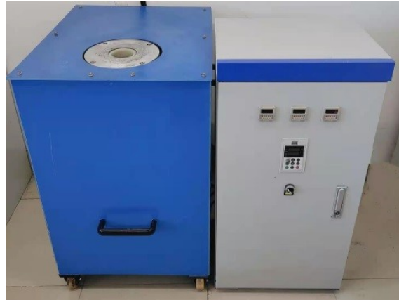
Figure S1. Magnetic Grinding equipment
