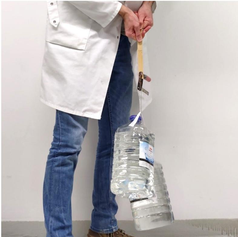
Fig. S18. EKL+LNP adhesive lifting 10 kg. The sample had a joint area of 1 cm<sup>2</sup> and was glued with a spread of 100 g/m<sup>2</sup> and was hot pressed at 130 °C for 5 minutes. The water jugs contained about 5 liters each and weighed exactly 10.0 kg in total. A video of lifting the jugs from the ground can be found in the supplementary video.
