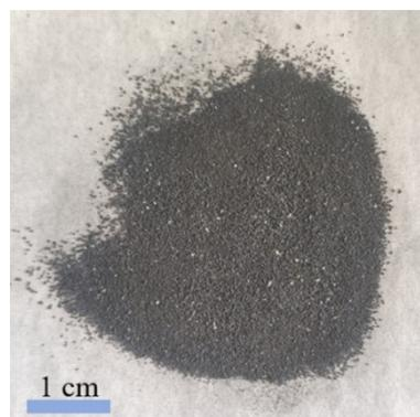
Fig. S2 S-LFP cathode powder stemming from retired LFP battery.
