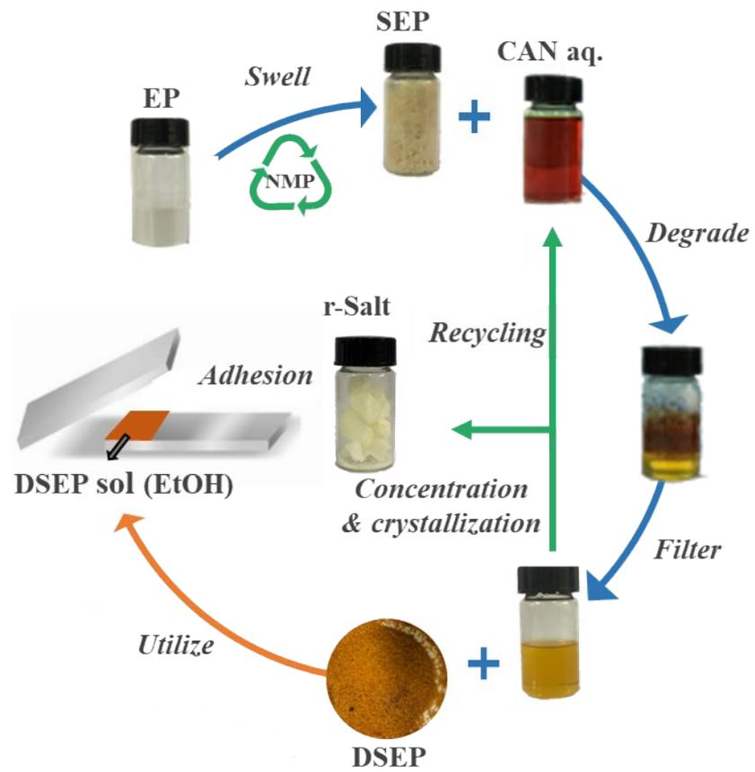
**Figure S8** Schematic diagram of the full recovery
