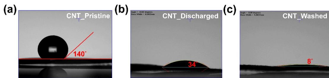
**Fig. S2.** Contact angle of water droplet on (a) pristine, (b) discharged, and (c) washed CNT cathode.
