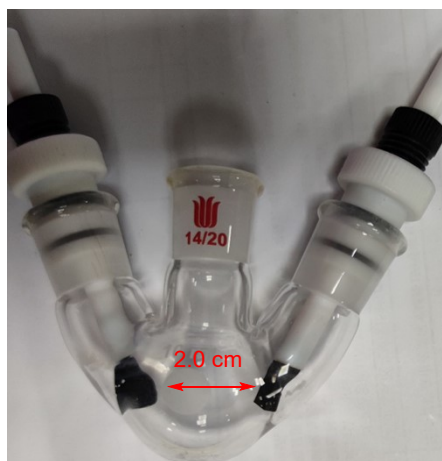
Figure S3. Micro electrosynthesis equipment.
