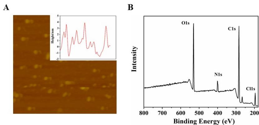
**Fig. S3** A. AFM image of CCDs. The inset shows the particle size distribution of CCDs; B. XPS full spectrum of CCDs.
