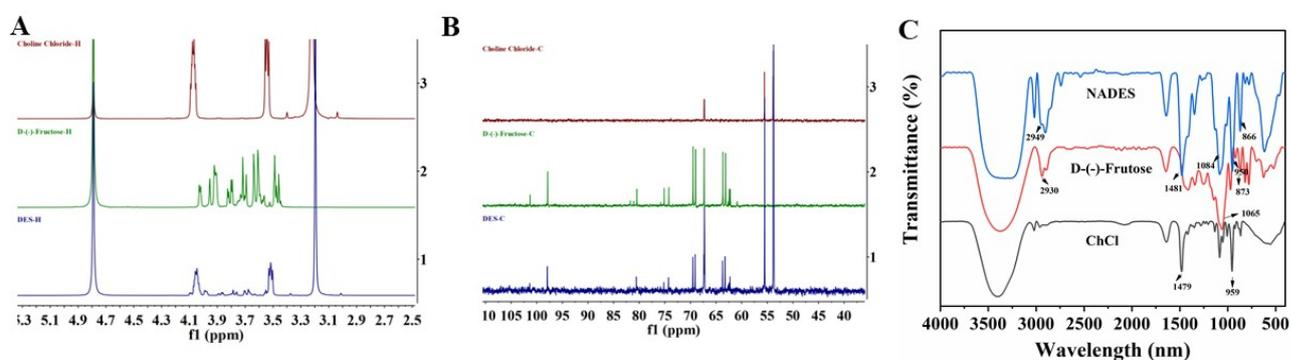
**Fig. S2** NMR (A, B) and FT-IR (C) spectra of DESs raw materials, DESs, and CCDs.
