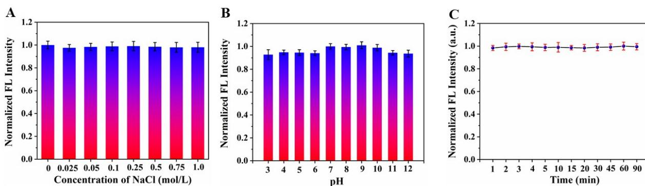
Fig. S5 Effect of concentration of NaCl and pH value on the fluorescence intensity of CCDs aqueous solution (A, B). C. The stability of CCDs.
