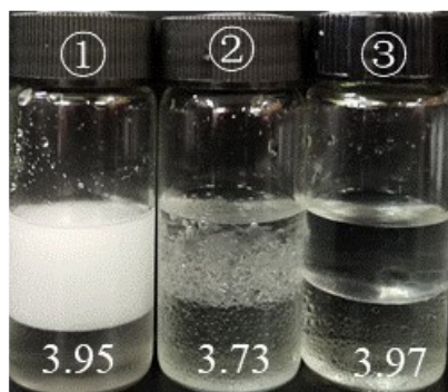
Figure S11. Digital photos of n -decane-in-water (7 mL/7 mL) conventional emulsions stabilized by (1) \text{H}^+\text{AA} at \text{pH} = 4 , (2) \text{AA}^- (original \text{pH} = 12 but was reduced to \text{pH} = 4 by addition of \text{HCl} ), (3) \text{FA-AA} (original \text{pH} = 12 but was reduced to \text{pH} = 4 by addition of \text{HCl} ) all at 6 mM taken immediately after preparation at 25 °C.
