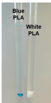
Figure S4. NMR tubes after depolymerisation of blue and white **PLA**, with the deposits of the additives in the crude mixture.
