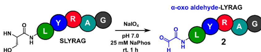
Figure S35. The preparation of \alpha -oxo aldehyde-LYRAG from SLYRAG using previously reported conditions. 3
