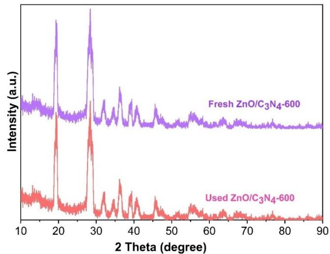
**Figure S5** XRD patterns of fresh and used  $\text{ZnO}/\text{C}_3\text{N}_4$ -600
