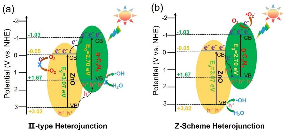
**Figure S9.** Scheme of the heterojunction type of ZnO/C<sub>3</sub>N<sub>4</sub> photocatalysts.
