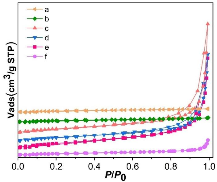
**Figure S4** The  $\text{N}_2$  adsorption/desorption isotherms of the (a)  $\text{ZnO}/\text{C}_3\text{N}_4$ -800, (b)  $\text{ZnO}/\text{C}_3\text{N}_4$ -700, (c)  $\text{ZnO}/\text{C}_3\text{N}_4$ -600, (d)  $\text{ZnO}/\text{C}_3\text{N}_4$ -500, (e)  $\text{ZnO-C}$ , (f)  $\text{ZnO-A}$ .
