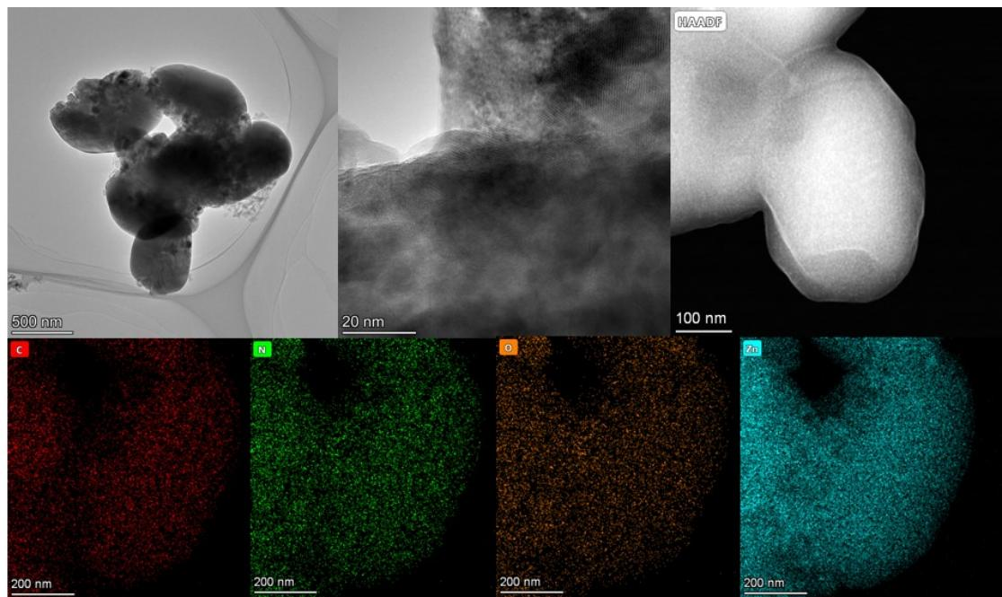
**Figure S7** TEM images and the EDX mapping images of used ZnO/C<sub>3</sub>N<sub>4</sub>-600 catalyst.
