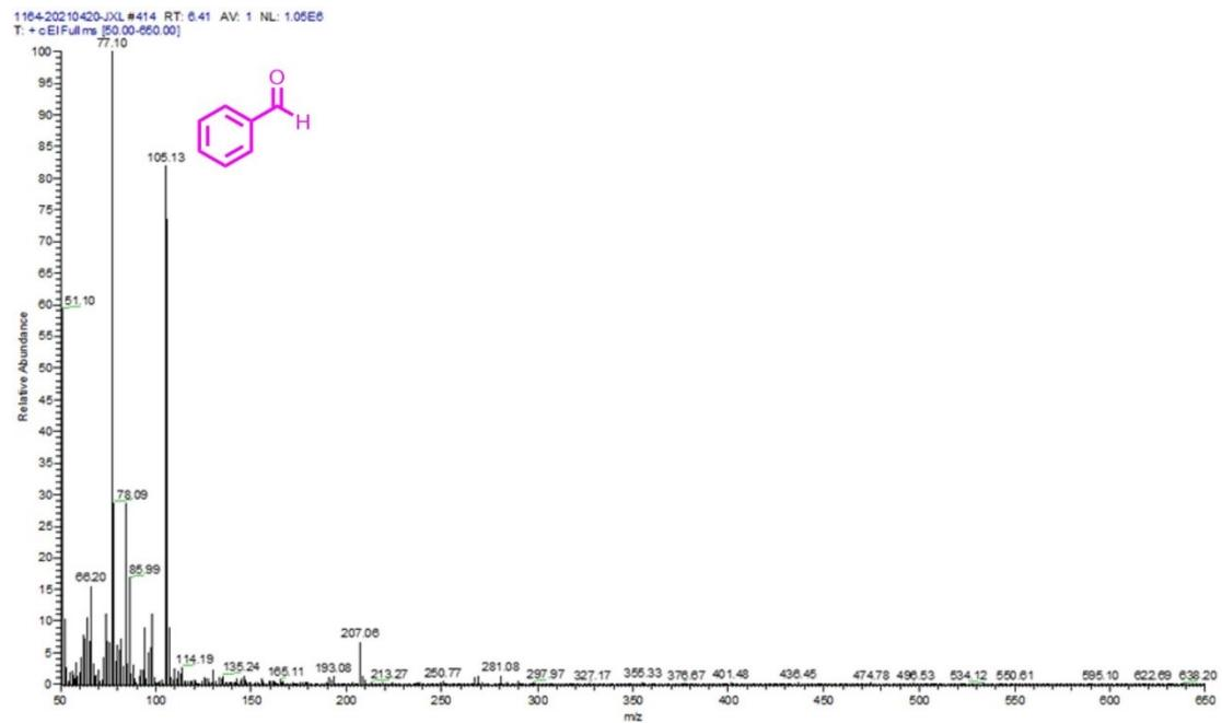
**Figure S1** The MS of benzaldehyde product detected by GC-MS.
