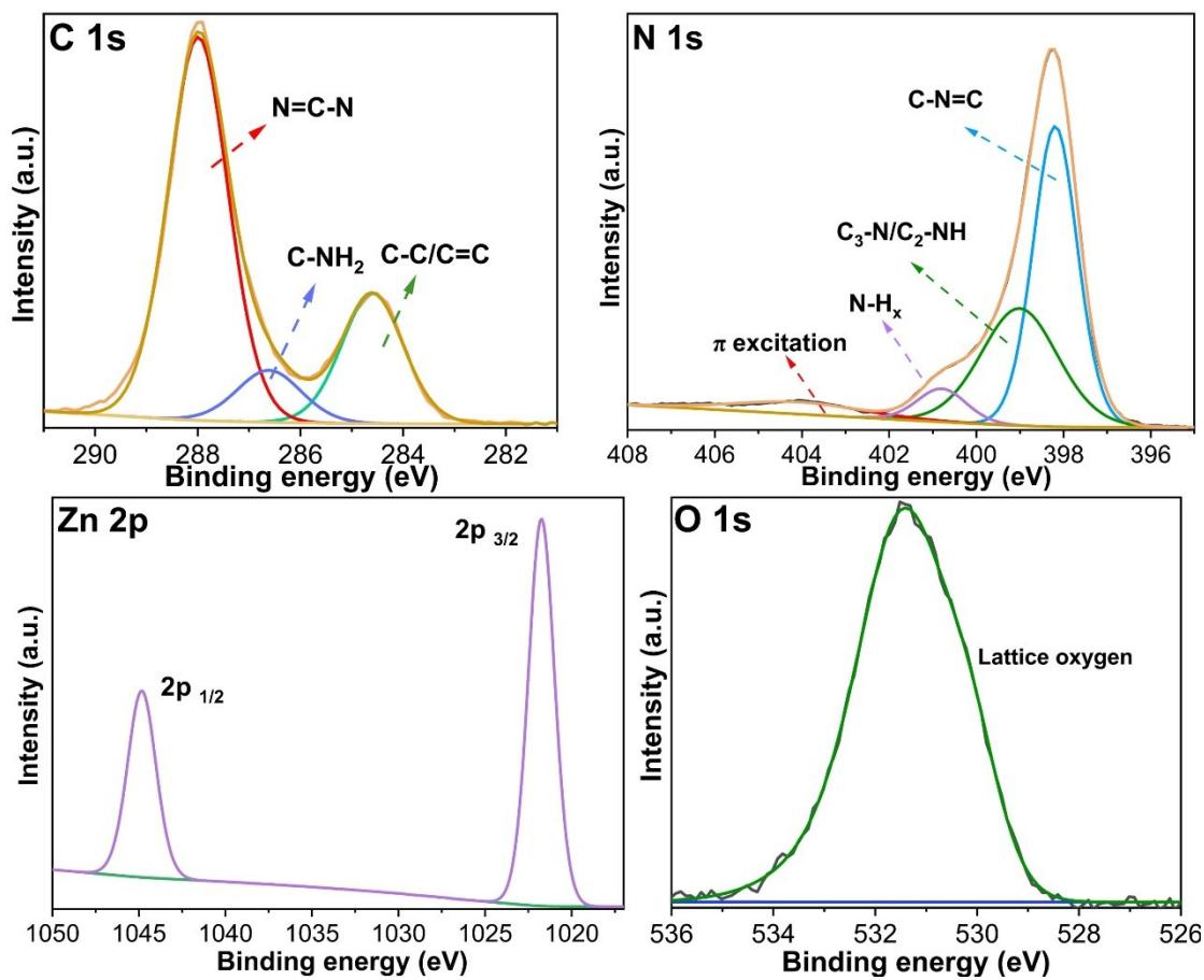
**Figure S8** XPS spectra of used ZnO/C<sub>3</sub>N<sub>4</sub>-600 catalyst.
