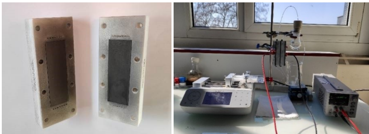
Figure S1: left: Graphite Electrodes and right: experimental set-up for the electrochemical trifluoromethylation in flow
