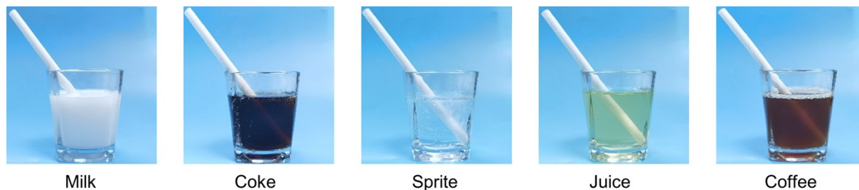
Figure S24. RM paper-20 straws are soaked in different drinks. RM paper-20 straws also show excellent liquid resistance for different drinks.
