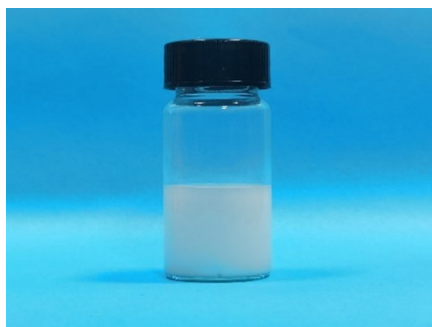
Figure S3. Photograph of RM emulsion. Cationic starch makes RM emulsion positively charged, which is not only conducive to maintaining emulsion stability, but also conducive to the adsorption of RM on cellulose fibers.
