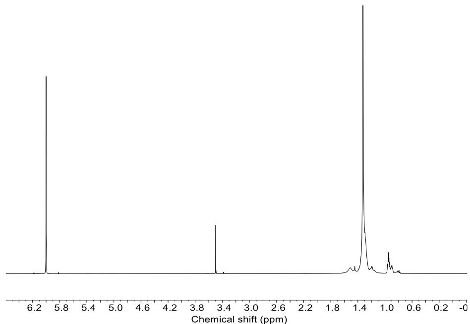
**Figure S5.** <sup>1</sup>H NMR spectrum ( $C_2D_2Cl_4$ , 80 °C) of the PE product after a 24 hour reaction in benzaldehyde at 120 °C under an inert Ar atmosphere (Table 1, entry 2).
