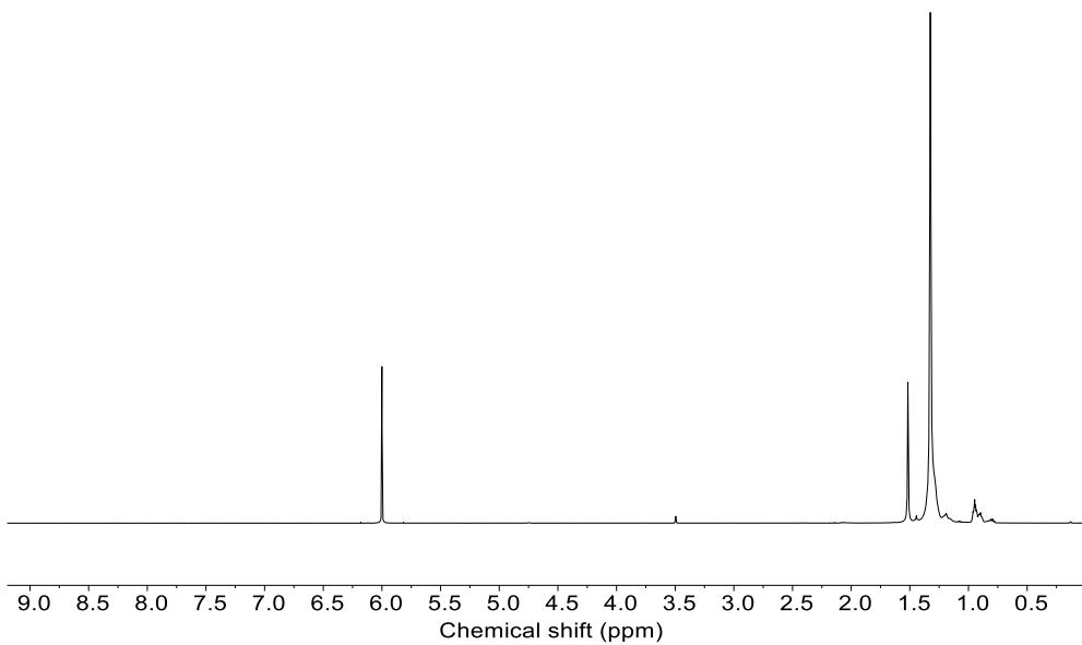
**Figure S10.** <sup>1</sup>H NMR spectrum ( $\text{C}_2\text{D}_2\text{Cl}_4$ , 80 °C) of the PE product after stirring for 24 hours in 1,2,4-TCB under  $\text{O}_2$  without benzaldehyde at 120 °C (Table 1, entry 7).
