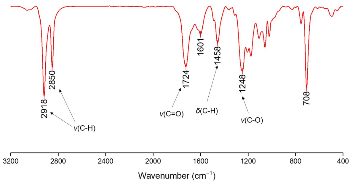
**Figure S25.** FTIR spectrum of PE after oxidation using benzaldehyde at 120 °C under O<sub>2</sub> in the presence of [CuCl<sub>2</sub>·DCH18-crown-6] (1 mol%).
