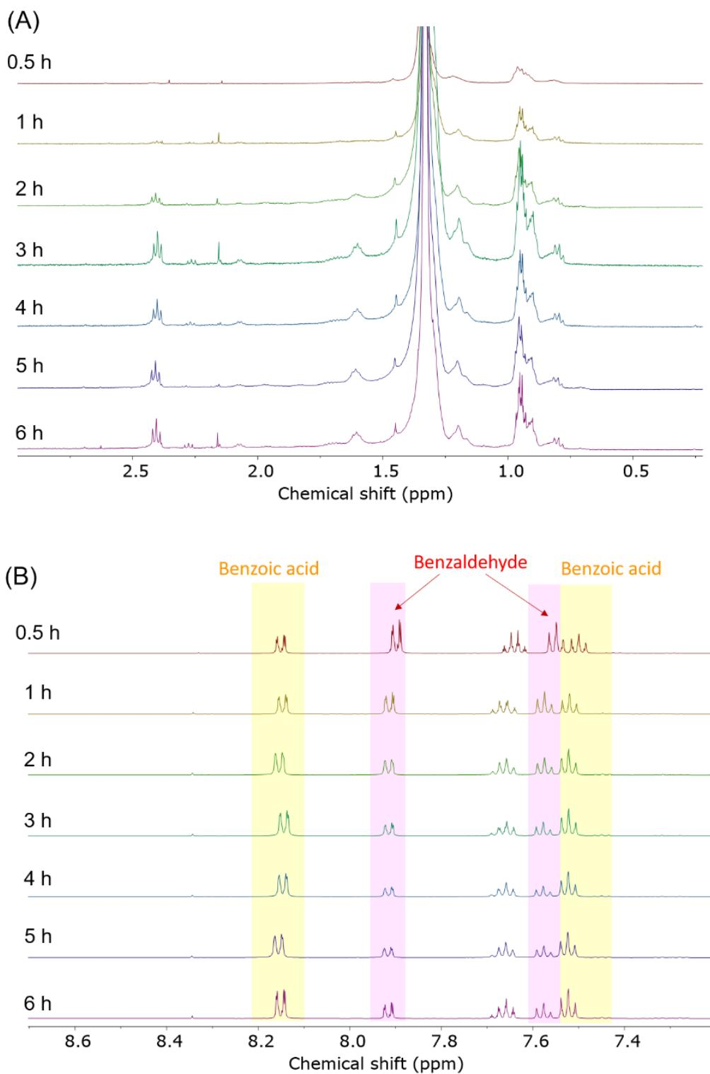
**Figure S1.** Stacked  $^1\text{H}$  NMR spectra ( $\text{C}_2\text{D}_2\text{Cl}_4$ , 80 °C) showing appearance of (A) a peak at 2.40 ppm arising from the carbonyl  $\alpha$ -H on PE and (B) the corresponding formation of benzoic acid from benzaldehyde as the reaction progresses.
