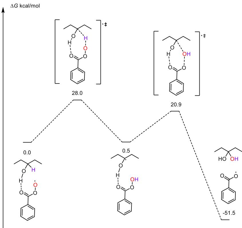
**Figure S26.** Reaction of benzoylperoxy radical with 3-pentanol via an oxygen rebound mechanism.
