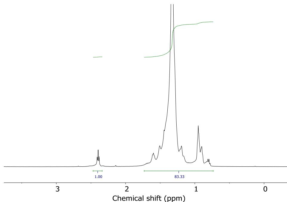
**Figure S3.**  $^1\text{H}$  NMR spectrum ( $\text{C}_2\text{D}_2\text{Cl}_4$ ,  $80^\circ\text{C}$ ) of the oxidised PE using benzaldehyde at  $120^\circ\text{C}$  (Table 1, entry 1).
