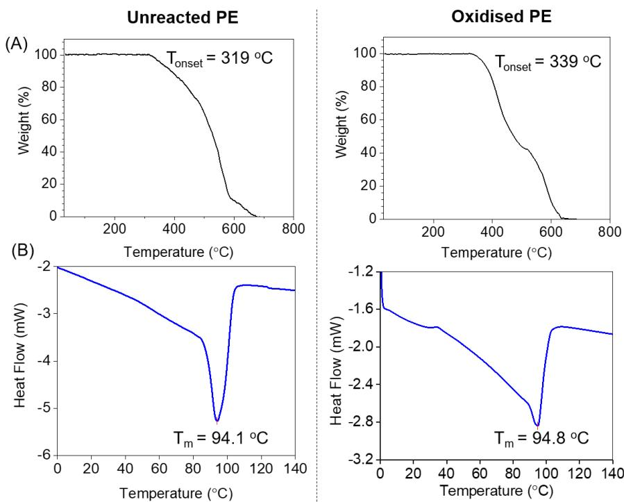
**Figure S22.** Comparisons of the properties of the (left panel) unreacted PE with the (right panel) carbonyl-containing oxidised PE (from Table 1, entry 1): (A) TGA curves, with the onset temperature of weight loss indicated; (B) DSC traces.
