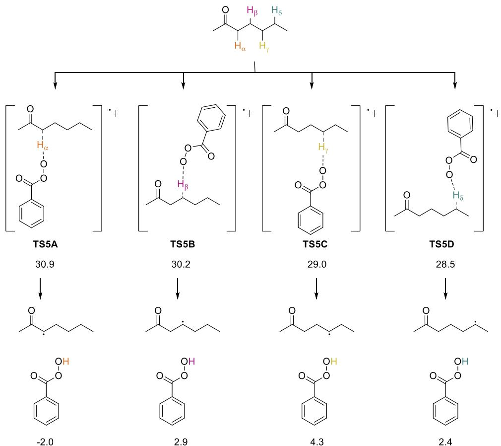
**Scheme S1:** Reaction free energies of hydrogen atom transfer reactions between 2-heptone and benzoylperoxy radical, at various positions along the 2-heptone chain.
