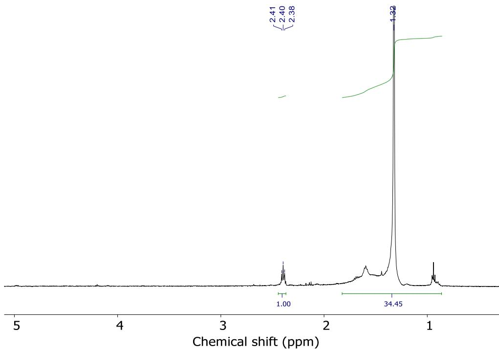
**Figure S23.** <sup>1</sup>H NMR spectrum ( $\text{C}_2\text{D}_2\text{Cl}_4$ , 80 °C) of the oxidised LDPE plastic bag after a 24 hour reaction in benzaldehyde at 120 °C under  $\text{O}_2$ .
