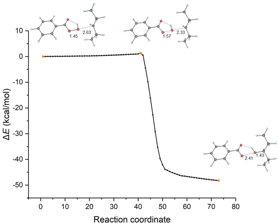
**Figure S27.** Intrinsic reaction coordinate for hydroxyl transfer from peroxybenzoic acid to the C-centered radical, calculated at B3LYP-D3BJ/def-TZVP level of theory.
