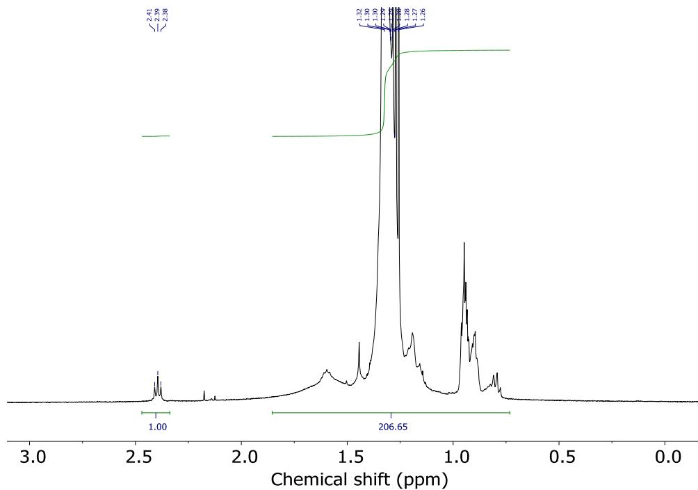
**Figure S7.** <sup>1</sup>H NMR spectrum ( $\text{C}_2\text{D}_2\text{Cl}_4$ , 80 °C) of the PE product after a 24 hour reaction in benzaldehyde at 100 °C under  $\text{O}_2$  (Table 1, entry 4).
