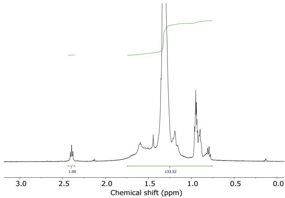
**Figure S6.** <sup>1</sup>H NMR spectrum ( $\text{C}_2\text{D}_2\text{Cl}_4$ , 80 °C) of the PE product after a 24 hour reaction in benzaldehyde at 120 °C in air (Table 1, entry 3).
