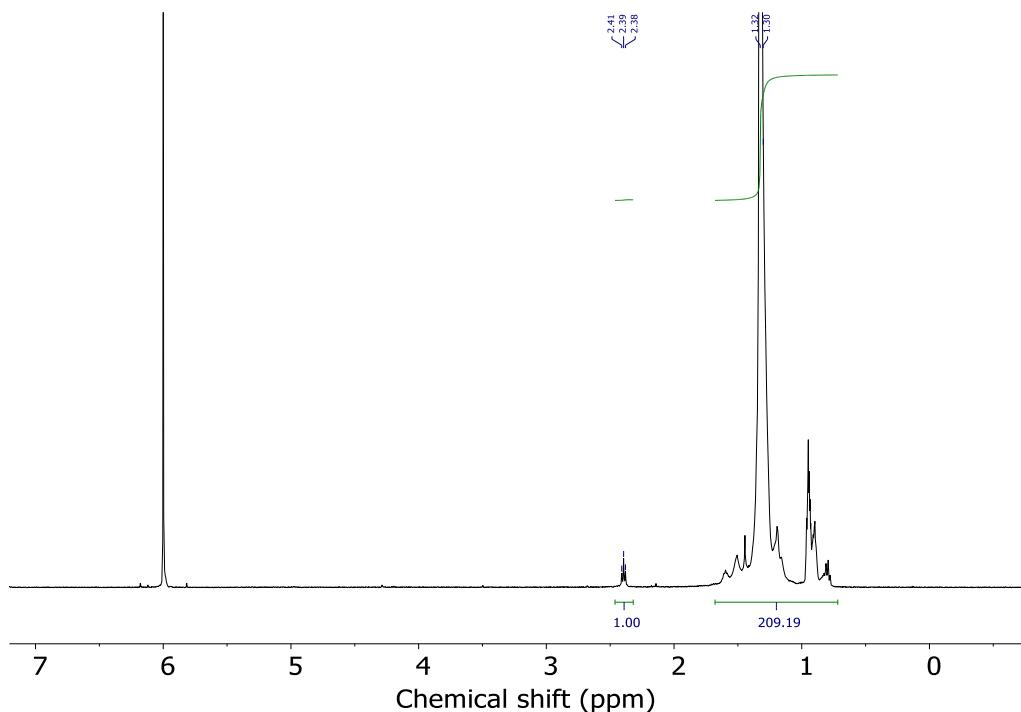
**Figure S9.** <sup>1</sup>H NMR spectrum ( $\text{C}_2\text{D}_2\text{Cl}_4$ , 80 °C) of the PE product after a 24 hour reaction in the presence of 1 equivalent of benzaldehyde at 120 °C under  $\text{O}_2$  (Table 1, entry 6).
