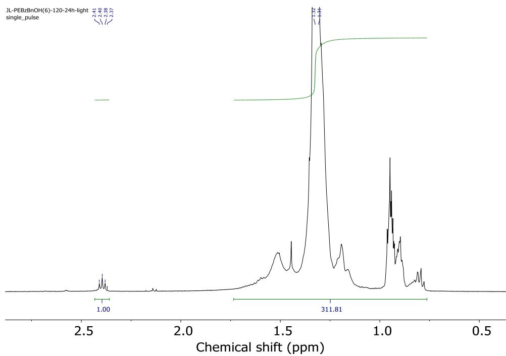
**Figure S14.**  $^1\text{H}$  NMR spectrum ( $\text{C}_2\text{D}_2\text{Cl}_4$ , 80 °C) of the oxidised PE using benzaldehyde with 6 eqv of benzyl alcohol at 120 °C under  $\text{O}_2$  (Table 1, entry 11).
