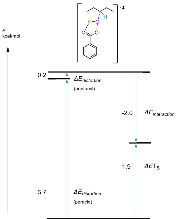
**Figure S28.** Distortion-interaction energy of **TS2B**.
