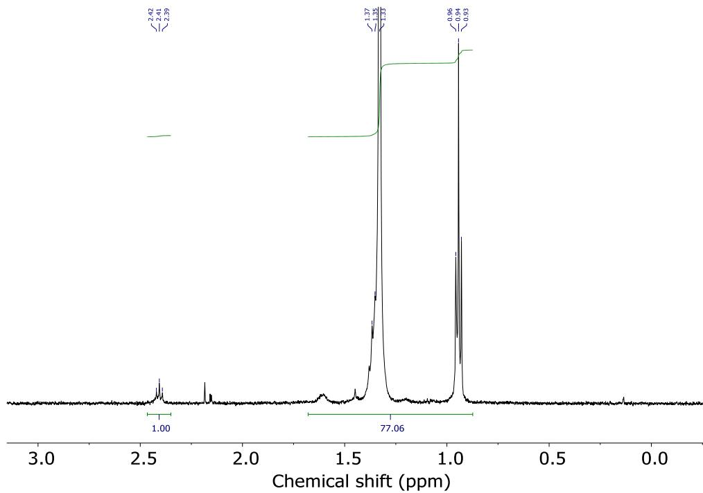
**Figure S18.** <sup>1</sup>H NMR spectrum ( $\text{C}_2\text{D}_2\text{Cl}_4$ , 80 °C) of the oxidised icosane ( $\text{C}_{20}\text{H}_{42}$ ) using benzaldehyde at 120 °C under  $\text{O}_2$ .
