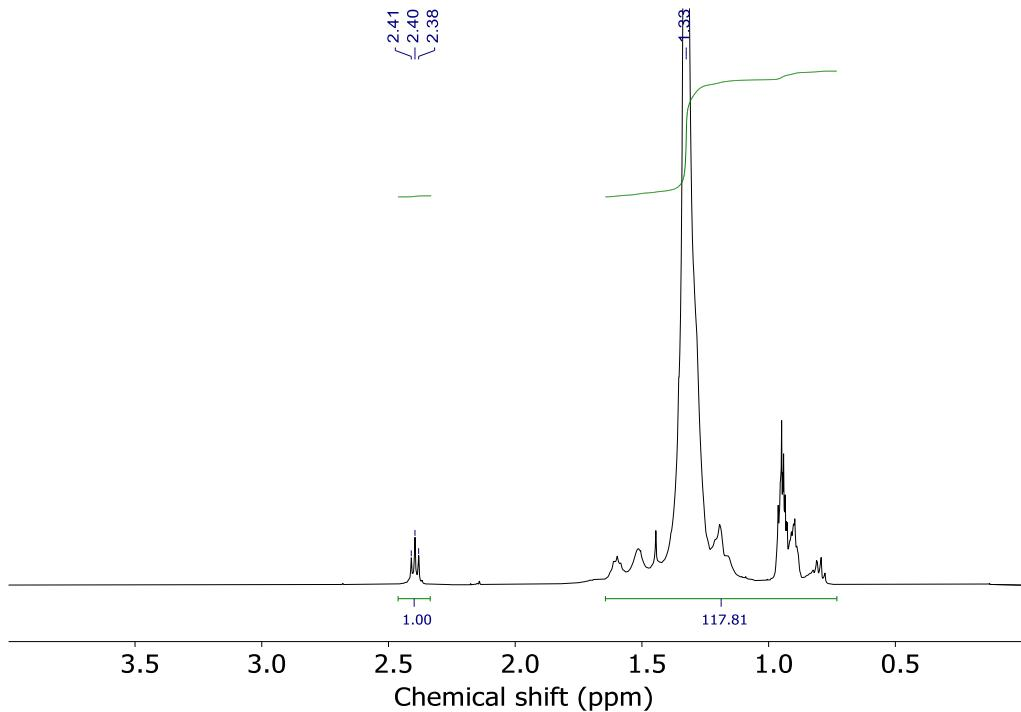
**Figure S19.**  $^1\text{H}$  NMR spectrum ( $\text{C}_2\text{D}_2\text{Cl}_4$ ,  $80^\circ\text{C}$ ) of the PE product after a 24 hour reaction at  $120^\circ\text{C}$  under  $\text{O}_2$  on a larger scale with 2.5 g PE starting material. A brand-new, unused stirrer bar was used for this reaction, which was soaked for 24 hours in aqua regia with the glassware used, to exclude the possibility of trace metal contamination being responsible for the PE oxidation observed.
