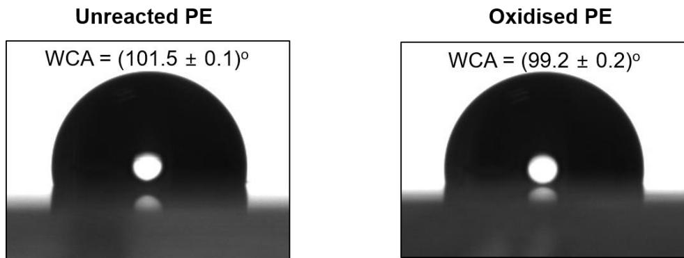
**Figure S20.** Contact angle images of water droplets on a film of unreacted PE and oxidised PE.
