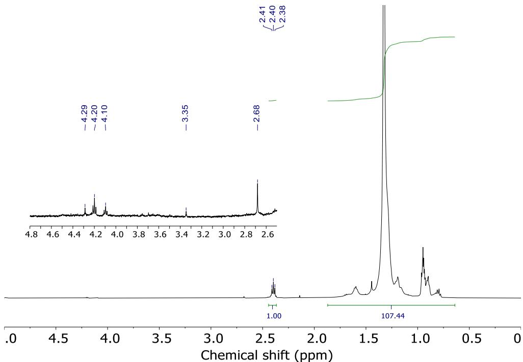
**Figure S24.** <sup>1</sup>H NMR spectrum ( $\text{C}_2\text{D}_2\text{Cl}_4$ , 80 °C) of the oxidised PE using benzaldehyde with 6.7 mL of 1,2,4-TCB (equivalent volume to 6 eqv of benzyl alcohol) at 120 °C under  $\text{O}_2$ .
