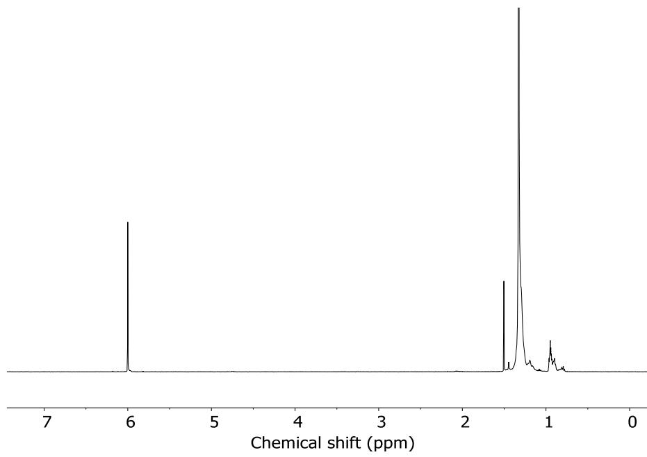
**Figure S17.** <sup>1</sup>H NMR spectrum ( $\text{C}_2\text{D}_2\text{Cl}_4$ , 80 °C) of the PE material after a 24 hour reaction at 120 °C under  $\text{O}_2$  in the absence of benzaldehyde. The reaction was conducted neat without any solvents.
