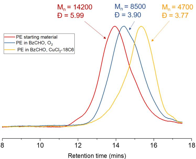
**Figure S21.** Stacked normalised GPC spectra showing changes in molecular weight distribution of PE before and after oxidation using benzaldehyde at 120 °C under O<sub>2</sub>, and after oxidation using benzaldehyde at 120 °C under O<sub>2</sub> in the presence of [CuCl<sub>2</sub>·DCH18-crown-6] (1 mol%).
