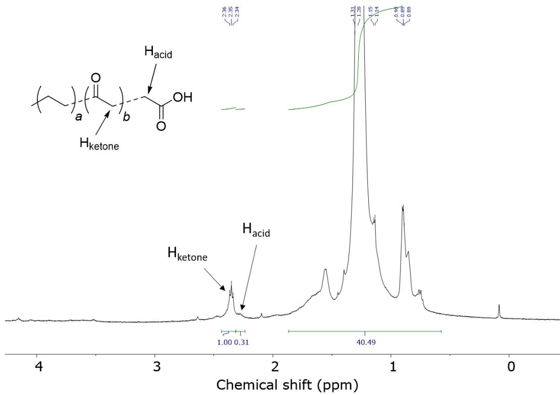
**Figure S15.**  $^1\text{H}$  NMR spectrum ( $\text{C}_2\text{D}_2\text{Cl}_4$ ,  $80^\circ\text{C}$ ) of the oxidised PE using benzaldehyde with  $[\text{CuCl}_2\cdot\text{DCH18-crown-6}]$  (1 mol%) at  $120^\circ\text{C}$  under  $\text{O}_2$  (Table 1, entry 12).
