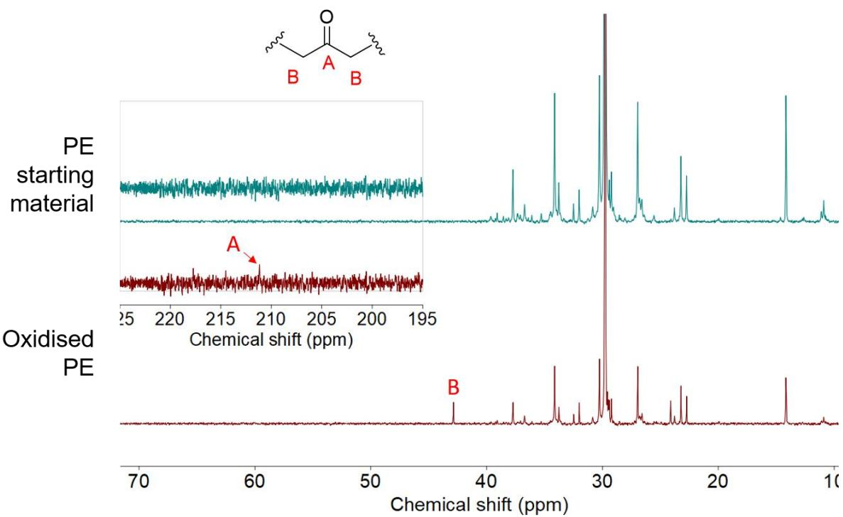
**Figure S2.** Stacked  $^{13}\text{C}$  NMR spectra ( $\text{C}_2\text{D}_2\text{Cl}_4$ ,  $80^\circ\text{C}$ ) of the PE starting material and the oxidised PE from Table 1 entry 1. Assignments are based on those reported by Nozaki and coworkers.<sup>1</sup>
