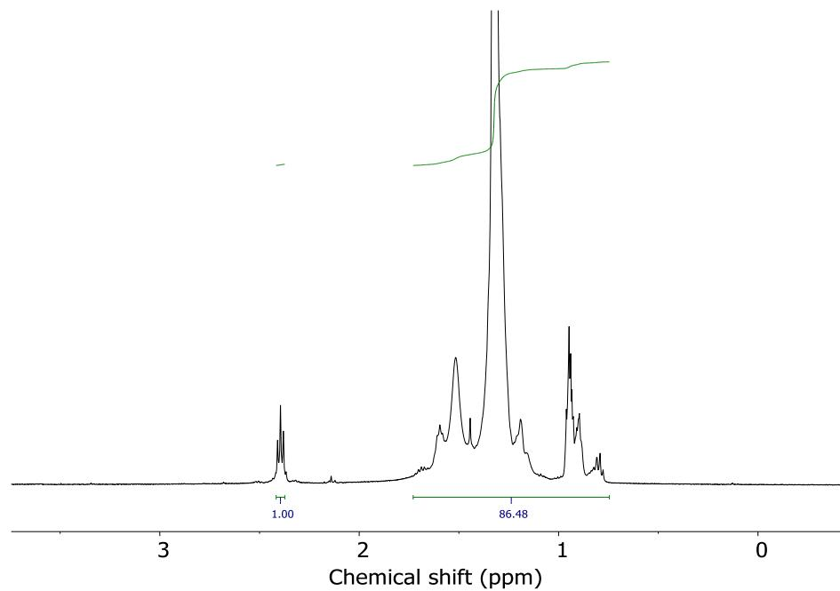
**Figure S11.** <sup>1</sup>H NMR spectrum ( $\text{C}_2\text{D}_2\text{Cl}_4$ , 80 °C) of the oxidised PE using benzaldehyde at 120 °C under  $\text{O}_2$  in the dark (Table 1, entry 8).
