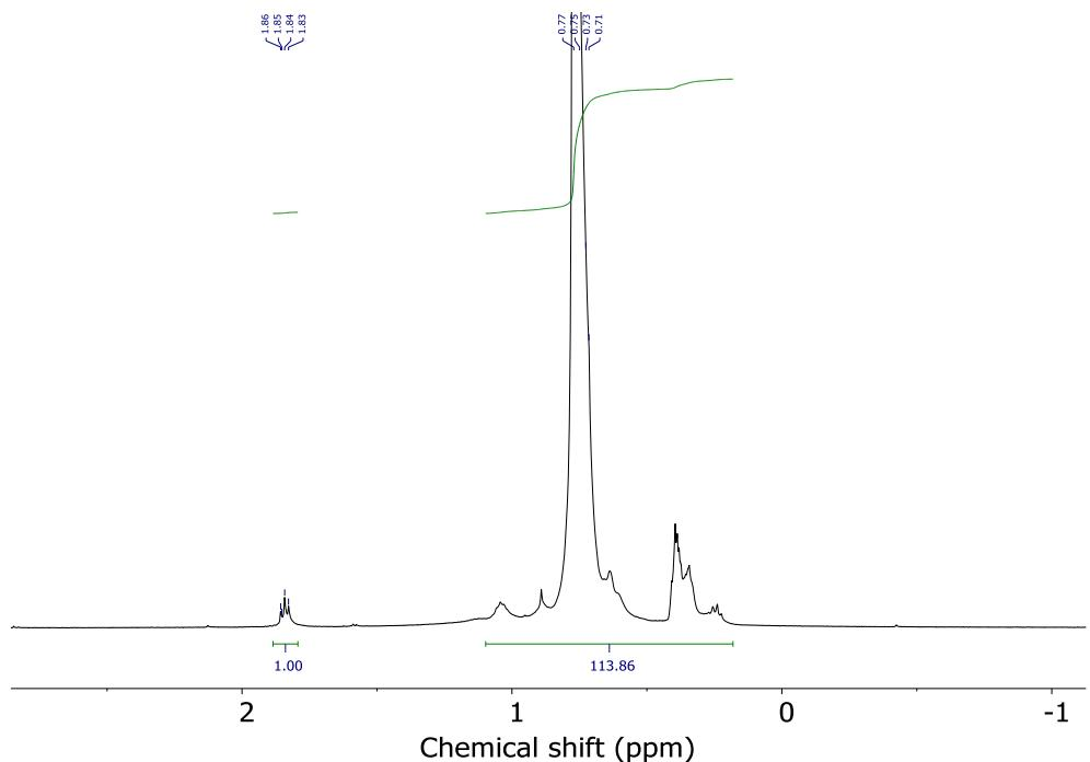
**Figure S13.**  $^1\text{H}$  NMR spectrum ( $\text{C}_2\text{D}_2\text{Cl}_4$ , 80 °C) of the oxidised PE using benzaldehyde with 1 equiv of benzyl alcohol at 120 °C under  $\text{O}_2$  (Table 1, entry 10).
