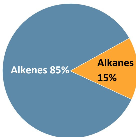
Fig. S9. Selectivity of hydrocarbons obtained from non-catalytic tandem conversion of disposable masks: Conversion = 99.1%
