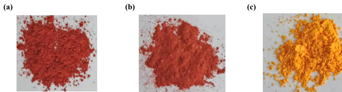
Fig. S7. Pictures of the fresh BiOI nanosheets catalyst (a), the used BiOI nanosheets catalyst (b), and the catalyst after calcination at 400 °C(c), respectively.
