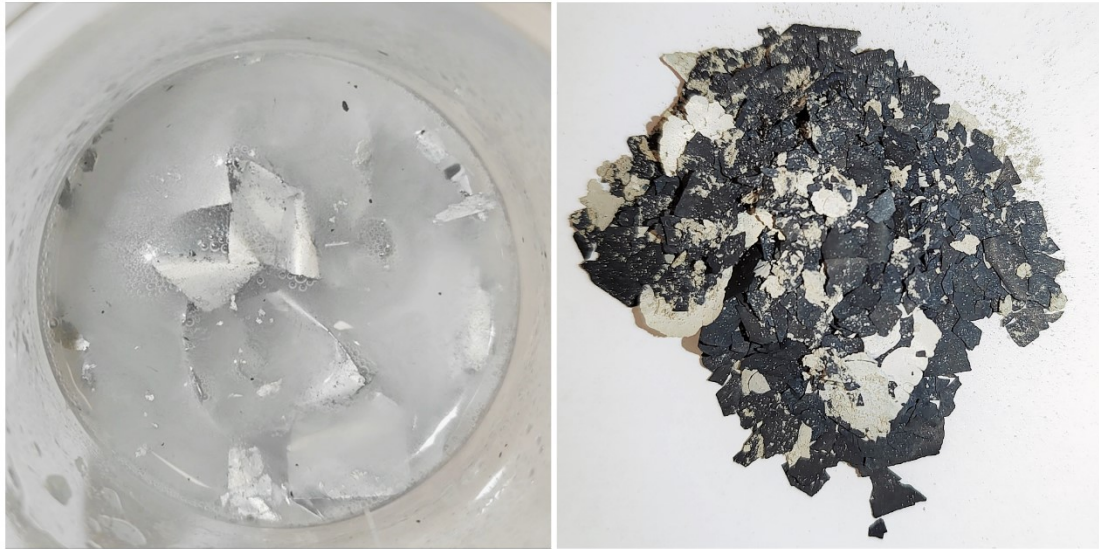
Fig. S4 The reaction phenomenon of cathode electrode in 20% \text{K}_2\text{CO}_3 water solution. Gas is clearly seen generating from the solution, and the Al foil is being corroded quickly (left). After reaction, Al foil has been severely corroded and mixed with the active material, making them impossible to be separated (right).
