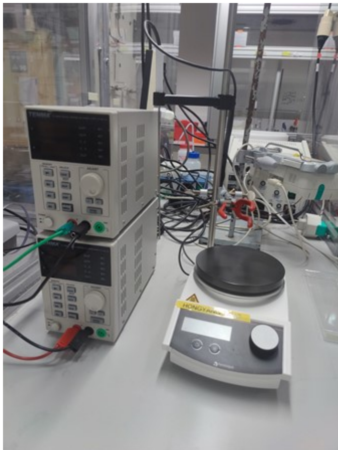
Figure S5. Power supply and magnetic stirrer for the electrocatalytic formation of epoxides.
