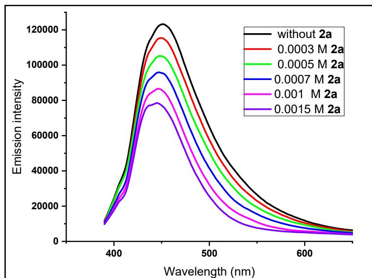
**Figure S6:** Emission spectra of PC-1 at different concentration of **2a**
