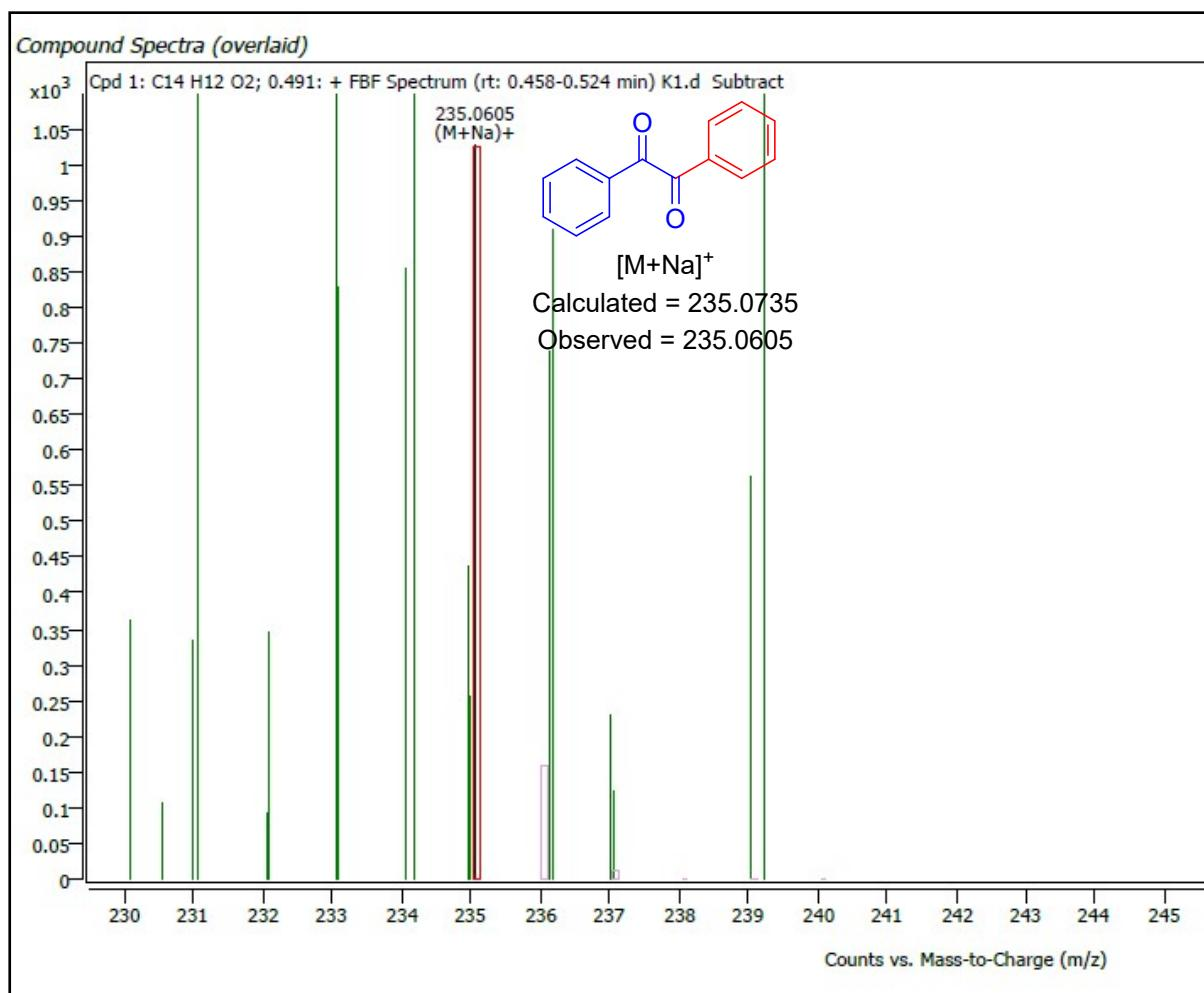
**Figure S3:** Analysis of reaction mixture by HRMS
