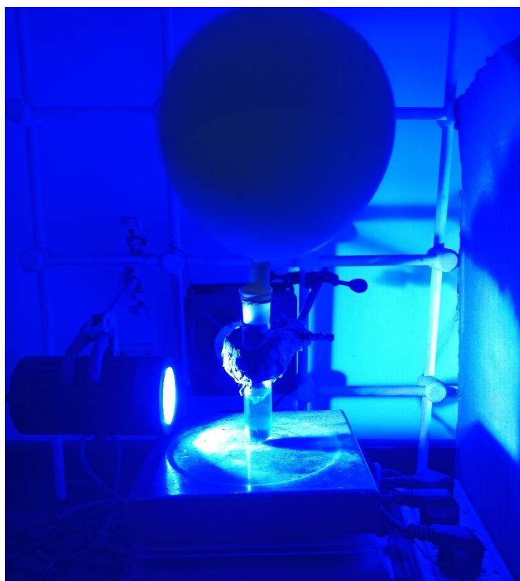
**Figure S1:** Reaction setup with Kessil PR160L-456nm Blue LED
