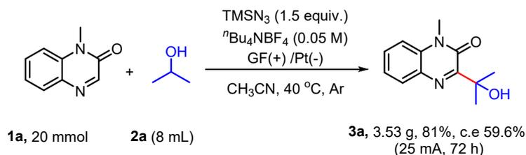
To an undivided three-necked flask (250 mL) were added 1-methylquinoxalin-2(1H)-one (**1a**, 3.20 g, 20 mmol), isopropanol (**2a**, 8.0 mL), TMSN<sub>3</sub> (3.46 g, 3.96 mL, 30.0 mmol, 1.5 equiv.) and CH<sub>3</sub>CN (100 mL). The flask was equipped with graphite felt as anode and platinum plate
