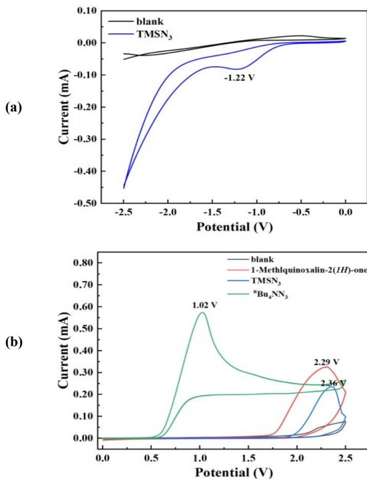
**Figure S1** CV scans (scan rate  $100 \text{ mV}\cdot\text{s}^{-1}$ ) of substrates: (a) Blank ( $n\text{Bu}_4\text{NBF}_4$  (0.01 M) in MeCN); TMSN<sub>3</sub> (0.02 M, blue curve). (b) Blank ( $n\text{Bu}_4\text{NBF}_4$  (0.02 M) in MeCN); 1-Methylquinoxalin-2(1H)-one (**1a**, 0.02 M, red curve); TMSN<sub>3</sub> (0.02 M, blue curve);  $t\text{Bu}_4\text{NN}_3$  (0.02 M, green curve).
