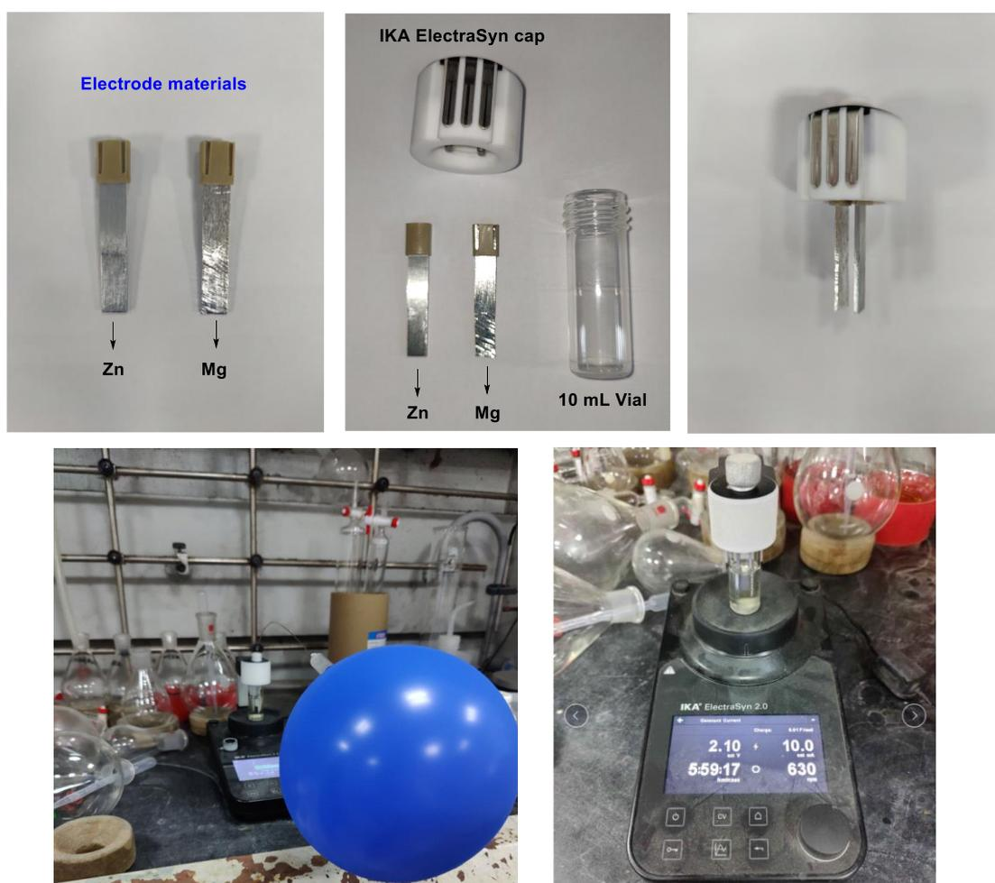
**Figure S1** Experimental setup (IKA ElectraSyn 2.0)
