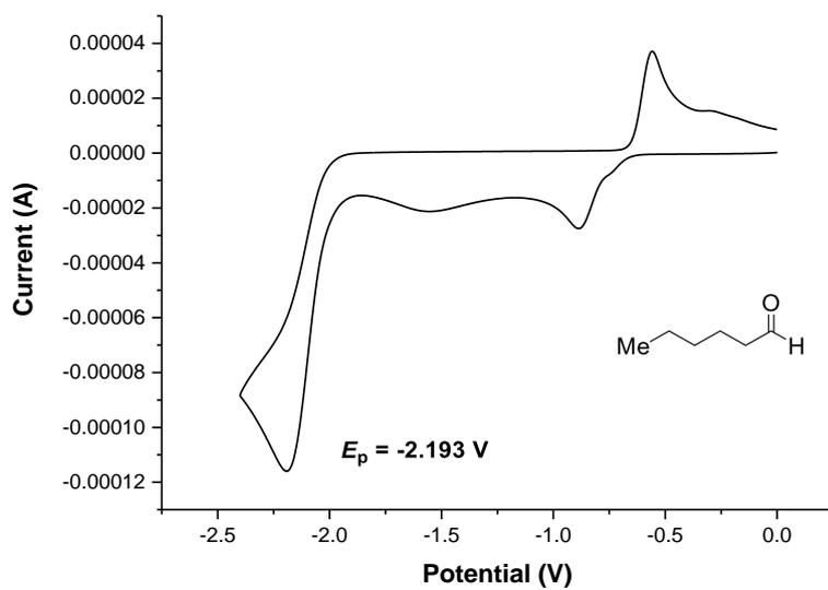
**Figure S5** Cyclic voltammograms for hexanal
