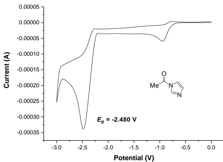
**Figure S10** Cyclic voltammograms for 1-(1H-imidazol-1-yl)ethan-1-one
