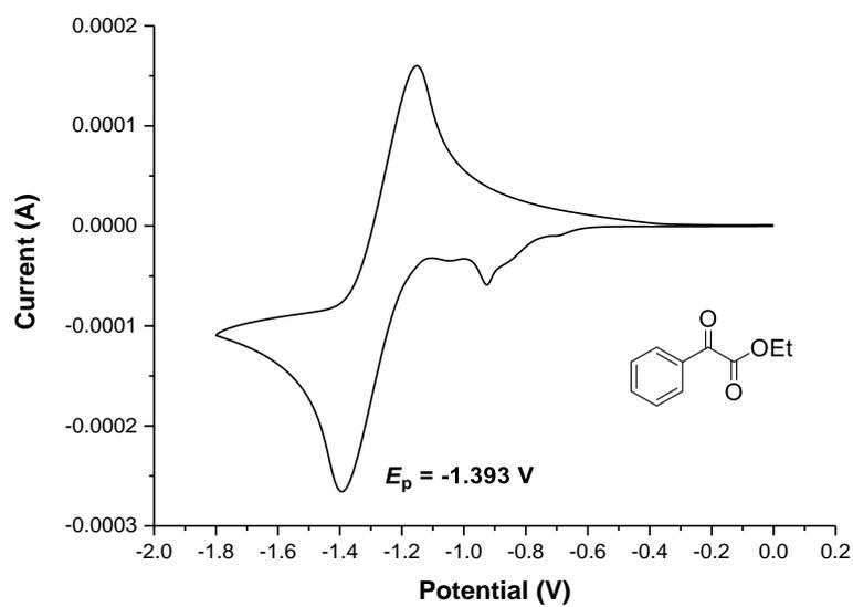
**Figure S7** Cyclic voltammograms for ethyl 2-oxo-2-phenylacetate
