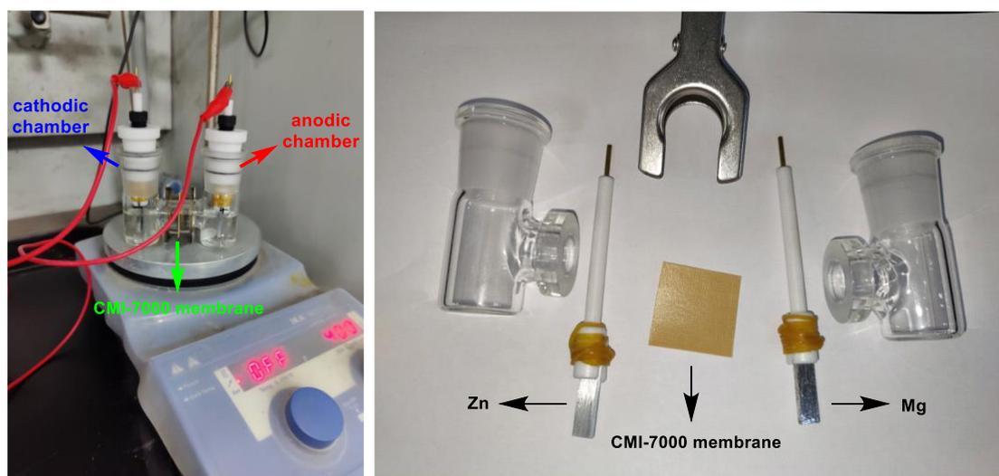
**Figure S2** Reaction setup for divided cell electrolysis
