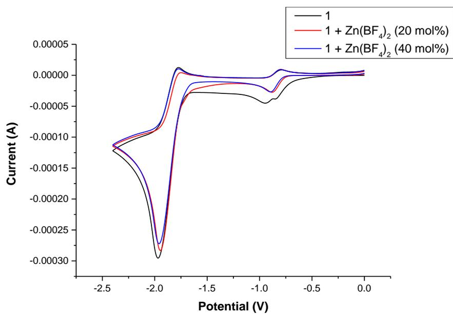
**Figure S11** Cyclic voltammograms for benzaldehyde (1) +  $Zn(BF_4)_2$
