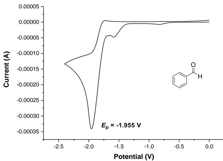
**Figure S4** Cyclic voltammograms for benzaldehyde
