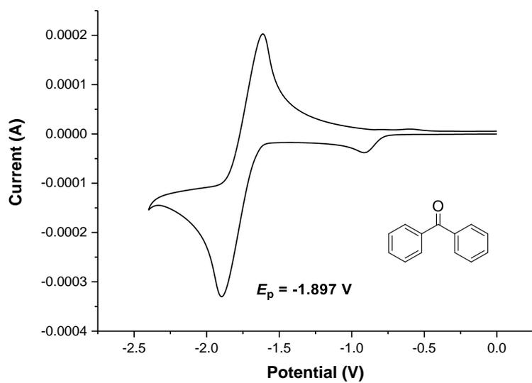
**Figure S6** Cyclic voltammograms for benzophenone
