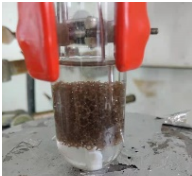
Figure S5. Standard setup for all semi-hydrogenation experiments.
