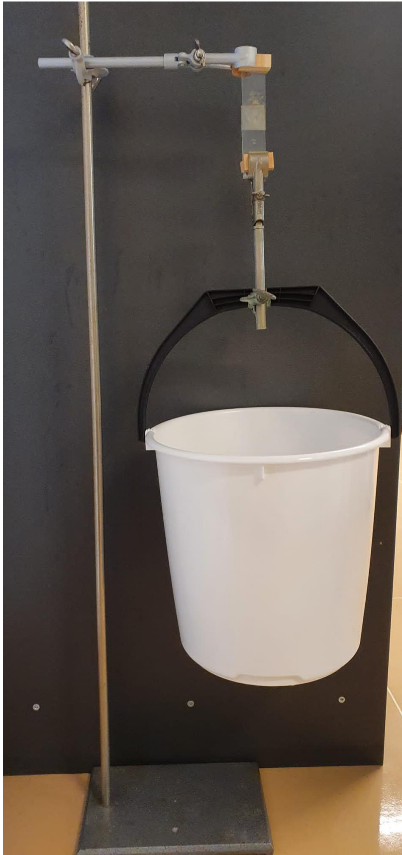
Figure S9. Experimental setup for shear mechanical tests. Glass joints were tightened by a grip and a load of increasing weight was added in the bucket.
