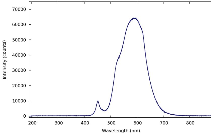
**Figure S4.** Measured wavelength of distribution for neutral white LED strip.
