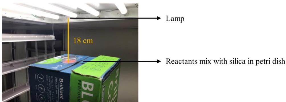
**Figure S12.** Reaction setup for solvent-free silica-supported lamp irradiation
