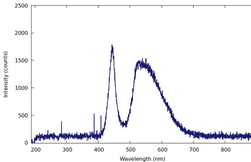
**Figure S3.** Measured wavelength of distribution for white LED strip.
