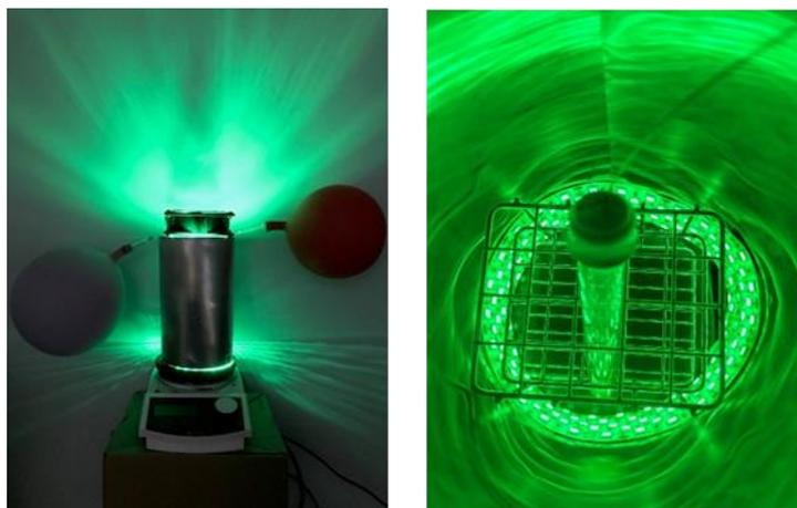
**Figure S1.** Actual reaction setup for light irradiation using LED strip.
