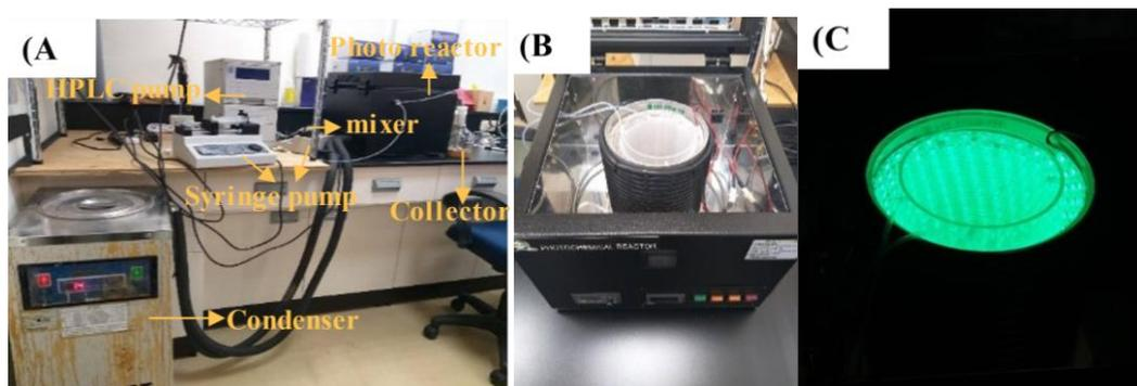
**Figure S7.** Reaction setup using the photoflow system: (A) full system; (B) photoflow reactor; and (C) “turned on” light source
