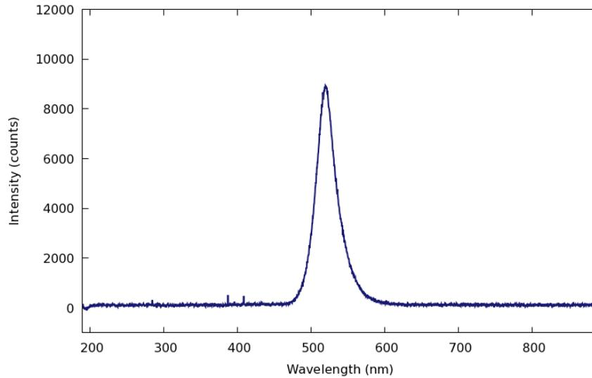
**Figure S2.** Measured wavelength of distribution for green LED strip.
