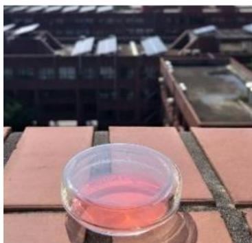
**Figure S10.** Reaction setup for solvent-free silica-supported sunlight exposure.
