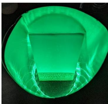
**Figure S8.** Reaction setup for TLC glass plate irradiation using green LED.
