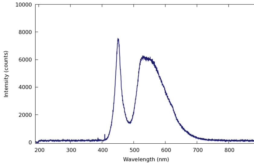
**Figure S5.** Measured wavelength of distribution for pure white LED strip.
