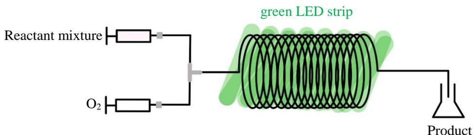
**Figure S6.** Schematic diagram for the photoflow reactor setup.
