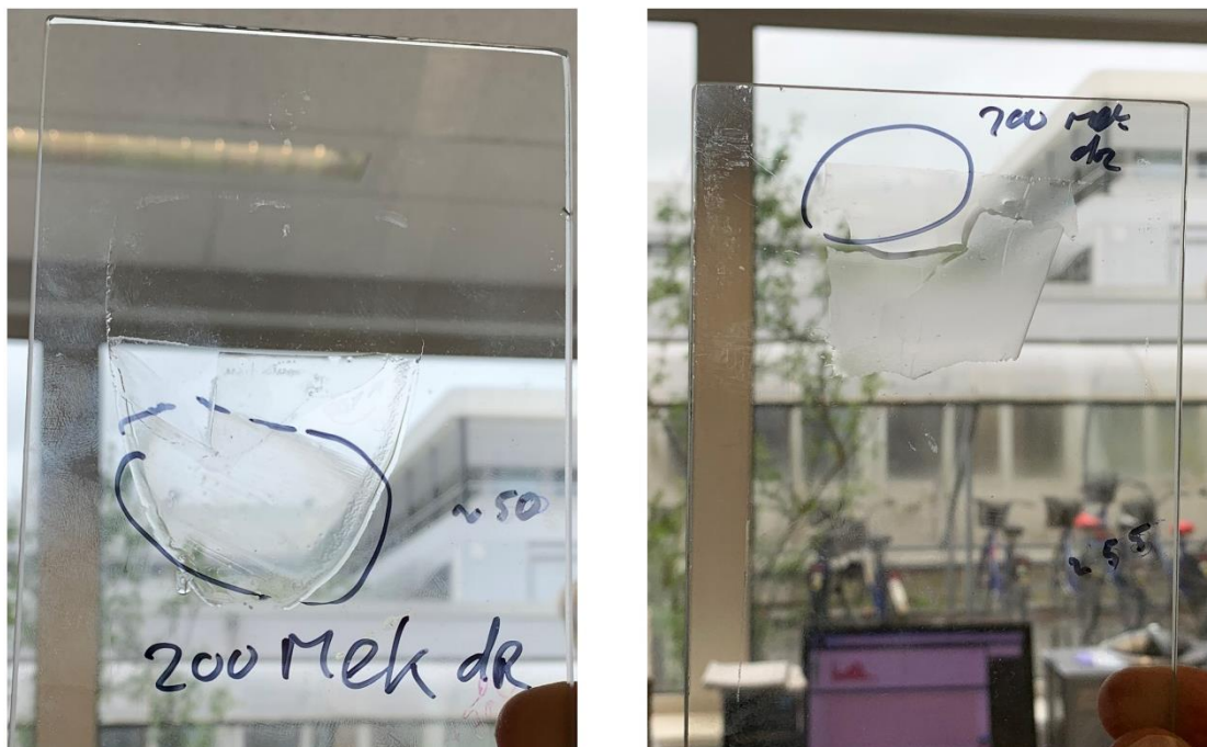
Figure S25 UV cured methoxybutenolide–1,4-butanedivinyl ether coatings BVEC1 (left) and BVEC2 (right) subjected to DSC, Knoop hardness measurement and MEK solvent resistance test. Only slight whitening and no other damage or deterioration of the surfaces was apparent after 200 MEK double rubs.
