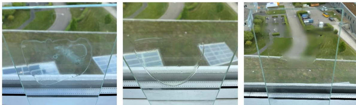
Figure S23 UV cured methoxybutenolide–1,4-butanediviny ether coatings using as photoinitiator 3 mol% VAPO (left), 6 mol% VAPO (middle) and 3 mol% BAPO (right). Coating formation conditions: methoxybutenolide–1,4-butanediviny ether (1:0.5 ratio), VAPO/BAPO (3–6 mol%), UV irradiation ( \lambda_{irr} = 395 \text{ nm} ), 20 min.
