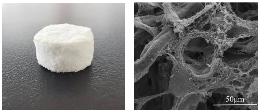
Fig. S11 The appearance and SEM image of disordered porous sponge
