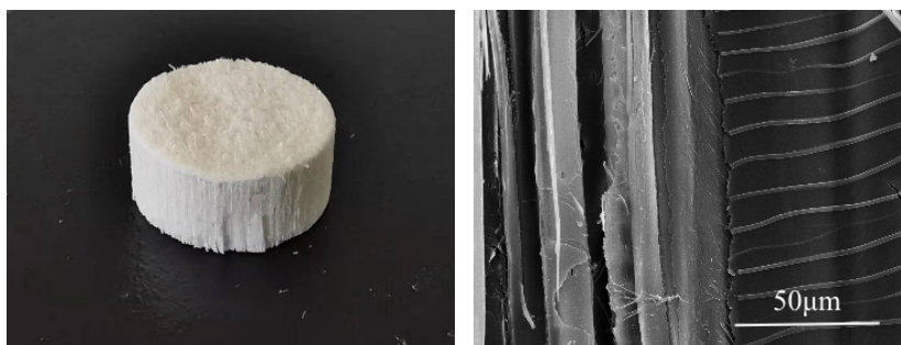
Fig. S10 The appearance and SEM image of natural basswood after delignification
