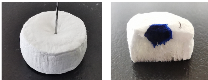
Fig. S12 Methylene blue permeation in CE
