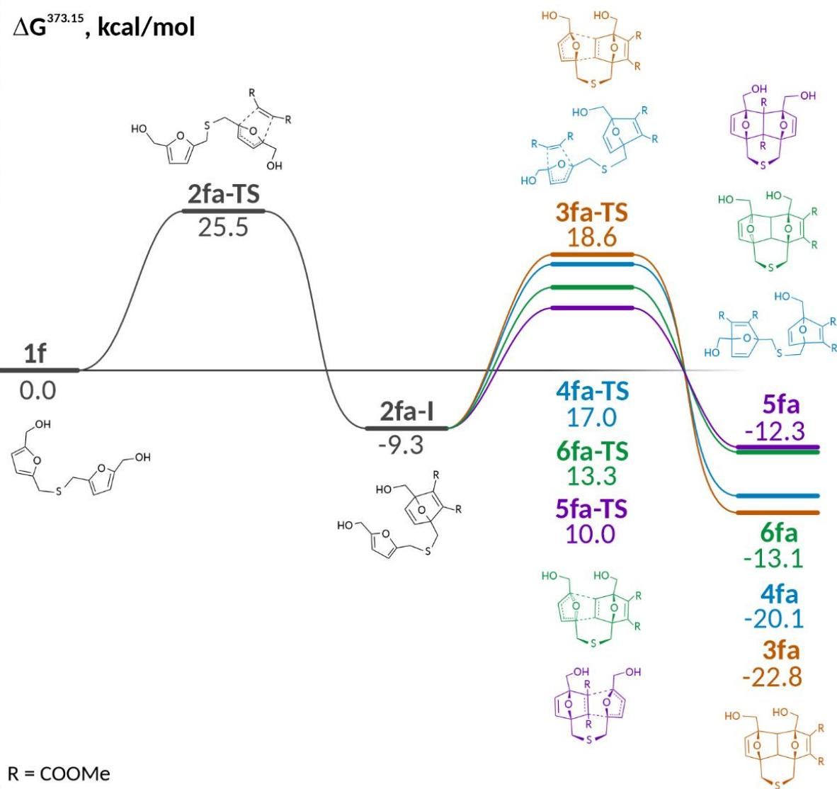
**Figure S116.** Gibbs free energy profile for the cycloaddition reaction involving substrate **1f**.
