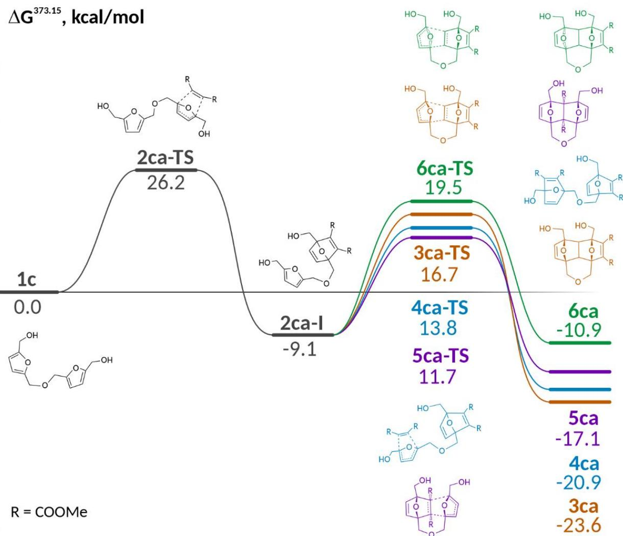
**Figure S113.** Gibbs free energy profile for the cycloaddition reaction involving substrate **1c**.
