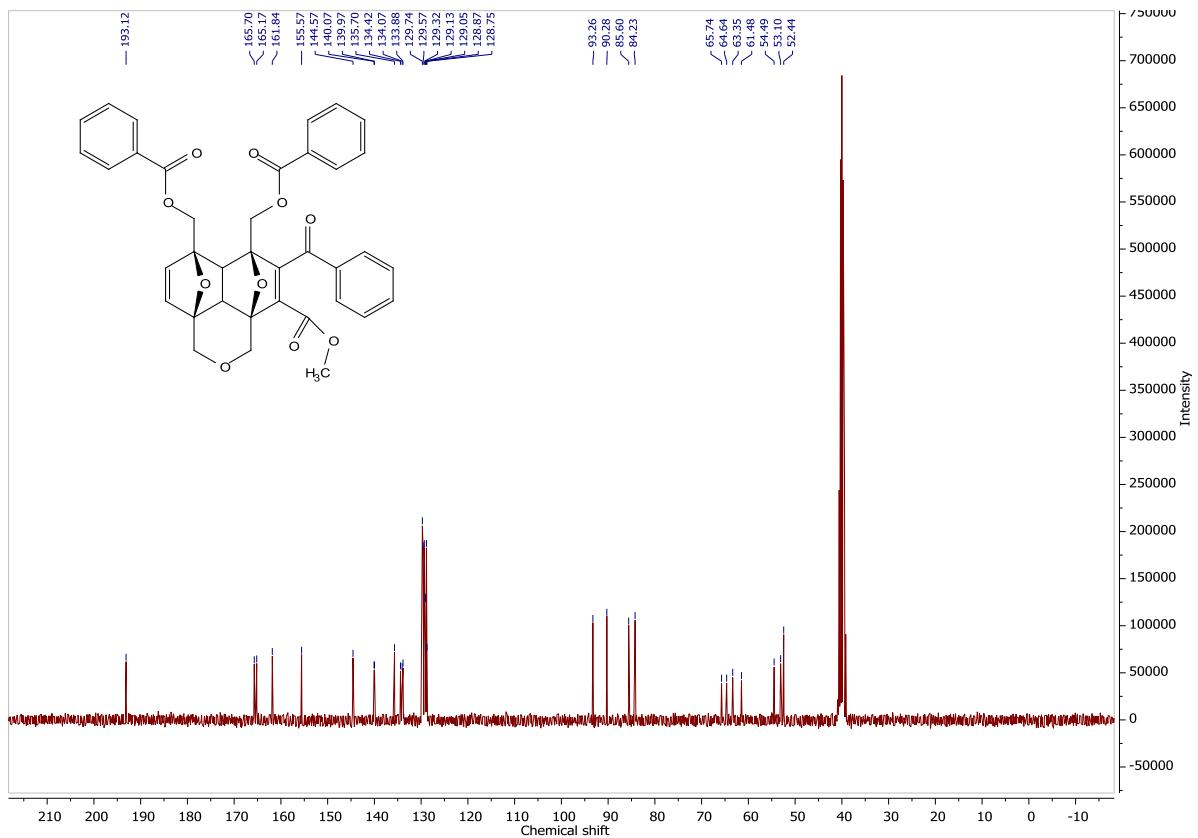
**Figure S54.**  $^{13}\text{C}$  NMR spectrum of (5-benzoyl-4-(methoxycarbonyl)-3a<sup>1</sup>,6a-dihydro-1H,3H,6H,7H-3a,6:7,9a-diepoxybenzo[de]isochromene-6,7-diyl)bis(methylene) dibenzoate **3agB** (75 MHz, DMSO- $\text{d}_6$ ).
