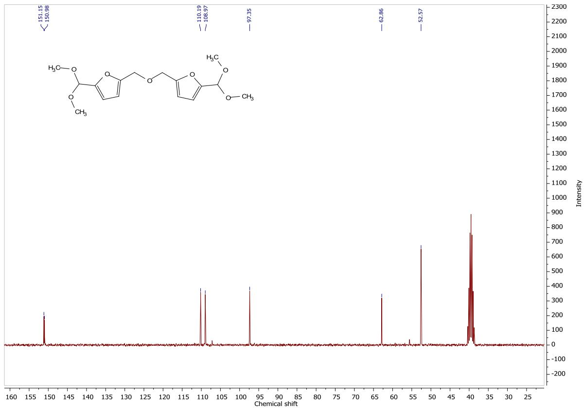
**Figure S10.**  $^{13}\text{C}$  NMR spectrum of 5,5'-(oxybis(methylene))bis(2-(dimethoxymethyl)furan), **1d** (75 MHz,  $\text{DMSO}-d_6$ ).
