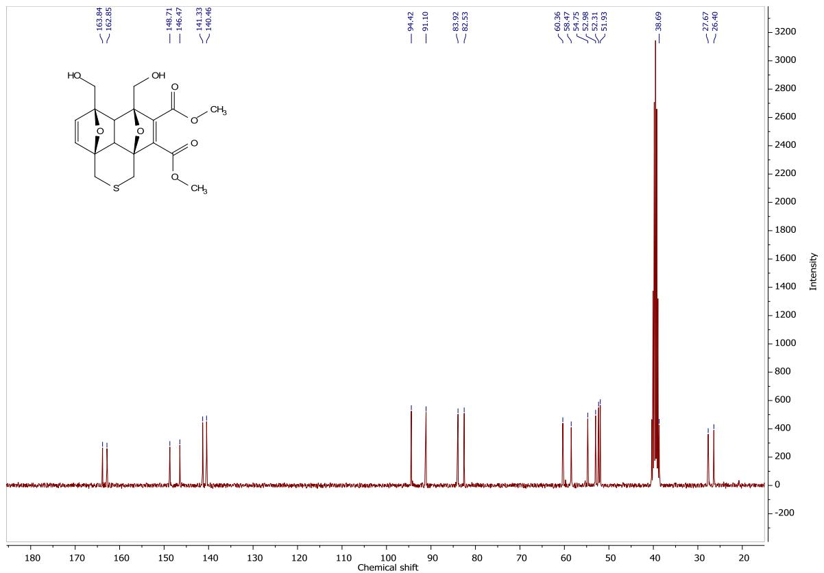
**Figure S64.**  $^{13}\text{C}$  NMR spectrum of dimethyl 6,7-bis(hydroxymethyl)-3a<sup>1</sup>,6a-dihydro-1H,3H,6H,7H-3a,6:7,9a-diepoxybenzo[de]isothiochromene-4,5-dicarboxylate **3fa** (75 MHz, DMSO-*d*<sub>6</sub>).
