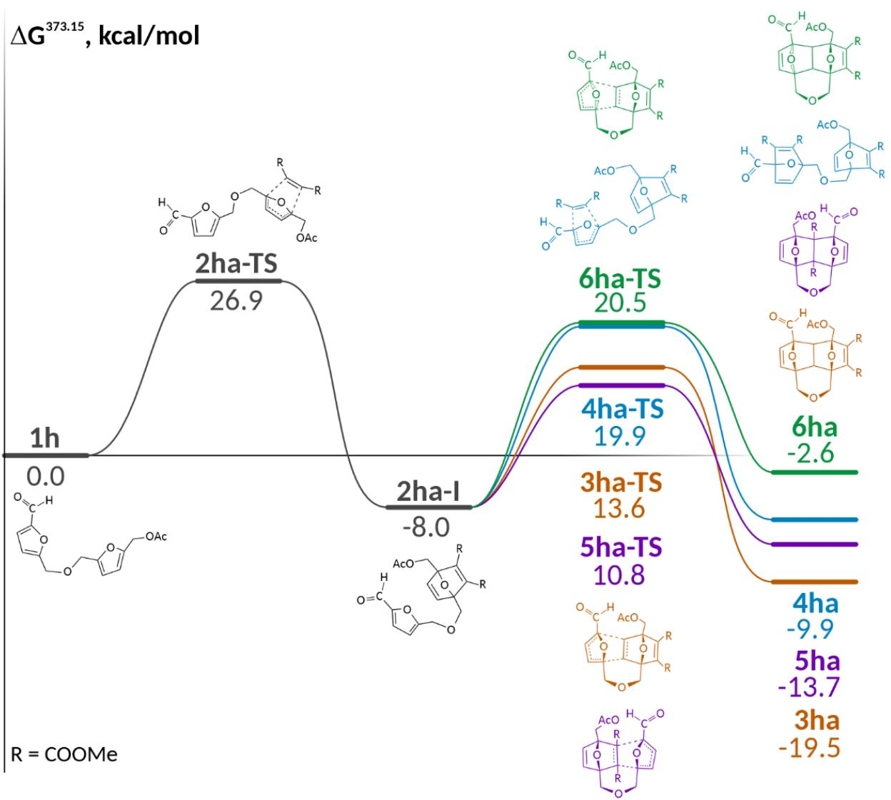
**Figure S118.** Gibbs free energy profile for the cycloaddition reaction involving substrate **1h**.
