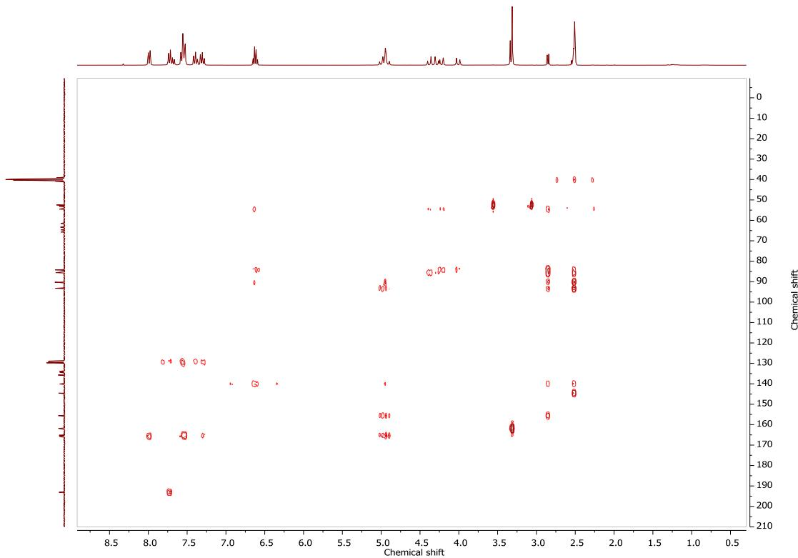
**Figure S56.**  $^1\text{H}$ - $^{13}\text{C}$  HMBC NMR spectrum of (5-benzoyl-4-(methoxycarbonyl)-3a<sup>1</sup>,6a-dihydro-1H,3H,6H,7H-3a,6:7,9a-diepoxybenzo[de]isochromene-6,7-diyl)bis(methylene) dibenzoate **3agB** (300 MHz, DMSO-d<sub>6</sub>).
