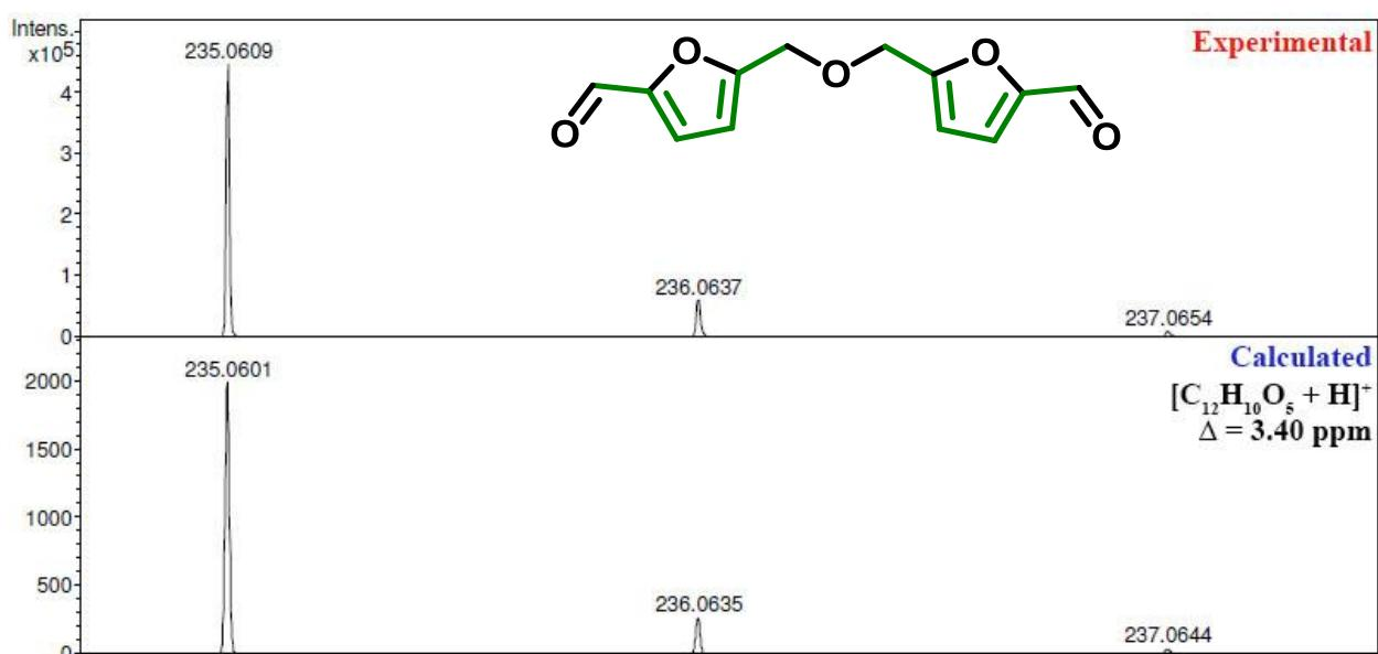
**Figure S75.** HRMS (ESI) spectrum of 5,5'-(oxybis(methylene))bis(furan-2-carbaldehyde) **1**.
