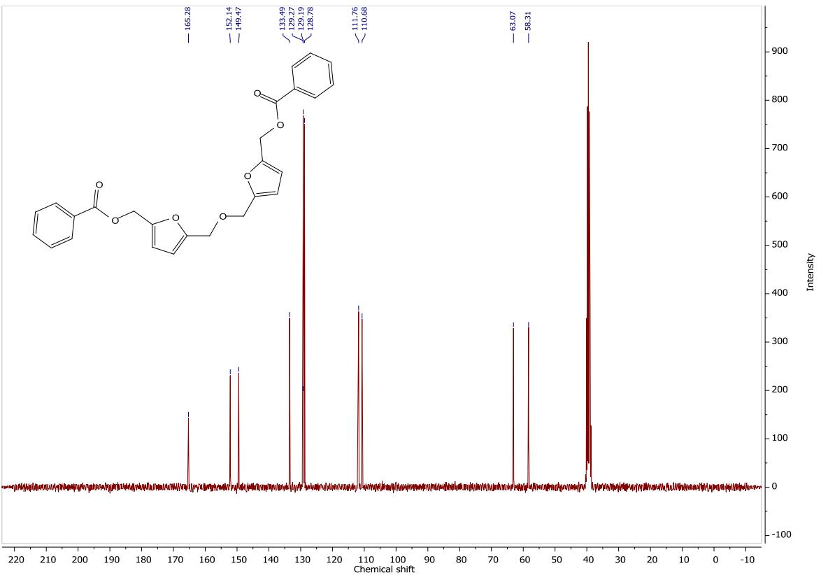
**Figure S4.** <sup>13</sup>C NMR spectrum of ((oxybis(methylene))bis(furan-5,2-diyl))bis(methylene) dibenzoate, **1a** (75 MHz, DMSO-*d*<sub>6</sub>).
