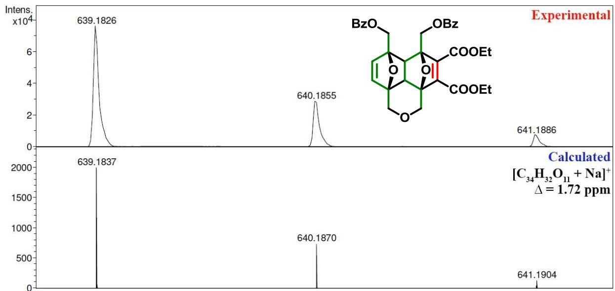
**Figure S88.** HRMS (ESI) spectrum of diethyl 6,7-bis((benzoyloxy)methyl)-3a<sup>1</sup>,6a-dihydro-1H,3H,6H,7H-3a,6:7,9a-diepoxybenzo[de]isochromene-4,5-dicarboxylate **3ad**.
