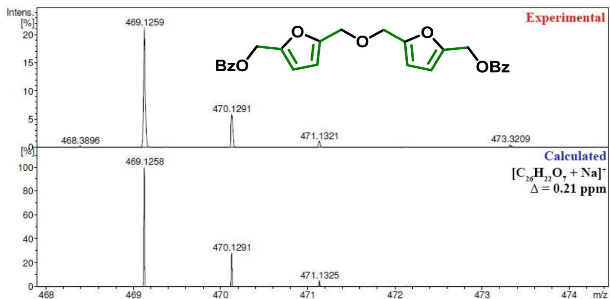
**Figure S76.** HRMS (ESI) spectrum of ((oxybis(methylene))bis(furan-5,2-diyl))bis(methylene) dibenzoate **1a**.
