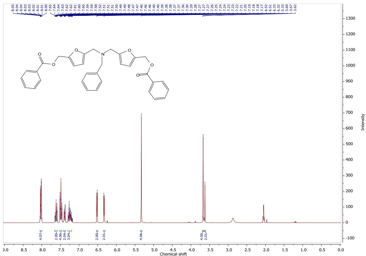
**Figure S11.**  $^1\text{H}$  NMR spectrum of (((benzylazanediyl)bis(methylene))bis(furan-5,2-diyl))bis(methylene) dibenzoate, **1e** (300 MHz, Acetone- $d_6$ ).
