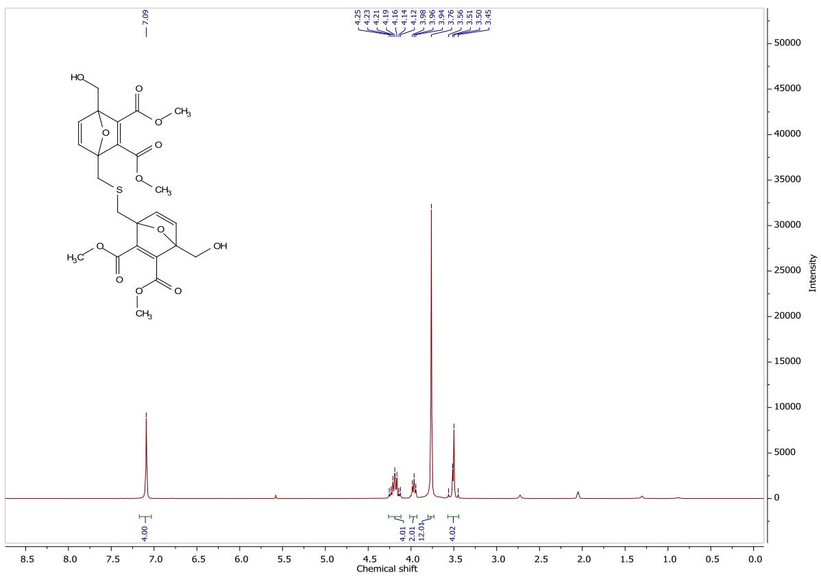
**Figure S27.**  $^1\text{H}$  NMR spectrum of 4,4'-(thiobis(methylene))bis(1-(hydroxymethyl)-7-oxabicyclo[2.2.1]hepta-2,5-diene-2,3-dicarboxylate) **4fa** (300 MHz, Acetone- $d_6$ ).
