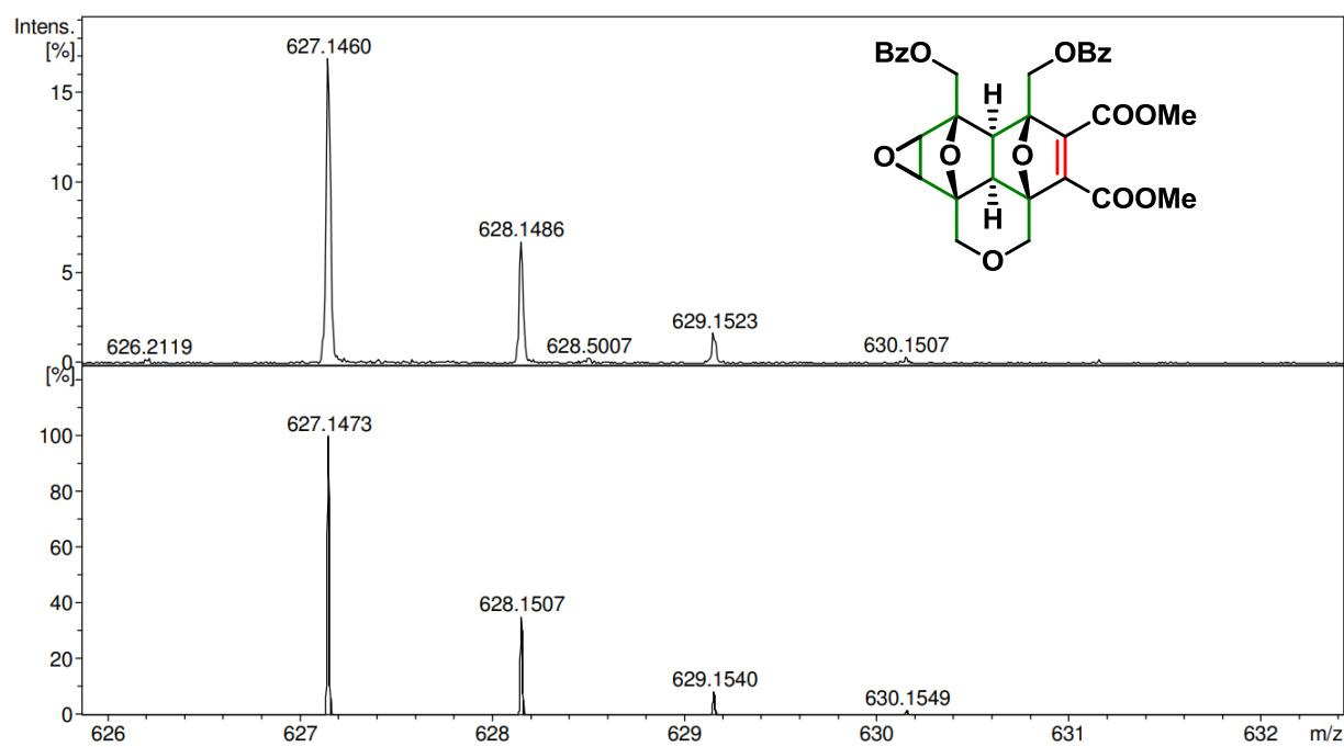
**Figure S105.** HRMS (ESI) spectrum of (3a*S*,3a*1S*,6*R*,6a*R*,7*R*,8*bS*)-dimethyl 6,7-bis((benzoyloxy)methyl)-1,3,3*a*1,6,6*a*,7,7*a*,8*a*-octahydro-3*a*,6:7,8*b*-diepoxybenzo[*d*]oxireno[2,3-*h*]isochromene-4,5-dicarboxylate **7aa**.
