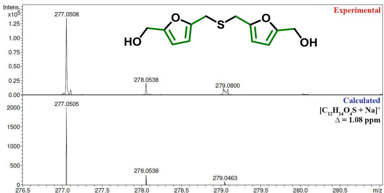
**Figure S81.** HRMS (ESI) spectrum of ((thiobis(methylene))bis(furan-5,2-diyl))dimethanol, **1f**.
