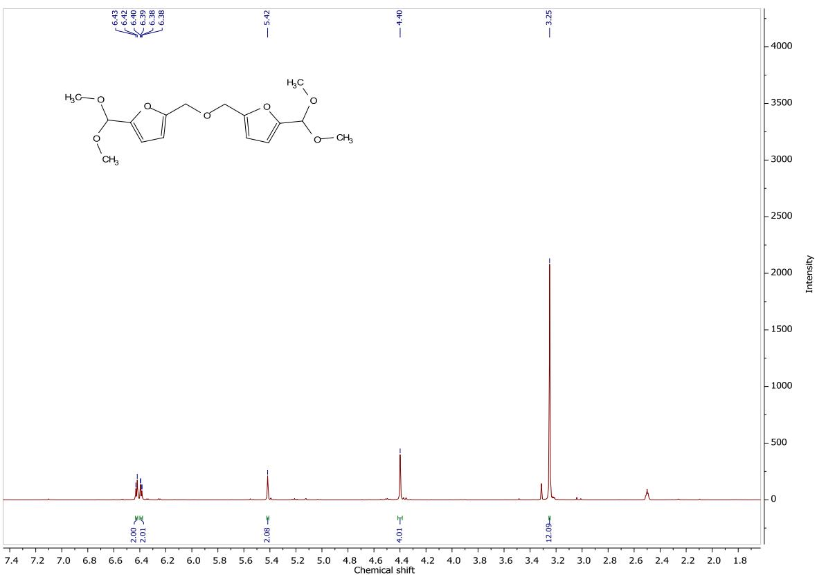
**Figure S9.**  $^1\text{H}$  NMR spectrum of 5,5'-(oxybis(methylene))bis(2-(dimethoxymethyl)furan), **1d** (300 MHz,  $\text{DMSO}-d_6$ ).
