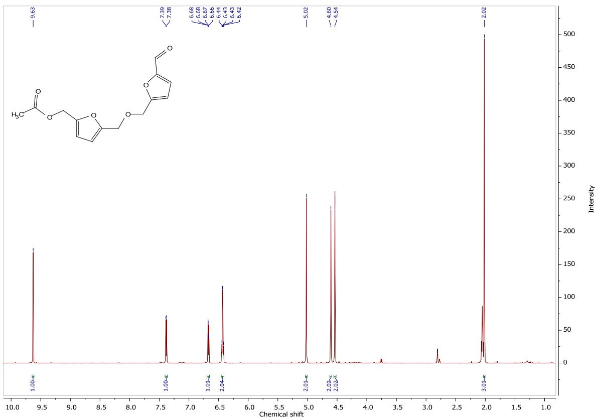
**Figure S17.**  $^1\text{H}$  NMR spectrum of (5-((5-formylfuran-2-yl)methoxy)methyl)furan-2-yl)methyl acetate, **1h** (300 MHz, Acetone- $d_6$ ).
