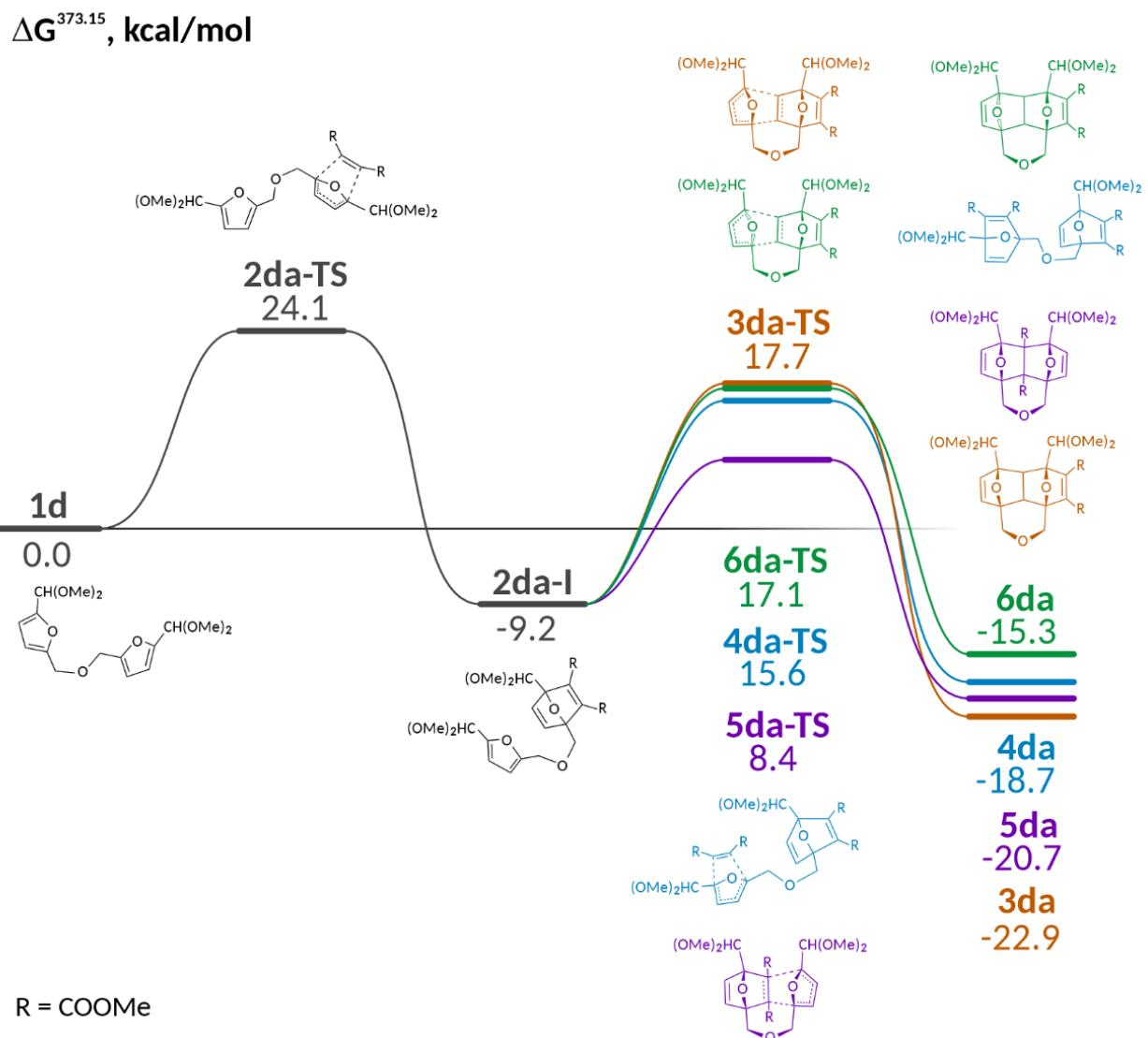
**Figure S114.** Gibbs free energy profile for the cycloaddition reaction involving substrate **1d**.
