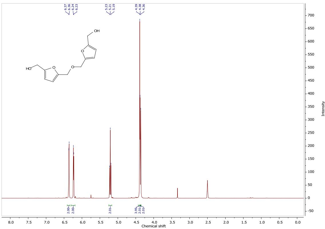
**Figure S7.**  $^1\text{H}$  NMR spectrum of ((oxybis(methylene))bis(furan-5,2-diyl))dimethanol, **1c** (300 MHz,  $\text{DMSO}-d_6$ ).
