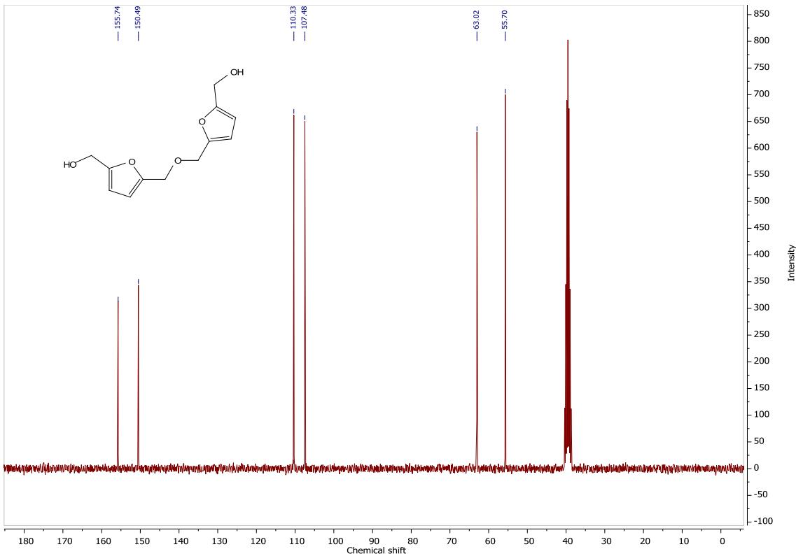
**Figure S8.**  $^{13}\text{C}$  NMR spectrum of ((oxybis(methylene))bis(furan-5,2-diyl))dimethanol, **1c** (75 MHz,  $\text{DMSO}-d_6$ ).
