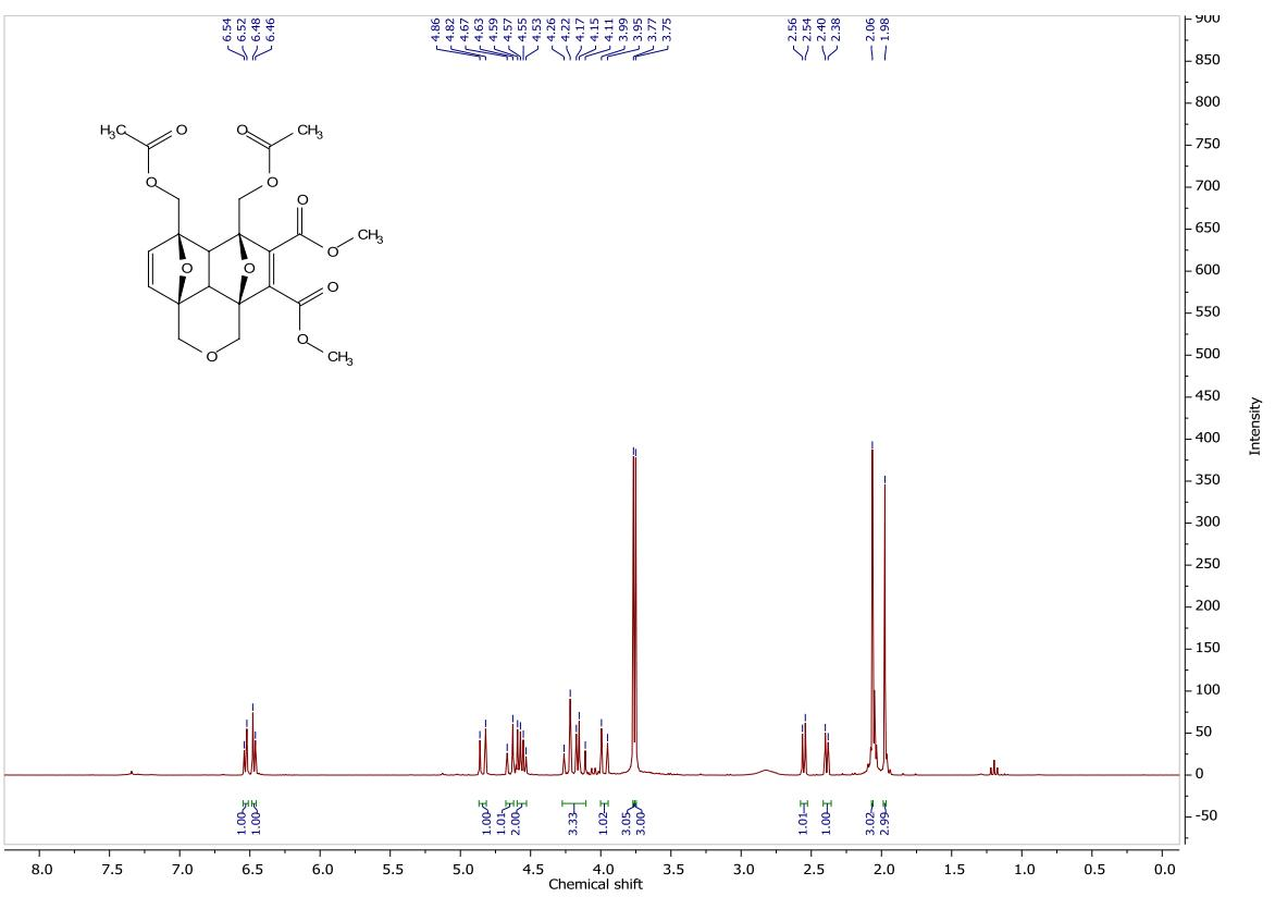
**Figure S57.** <sup>1</sup>H NMR spectrum of dimethyl 6,7-bis(acetoxymethyl)-3a<sup>1</sup>,6a-dihydro-1H,3H,6H,7H-3a,6:7,9a-diepoxybenzo[de]isochromene-4,5-dicarboxylate **3ba** (300 MHz, Acetone-d<sub>6</sub>).
