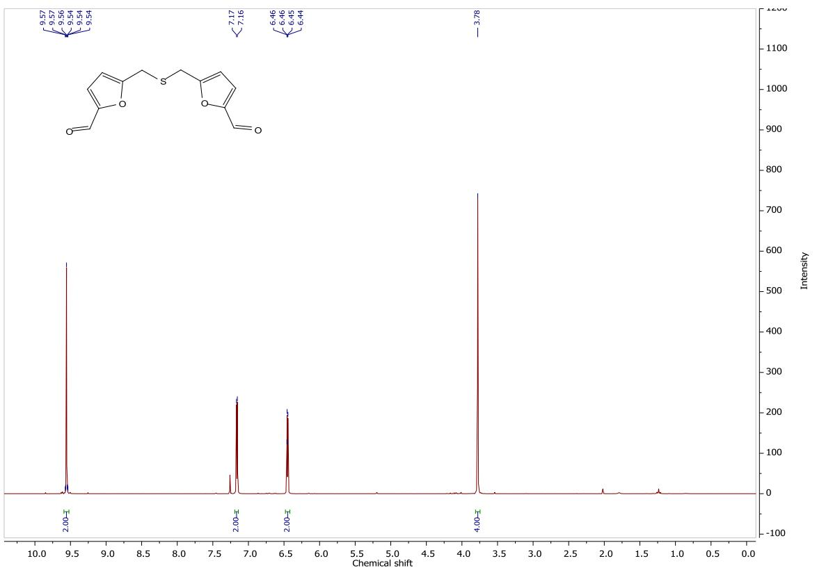
**Figure S19.** <sup>1</sup>H NMR spectrum of 5,5'-(thiobis(methylene))bis(furan-2-carbaldehyde) **1i** (300 MHz, Chloroform-*d*).
