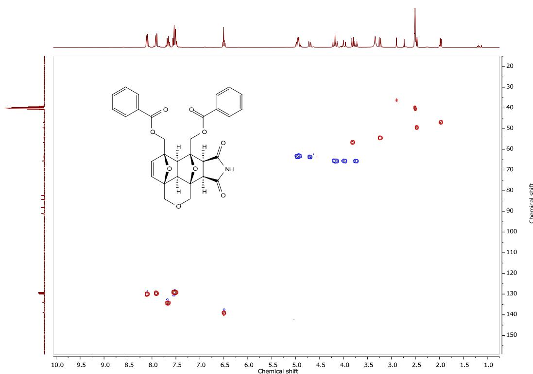
**Figure S31.**  $^1\text{H}$ - $^{13}\text{C}$  HSQC NMR spectrum of exo-(8,10-dioxo-3a<sup>1</sup>,6a,8,9,10,10a-hexahydro-1H,3H,6H-3a,6:7,10b-diepoxyisochromeno[4,5-ef]isoindole-6,7(7aH)-diyl)bis(methylene) dibenzoate **3ab** (300 MHz, DMSO-*d*<sub>6</sub>).
