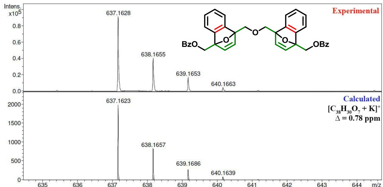
**Figure S102.** HRMS (ESI) spectrum of ((oxybis(methylene))bis(1,4-epoxynaphthalene-4,1(4H)-diyl))bis(methylene) dibenzoate **4ac**
