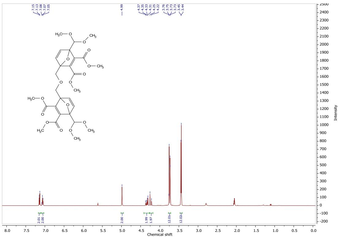
**Figure S25.** <sup>1</sup>H NMR spectrum of 4,4'-(oxybis(methylene))bis(1-(dimethoxymethyl)-7-oxabicyclo[2.2.1]hepta-2,5-diene-2,3-dicarboxylate) **4da** (300 MHz, Acetone-*d*<sub>6</sub>).
