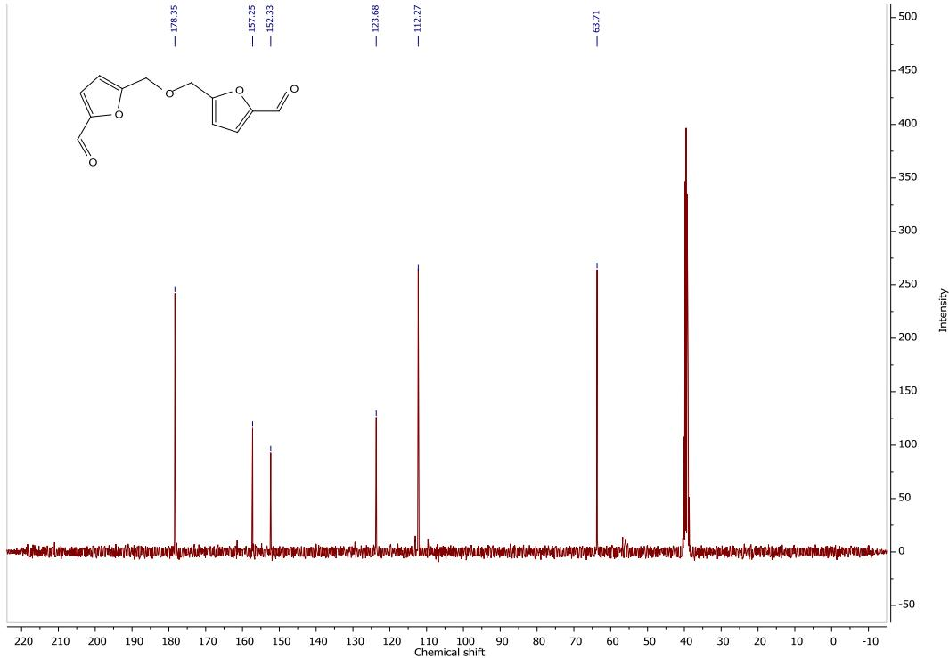
**Figure S2.**  $^{13}\text{C}$  NMR spectrum of 5,5'-(oxybis(methylene))bis(furan-2-carbaldehyde), **1** (75 MHz,  $\text{DMSO}-d_6$ ).
