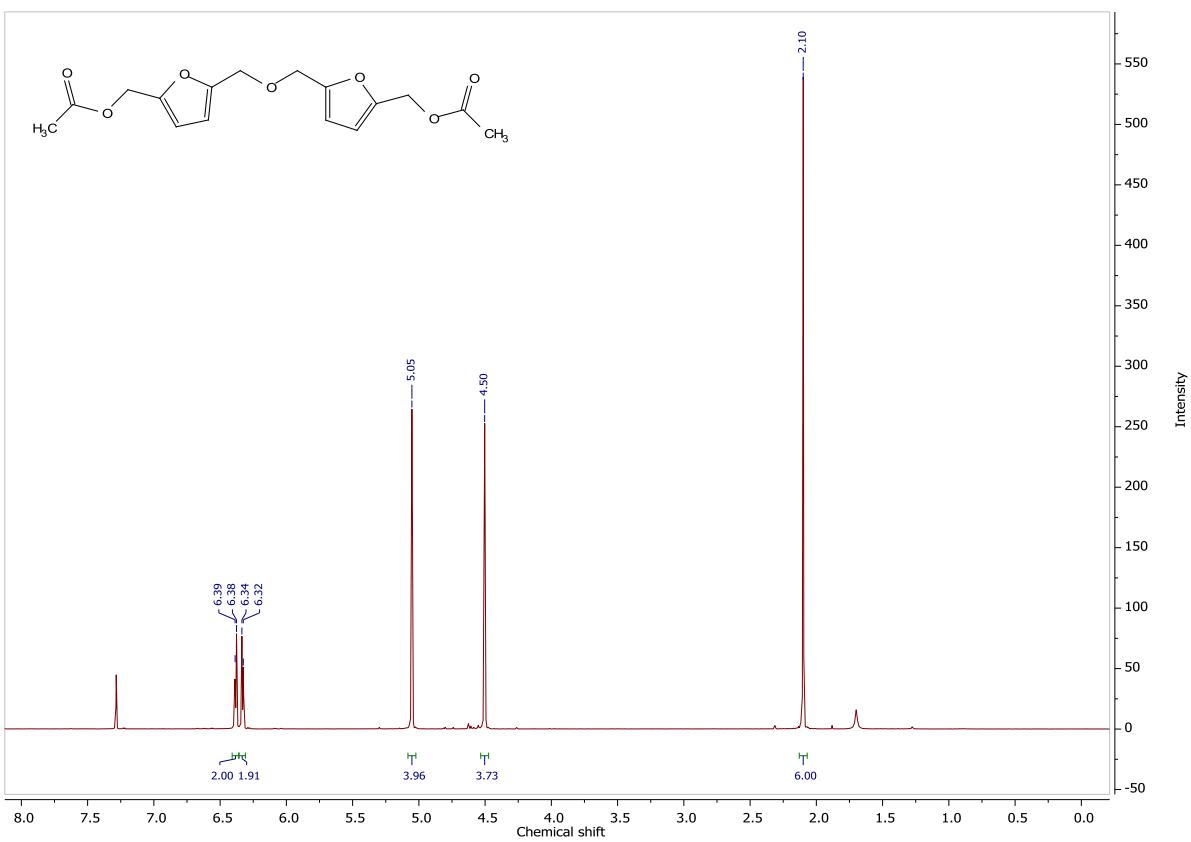
**Figure S5.**  $^1\text{H}$  NMR spectrum of ((oxybis(methylene))bis(furan-5,2-diyl))bis(methylene) diacetate, **1b** (300 MHz, chloroform-*d*).
