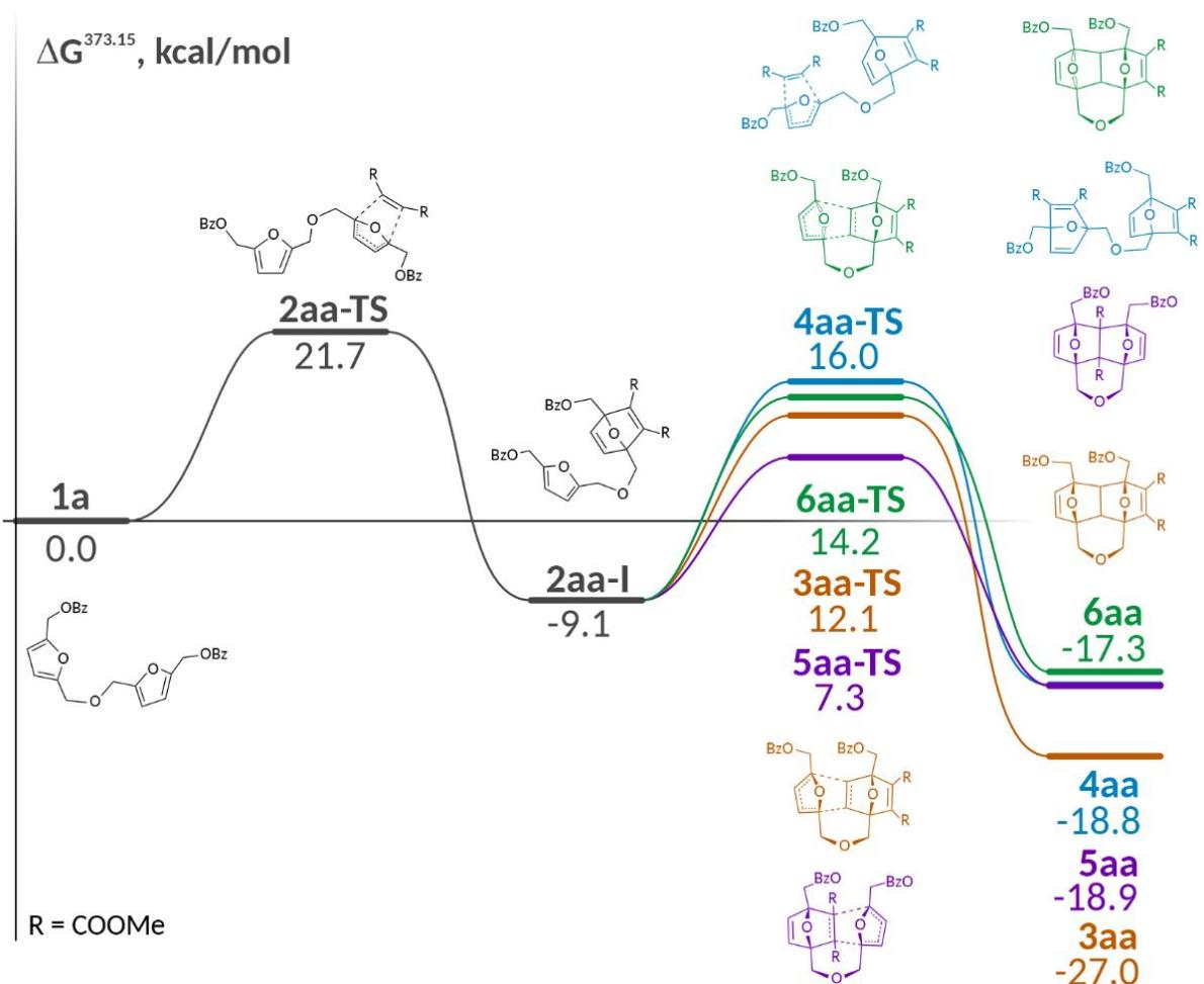
**Figure S111.** Gibbs free energy profile for the cycloaddition reaction involving substrate **1a**.
