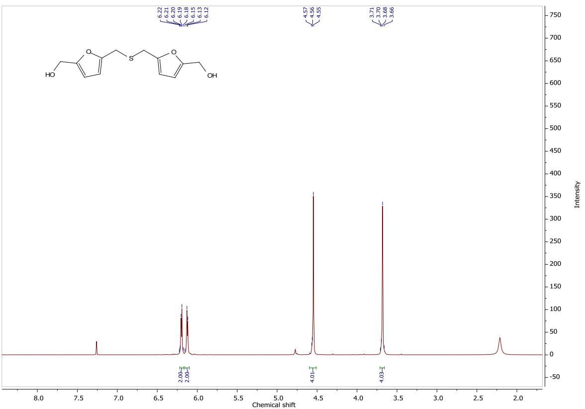
**Figure S13.**  $^1\text{H}$  NMR spectrum of ((thiobis(methylene))bis(furan-5,2-diyl))dimethanol, **1f** (300 MHz, Chloroform-*d*).
