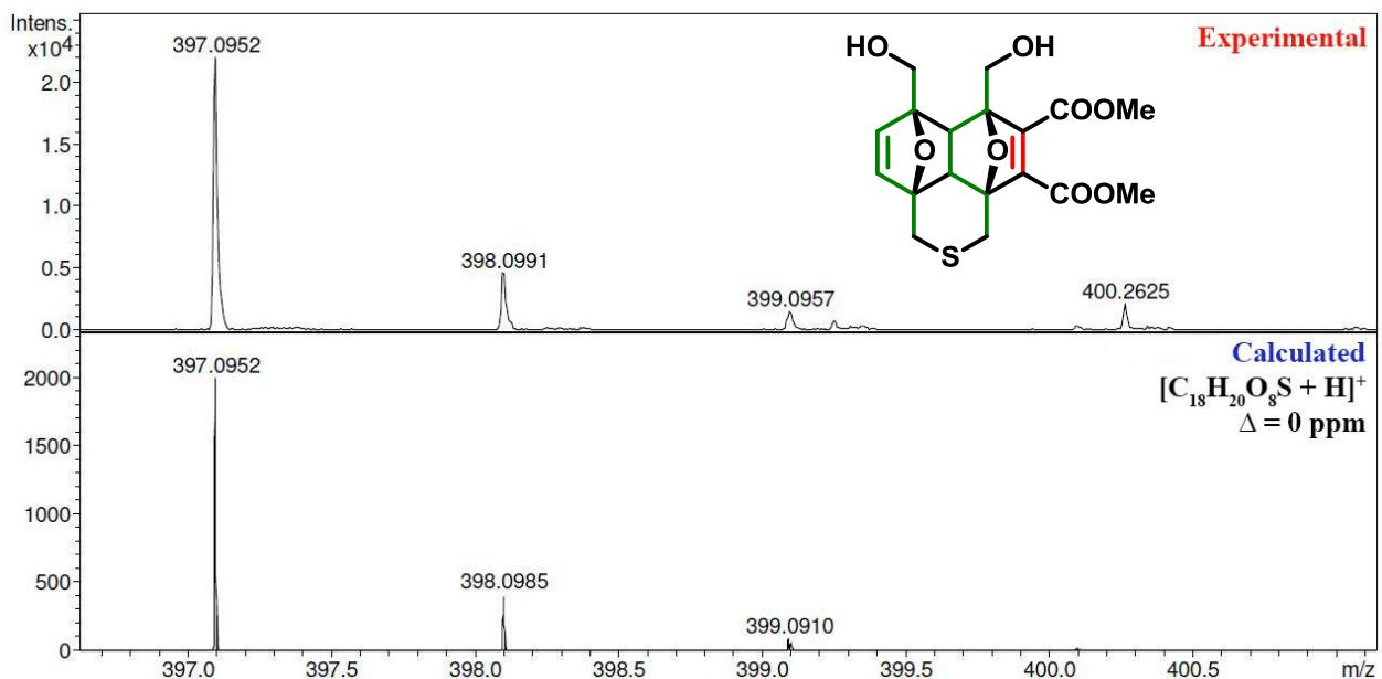
**Figure S98.** HRMS (ESI) spectrum of dimethyl 6,7-bis(hydroxymethyl)-3a<sup>1</sup>,6a-dihydro-1H,3H,6H,7H-3a,6:7,9a-diepoxybenzo[de]isothiocromene-4,5-dicarboxylate **3fa**.
