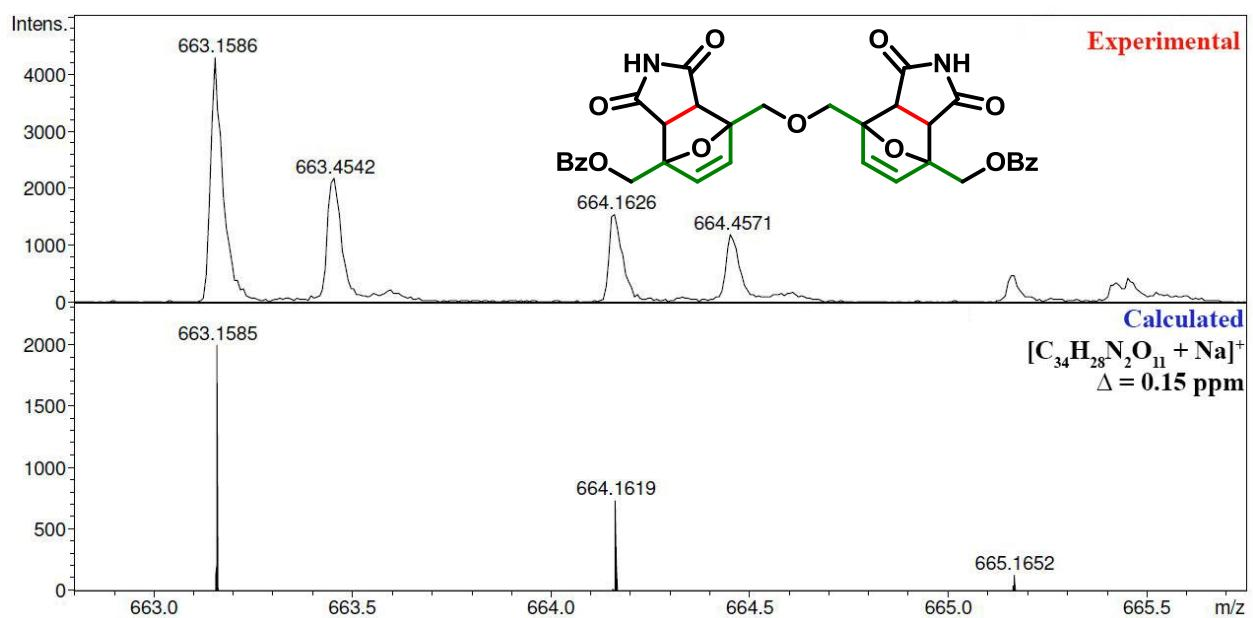
**Figure S101.** HRMS (ESI) spectrum of ((oxybis(methylene))bis(1,3-dioxo-1,2,3,3a,7,7a-hexahydro-4H-4,7-epoxyisoindole-7,4-diyl))bis(methylene) dibenzoate **4ab**.
