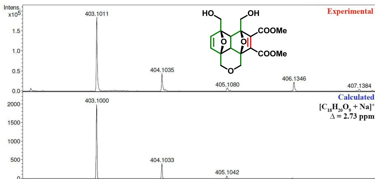
**Figure S95.** HRMS (ESI) spectrum of dimethyl 6,7-bis(hydroxymethyl)-3a1,6a-dihydro-1H,3H,6H,7H-3a,6:7,9a-diepoxybenzo[de]isochromene-4,5-dicarboxylate **3ca**
