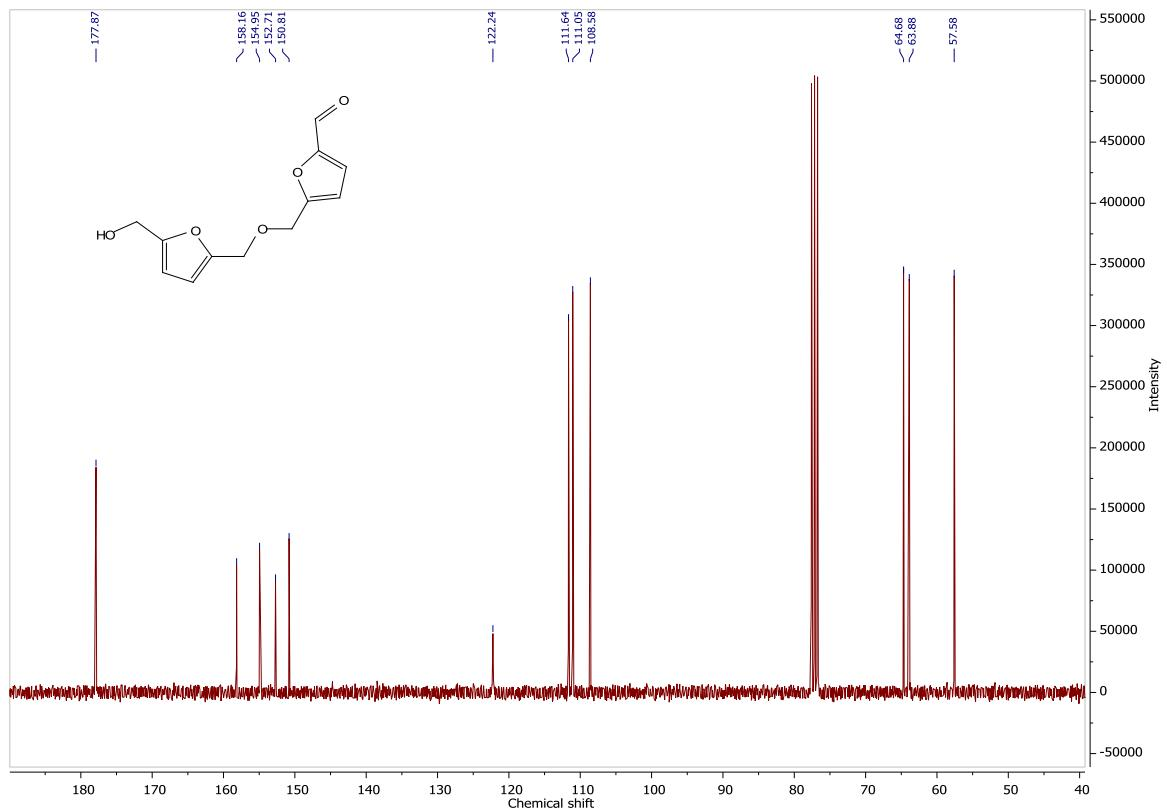
**Figure S16.** <sup>13</sup>C NMR spectrum of 5-((5-(hydroxymethyl)furan-2-yl)methoxy)methyl)furan-2-carbaldehyde, **1g** (75 MHz, Chloroform-*d*).
