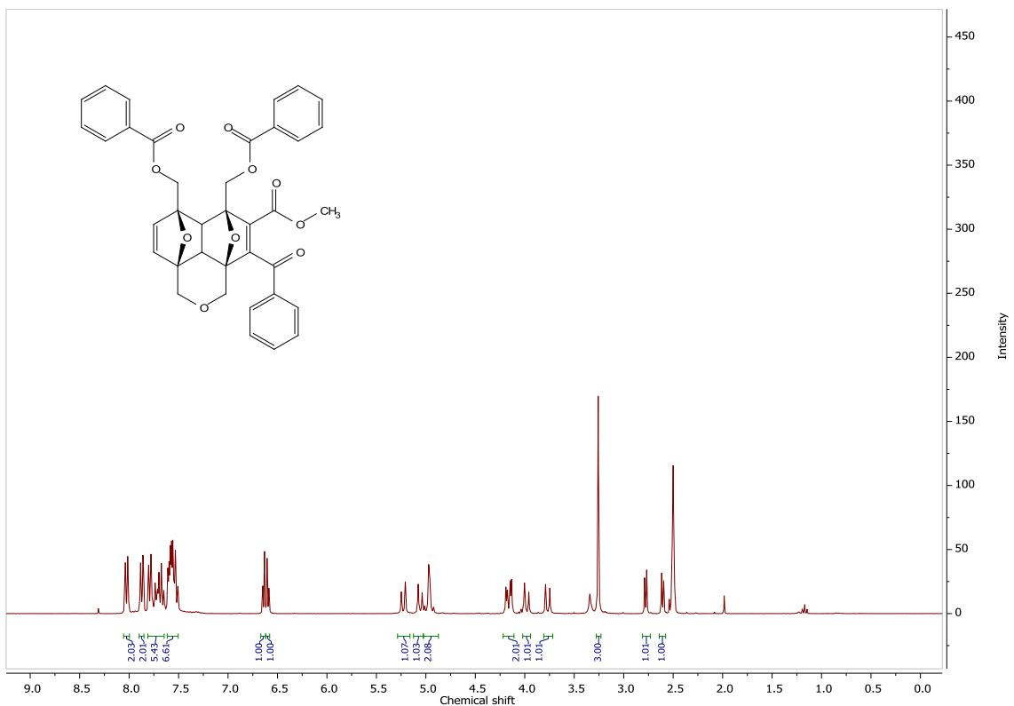
**Figure S49.** <sup>1</sup>H NMR spectrum of (4-benzoyl-5-(methoxycarbonyl)-3a<sup>1</sup>,6a-dihydro-1H,3H,6H,7H-3a,6:7,9a-diepoxybenzo[de]isochromene-6,7-diyl)bis(methylene) dibenzoate **3agA** (300 MHz, DMSO- $d_6$ ).
