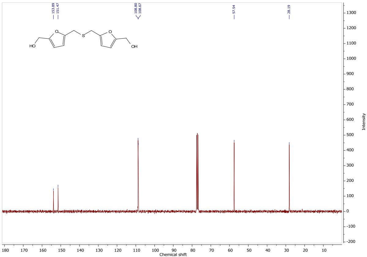
**Figure S14.**  $^{13}\text{C}$  NMR spectrum of ((thiobis(methylene))bis(furan-5,2-diyl))dimethanol, **1f** (75 MHz, Chloroform-*d*).
