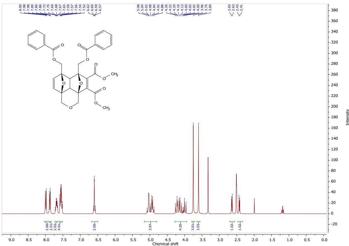
**Figure S35.**  $^1\text{H}$  NMR spectrum of Dimethyl 6,7-bis((benzoyloxy)methyl)-3a<sup>1</sup>,6a-dihydro-1H,3H,6H,7H-3a,6:7,9a-diepoxybenzo[de]isochromene-4,5-dicarboxylate **3aa** (300 MHz, DMSO-*d*<sub>6</sub>).
