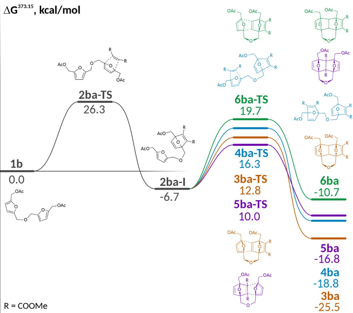
**Figure S112.** Gibbs free energy profile for the cycloaddition reaction involving substrate **1b**.
