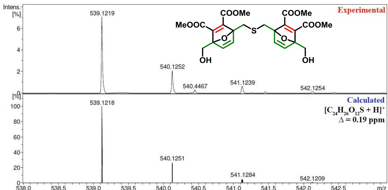
**Figure S104.** HRMS (ESI) spectrum of 4,4'-(thiobis(methylene))bis(1-(hydroxymethyl)-7-oxabicyclo[2.2.1]hepta-2,5-diene-2,3-dicarboxylate) **4fa**.
