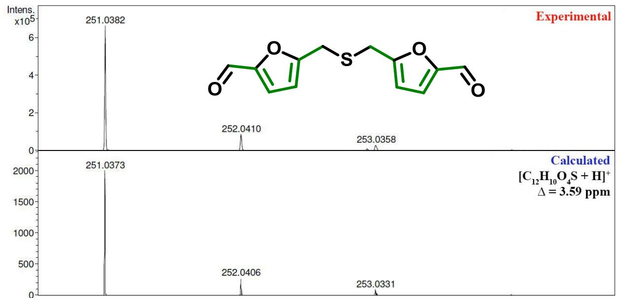
**Figure S84.** HRMS (ESI) spectrum of 5,5'-(thiobis(methylene))bis(furan-2-carbaldehyde) **1i**.
