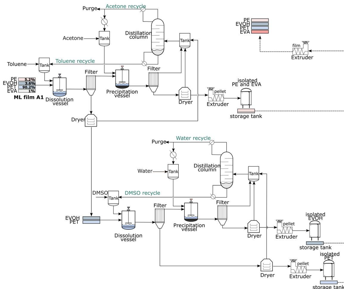
**Figure SI 1:** Process flow diagram to recycle multilayer film A1 composed of polymer resins PE, EVOH, PET, and EVA through STRAP-A, including inputs to the process (orange) and the solvent recycle streams (green). Each polymer component is recovered in the pellet form, which is then sent to the film extruder to produce recycled multilayer film A1 (grey box).
