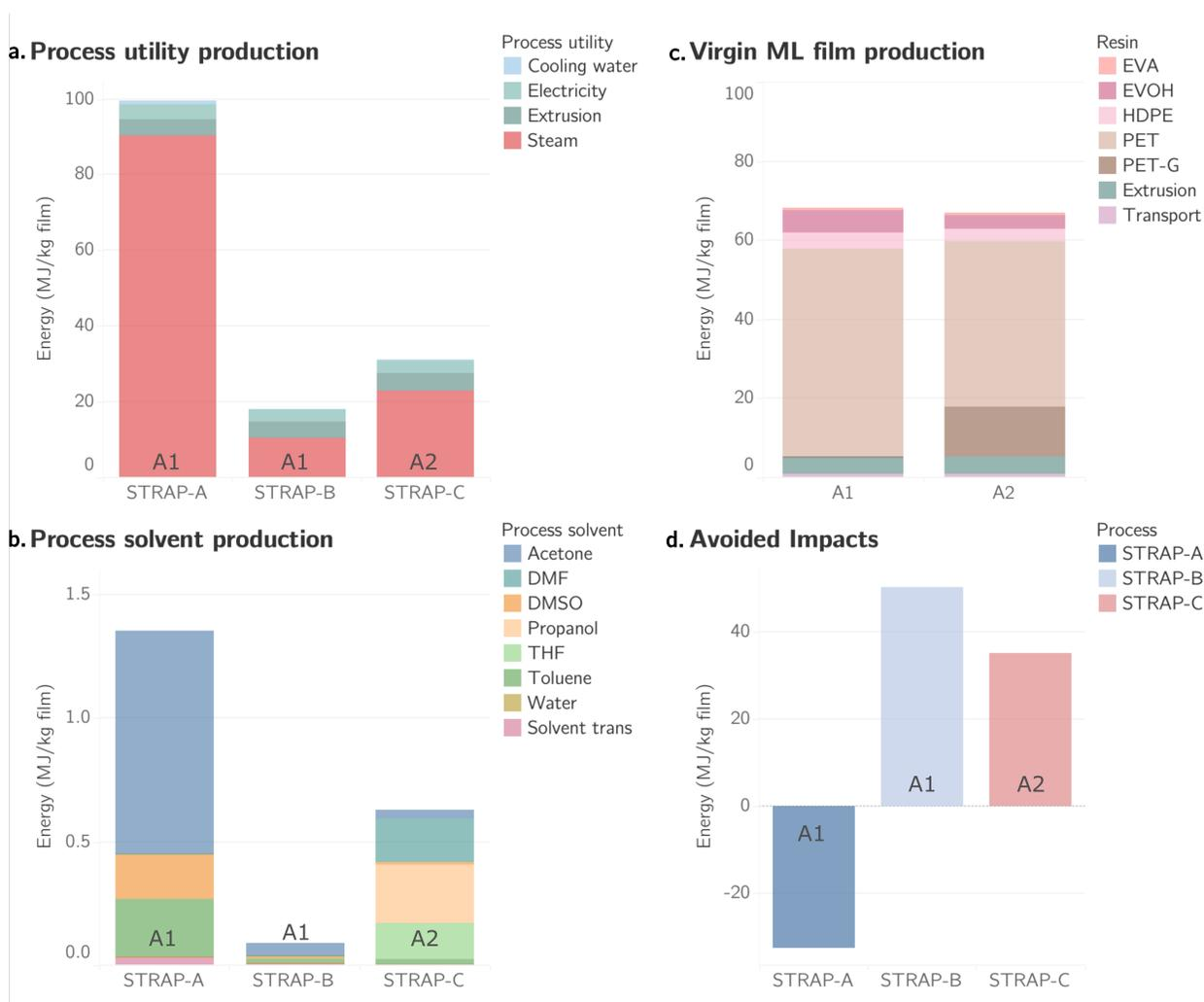
**Figure SI 6:** Energy use (MJ) of STRAP process in terms of utility and raw materials for the production of 1 kg of film A1 (STRAP-A and STRAP-B) and 1 kg of film A2 (STRAP-C), their constituent virgin polymer production and avoided impacts via STRAP recovery technology.
