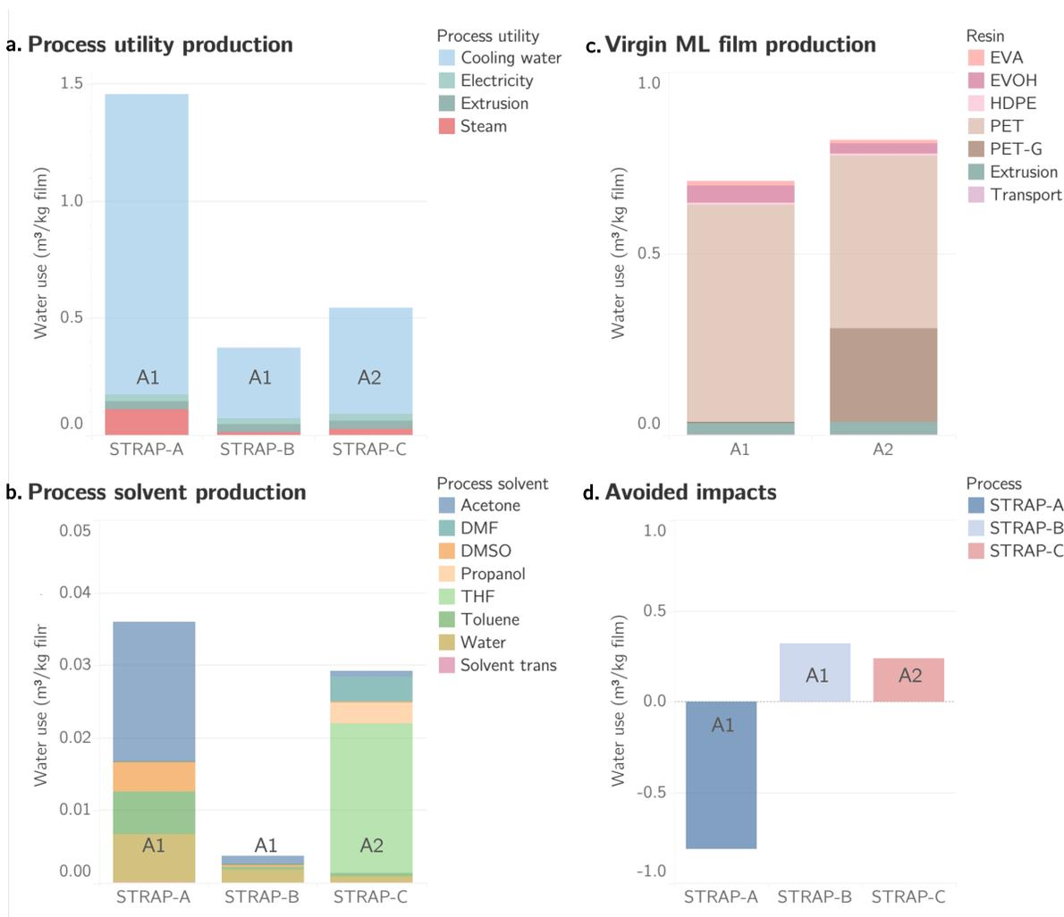
**Figure SI 8:** Water usage factor (m<sup>3</sup>) of STRAP process in terms of utility and raw materials for the production of 1 kg of film A1 (STRAP-A and STRAP-B) and 1 kg of film A2 (STRAP-C), their constituent virgin polymer production and avoided impacts via STRAP recovery technology.
