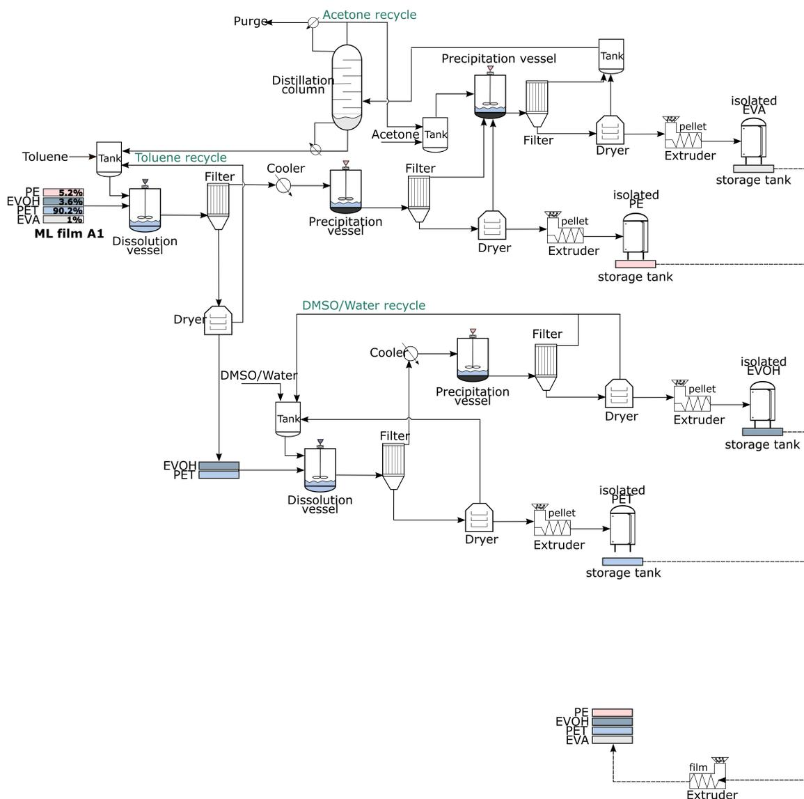
**Figure SI 2:** Process flow diagram to recycle multilayer film A1 composed of polymer resins PE, EVOH, PET, and EVA through STRAP-B, including inputs to the process (orange) and the solvent recycle streams (green). Each polymer component is recovered in the pellet form, which is then sent to the film extruder to produce recycled multilayer film A1 (grey box).
