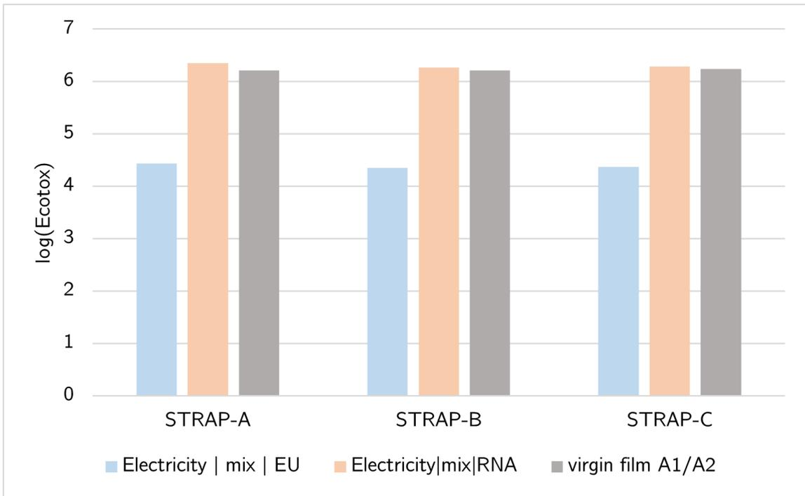
**Figure SI 5:** Ecotoxicity values for the electricity usage in STRAP processes based on EU and RNA regions compared to the virgin film production: film A1 (STRAP-A and STRAP-B) and film A2 (STRAP-C) | Region: EU.
