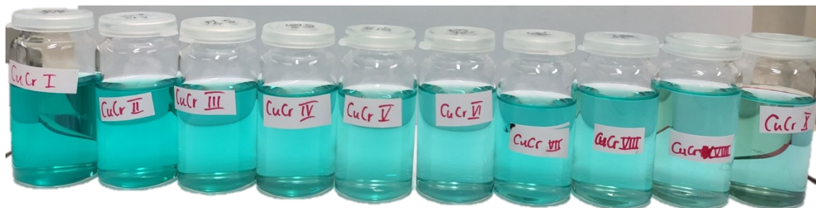
Figure S5: Filtrates of CuO/Cr 2 O 3 -B experiment. The blue colour is typical for copper formate species.
