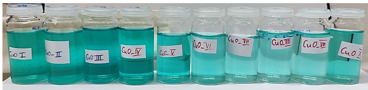
Figure S4: Filtrates of CuO/ZnO-B experiment. The blue colour is typical for copper formate species.
