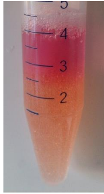
Figure S7. Photograph of resin AmberLite® HPR 1100 when in contact with the IL and betalains rich phase of the ABS.
