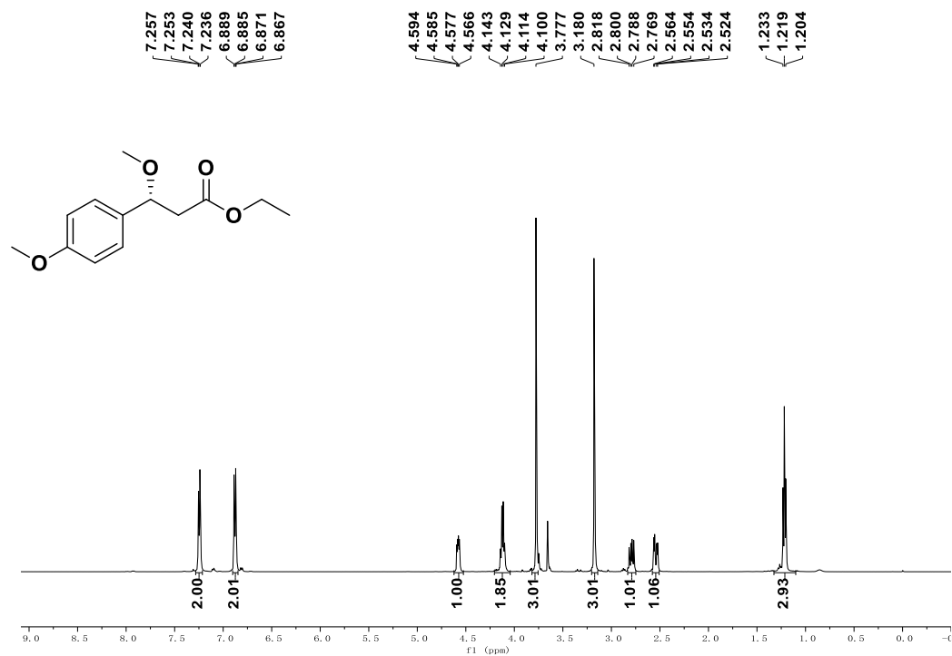
Figure S26. 1 H NMR spectrum of ethyl ( R )-3-methoxy-3-(4'-methoxyphenyl) propanoate ( 5j ) (500 MHz, CDCl 3 )
