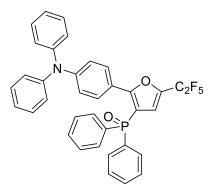
(2-(4-(Diphenylamino)phenyl)-5-(perfluoroethyl)furan-3-yl)diphenylphosphine oxide (12): Yield = 42% (79.3 mg, 0.3 mmol scale). White solid.
