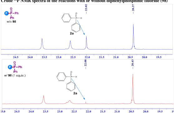
Crude <sup>31</sup>P NMR spectra of the reactions with or without diphenylphosphinic fluoride (98)
