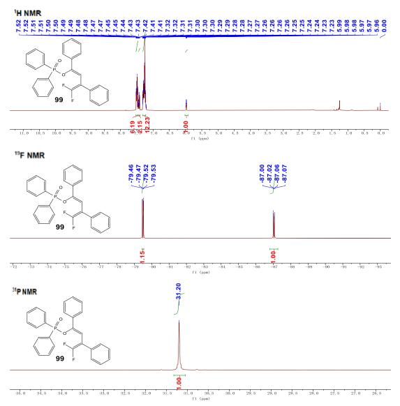
NMR spectra of (Z)-4,4-difluoro-1,3-diphenylbuta-1,3-dien-1-yl diphenylphosphinate (99)
